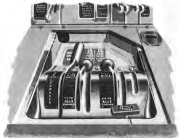
AUXILIARY TANK SELECTOR CONTROLS
