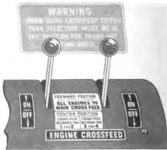
Crossfeed Valve Controls
