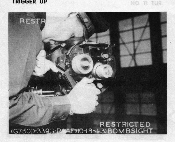
Hold trigger all the way up, do not apply too muc possible precission.
