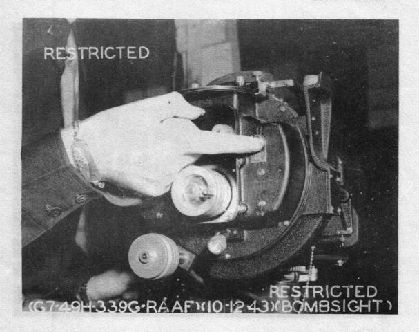
After trigger, reach over with right hand and turn on Telescope Switch.
