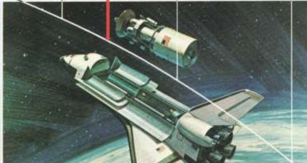
Shuttle-deployed interplanetary spacecraft is attached to an Interim Upper Stage, which will propel it across space to Jupiter.
