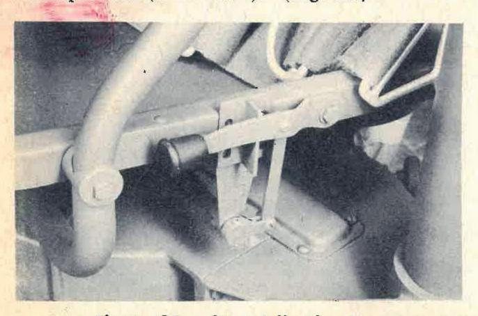
Figure 31 — Seat Adjusting Lever
