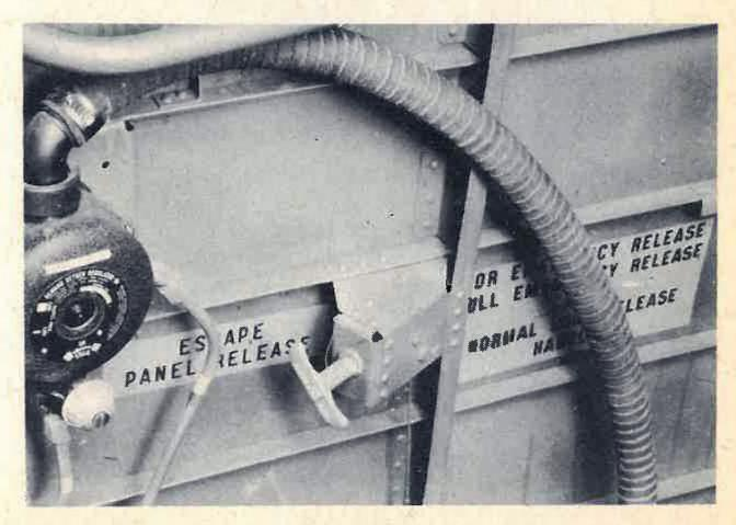
Figure 23 — Radio Operator's Emergency Release
