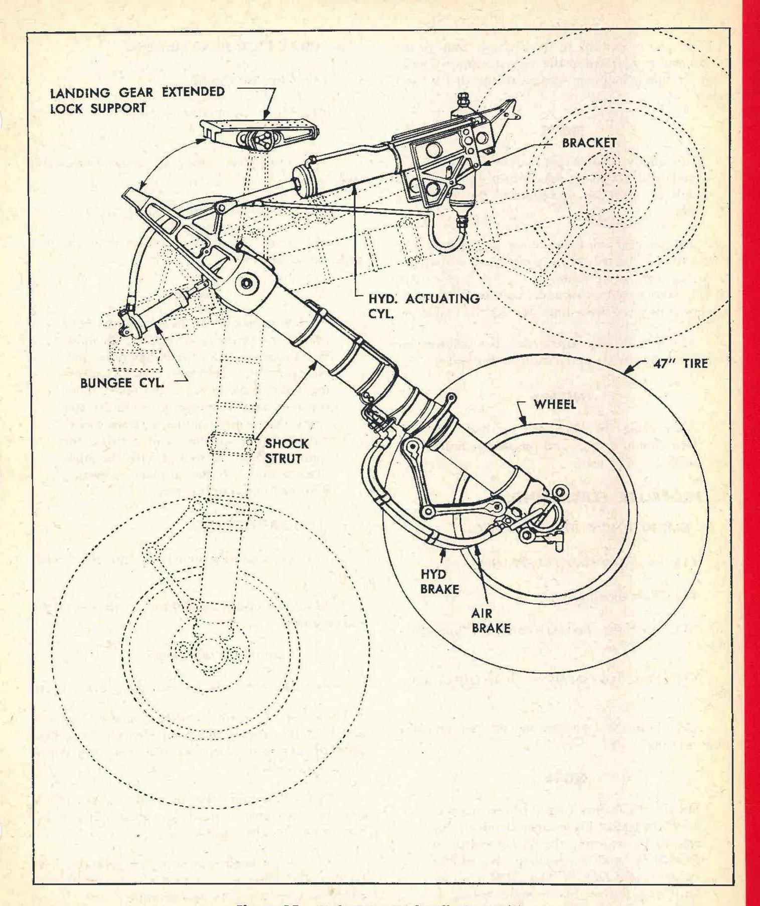
Figure 25 — Main Gear Hydraulic Operation
