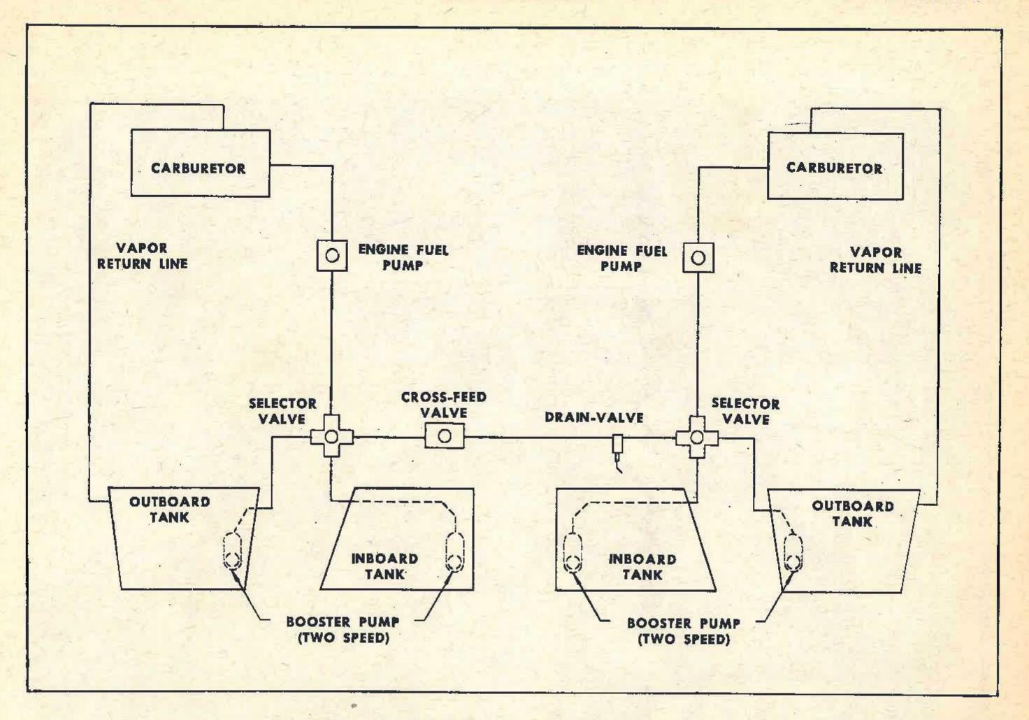
Figure 2 - Simplified Fuel System Diagram
