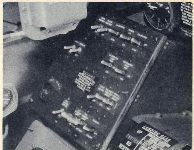
Figure 16 - Pilat's Electrical Switch Panel
