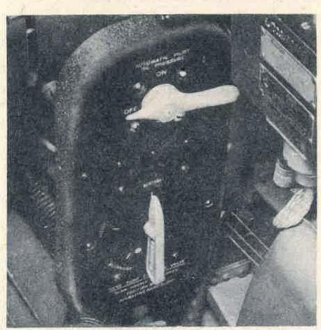
Figure 24 — Hydraulic Hand Pump Selector Valve
