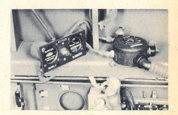
Figure 34 - Oxygen Control Unit
