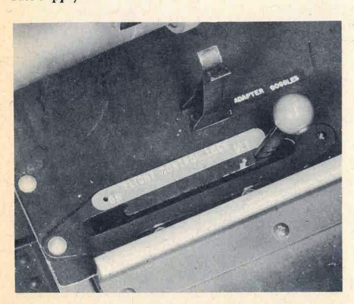
Figure 12.—Flight Control Lock
