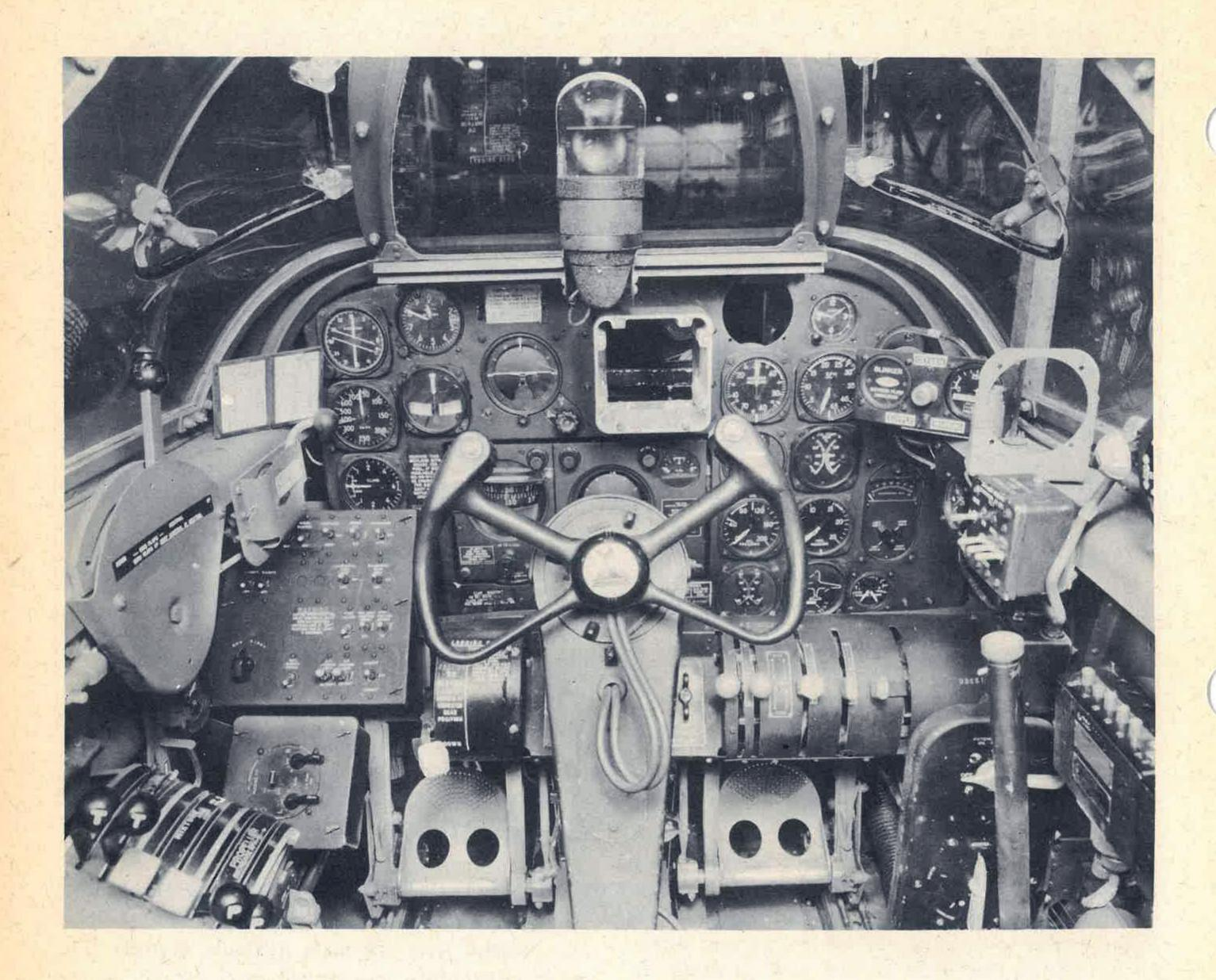
Figure 3 - Pilot's Instrument Panel
