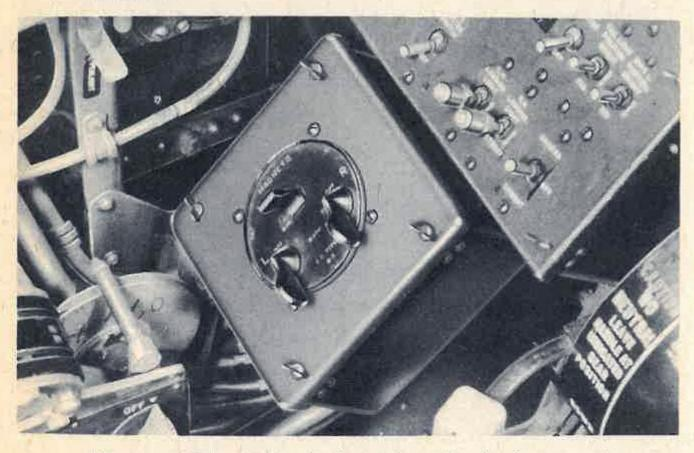
Figure 17 —Pilot's Ignition Switch Panel
