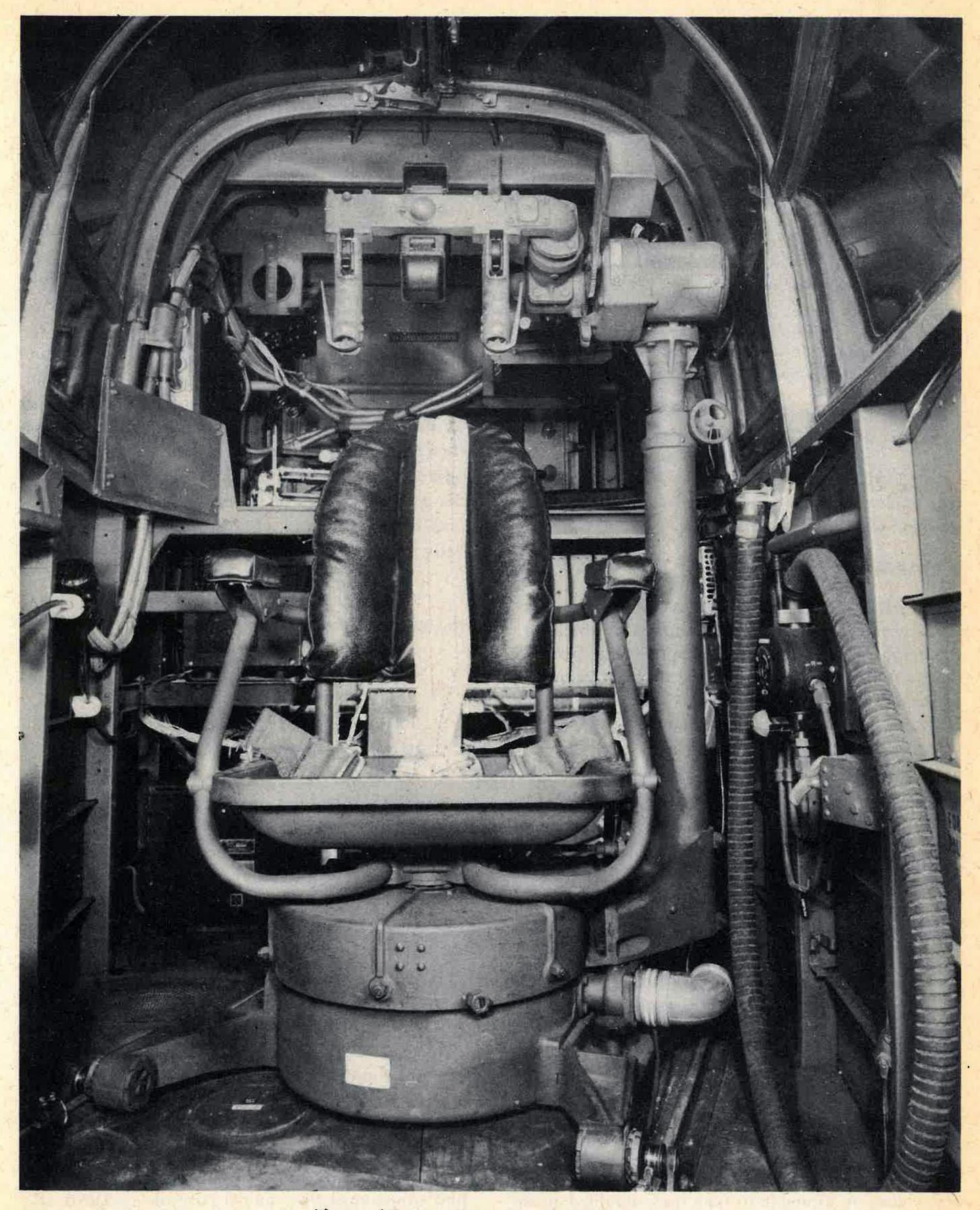
Figure 27 — Radio Operator's Controls
