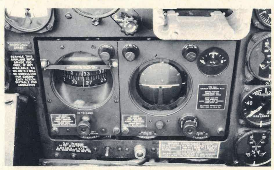
Figure 21 — Auto Pilot Instruments
