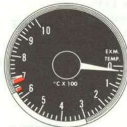
TURBINE INLET TEMPERATURE (T 5 )
