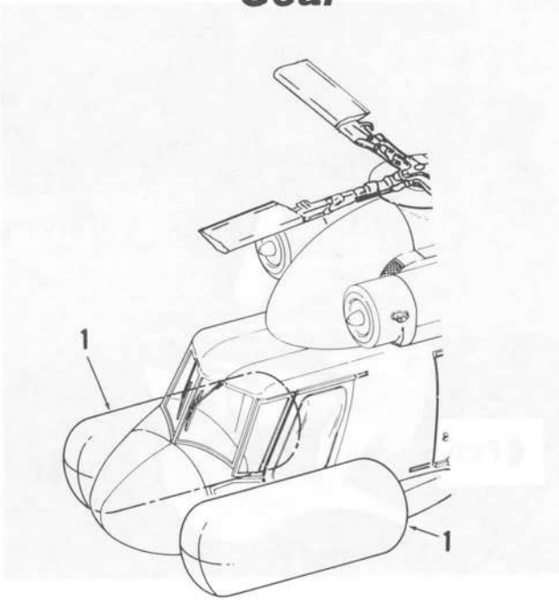
1. EMERGENCY FLOATATION GEAR
