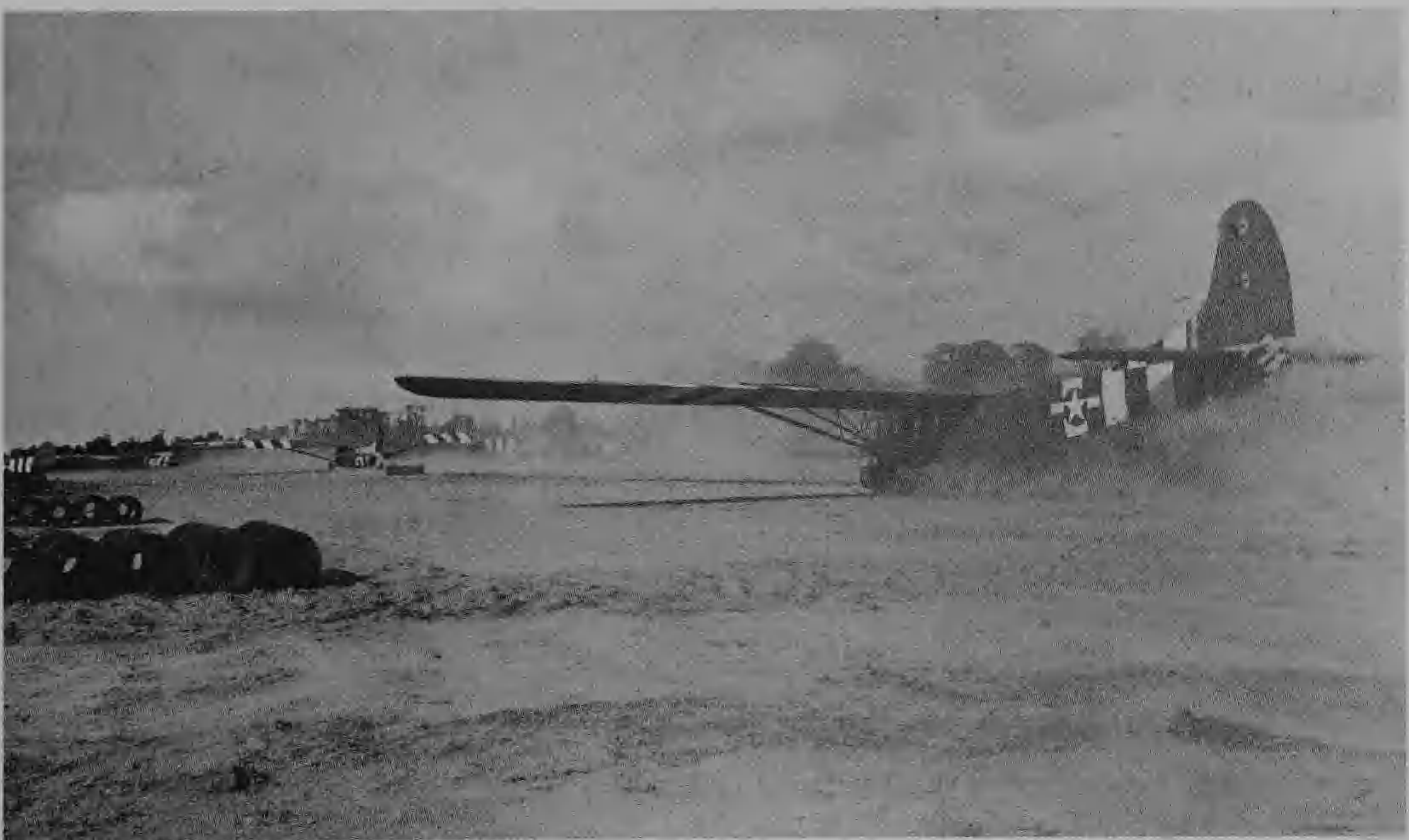
Waco CG-4A gliders with D-Day markings landing at a rough strip. The CG-4A could carry thirteen troops. (USAF)
