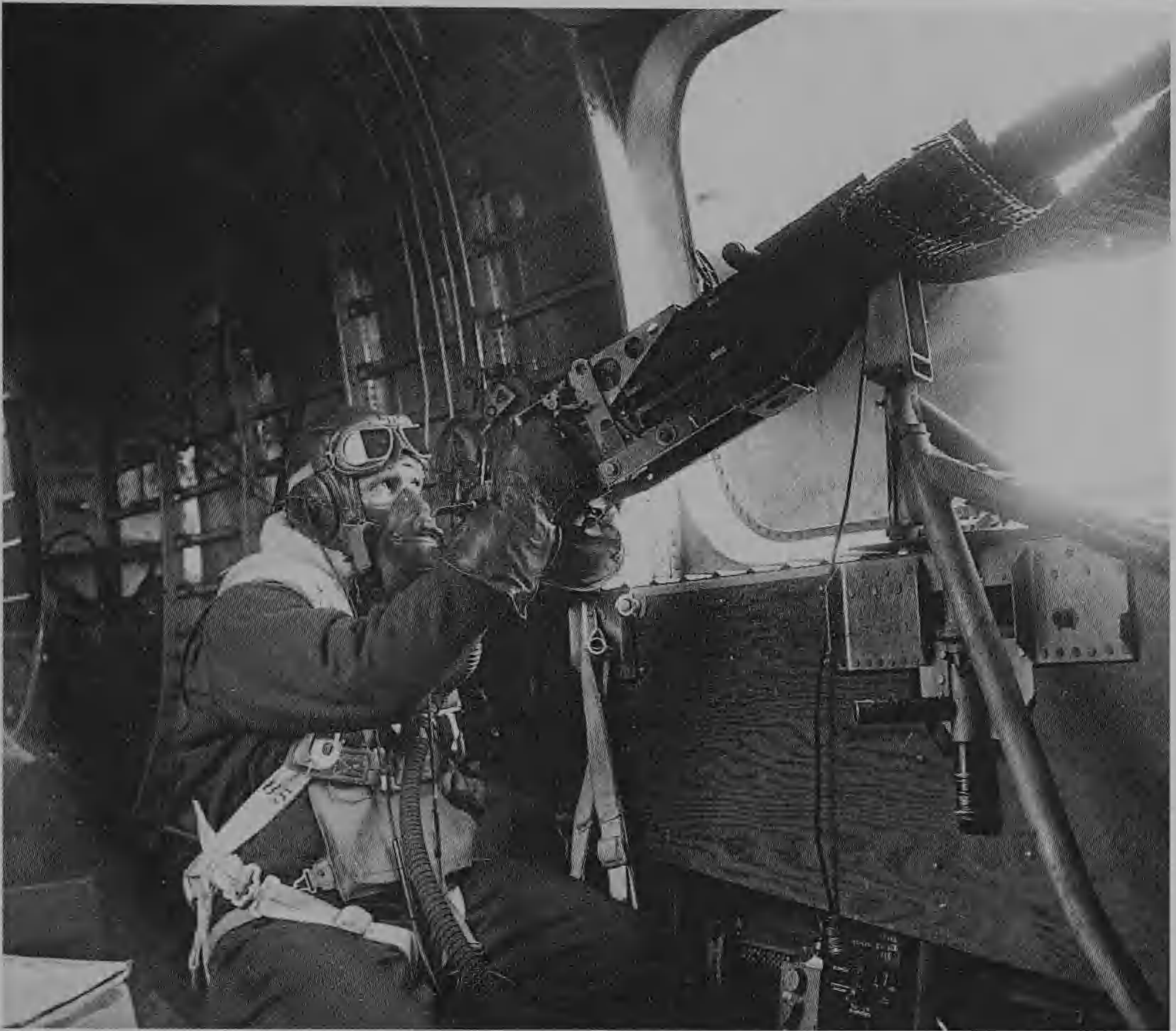
B-24 Betta Duck , 34th BG, waist gunner at his position in F-2 electric suit, with extremely rare white fur collar, and gloves, A-11 winter helmet, RAF Mk VIII goggles with tinted lenses, A-14 oxygen mask and 6 ft extension oxygen tube, chest parachute harness, and B-4 life preserver. The intercom jack box is visible below the gun mount. (via Mike Bailey)
