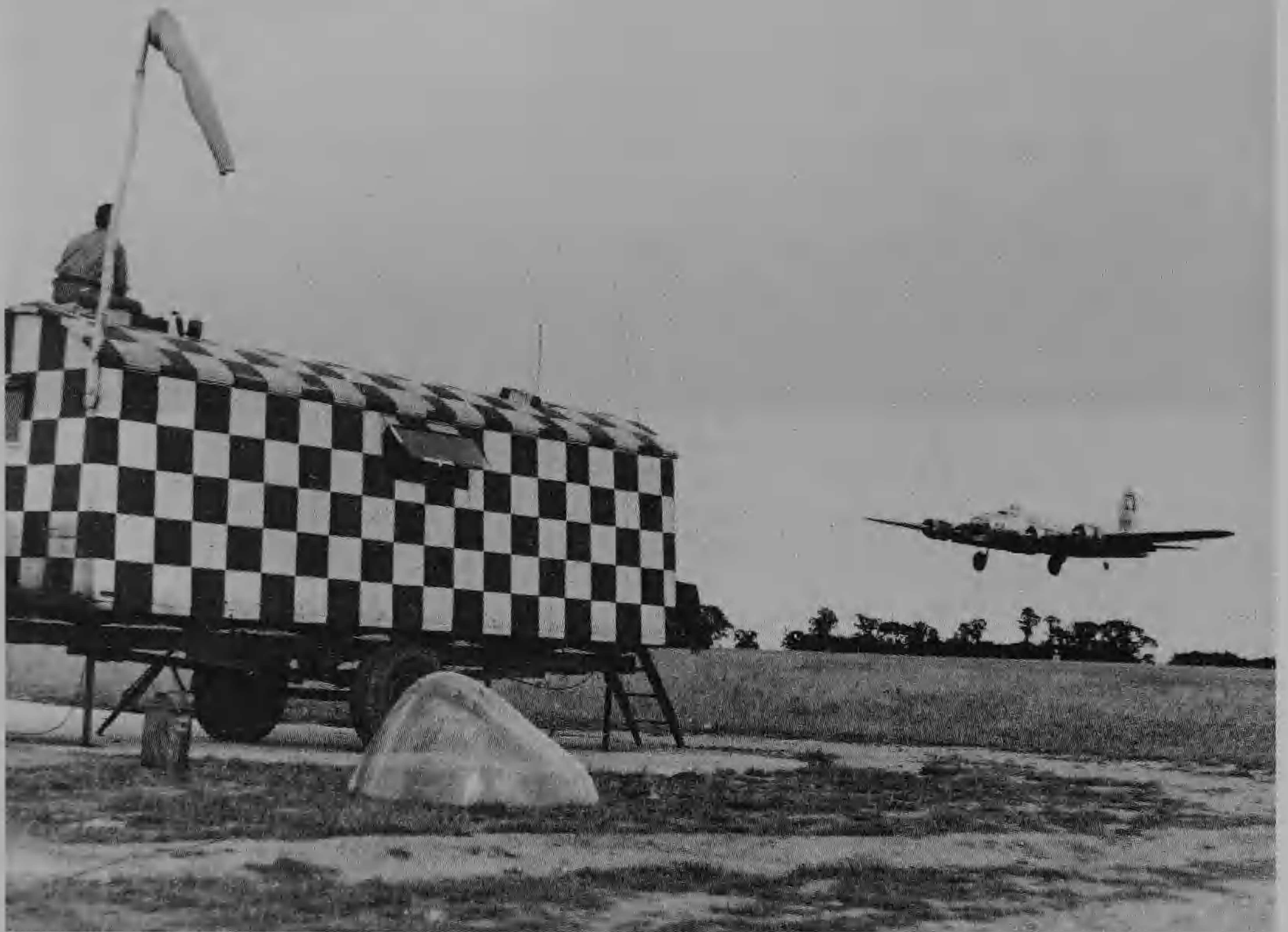
A B-17 comes into land past a black-and-white chequered runway control caravan. These were often obtained locally and highly improvised (note the domed observation canopy, a B-17 Plexiglas nose). (USAF)
