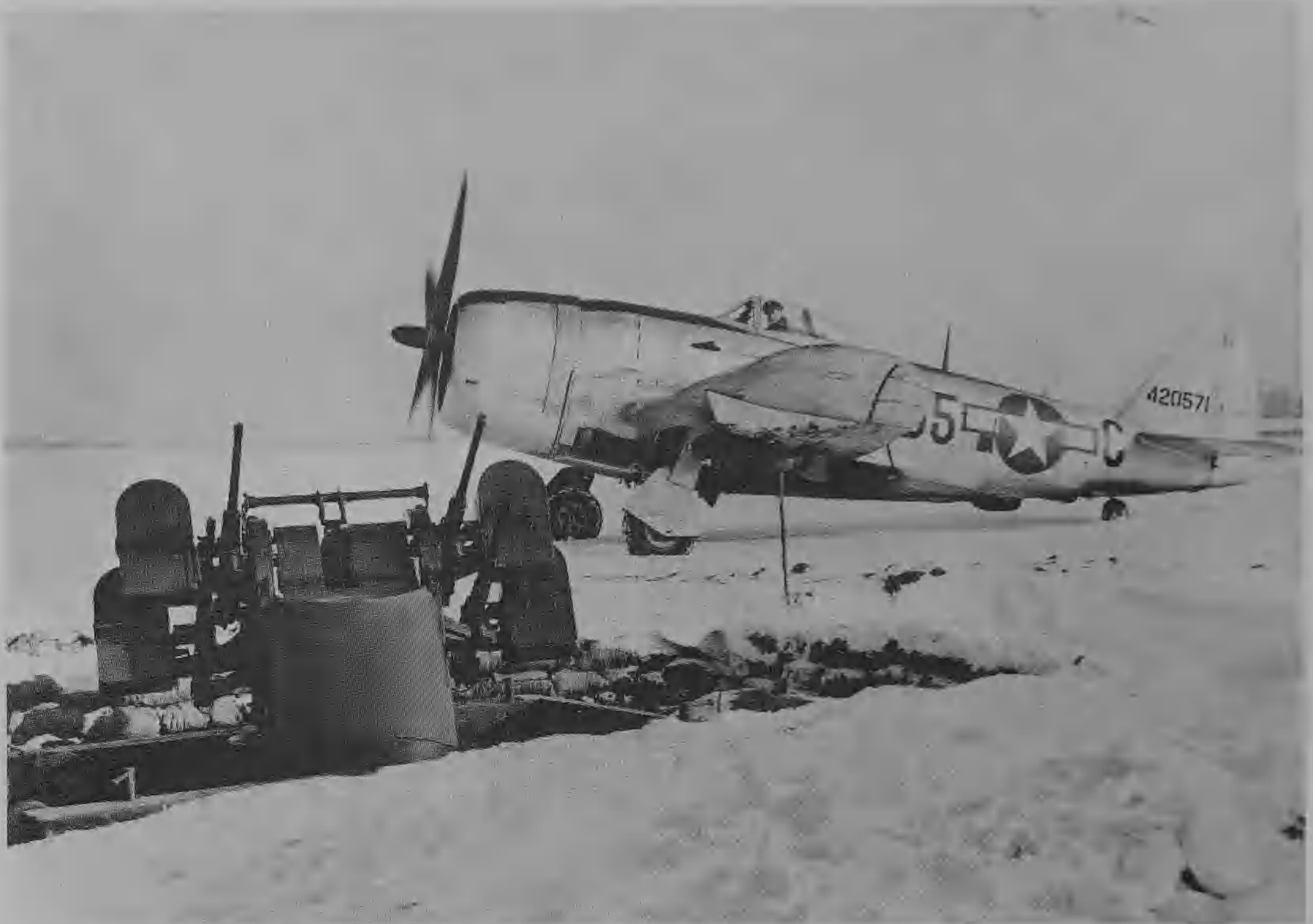
365th FG P-47D-RE 44-20571 on a snowbound airfield next to a four × .50 in AA quad mount, normally mounted on half-tracks, used for airfield defence. One of these quads shot down and killed George Preddy of the 328th FS, 352nd FG, 8th AF, on Christmas Day 1944. (USAF)
