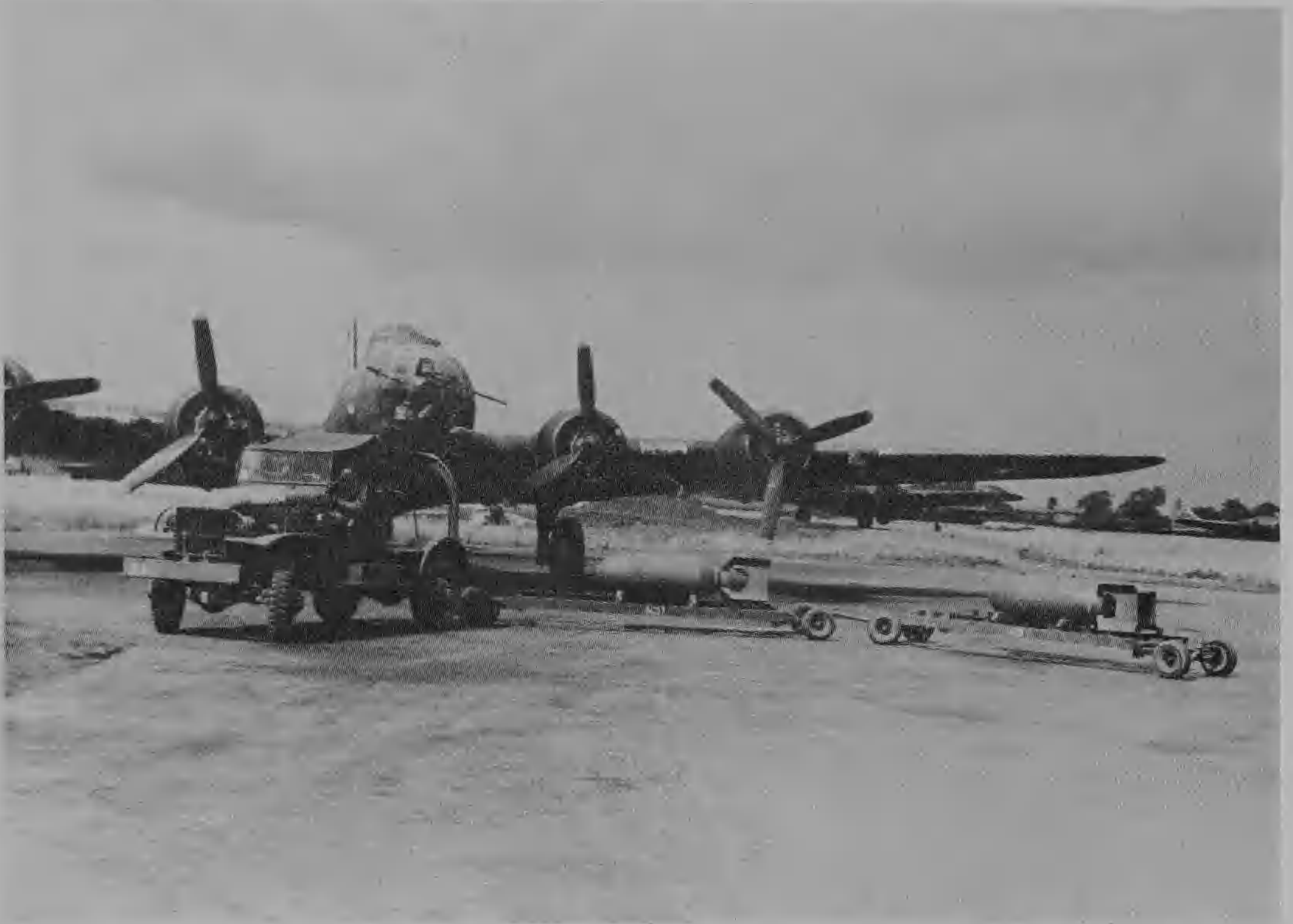
B-17F Lucky Strike of the 303rd BG, 8th AF, at Molesworth being loaded with bombs by a Chevrolet M6 4 × 4 1½ ton bomb service truck. The 303rd flew its first mission on 17 November 1942. (USAF)
