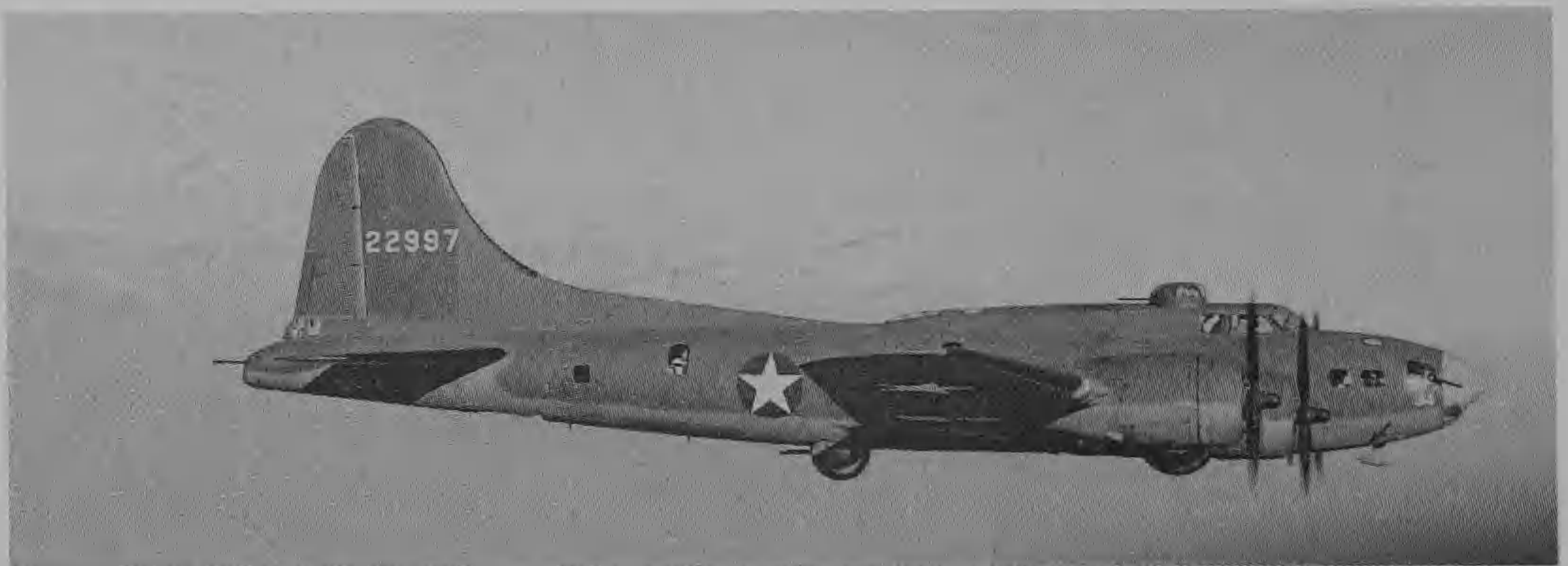
B-17F-10-DL showing the cheek gun, tail, mid-upper and ball turret positions. A radio hatch gun was also mounted in an attempt to improve firepower, but was largely ineffective. (McDonnell Douglas)
