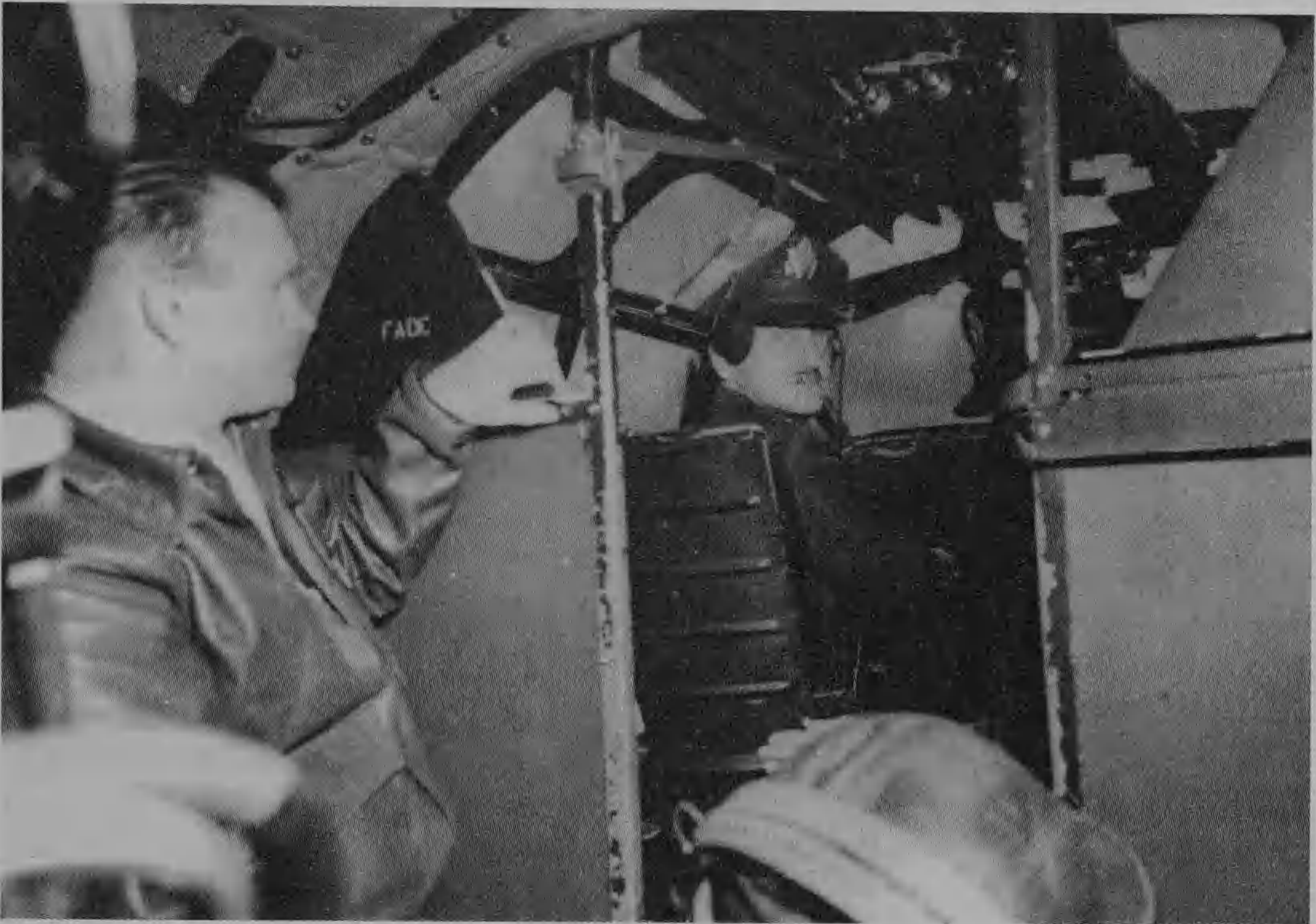
Cockpit interior of a B-24D Liberator showing flak curtains which were fitted during production behind the pilots' seats, the left one occupied on this occasion by Gen. Carl A. Spaatz. Armour was installed here and in the waist and bulkhead sections to reduce possible damage from enemy fighter attacks from the rear, but was deleted on subsequent models as tactics changed. (USAF via Mike Bailey)
