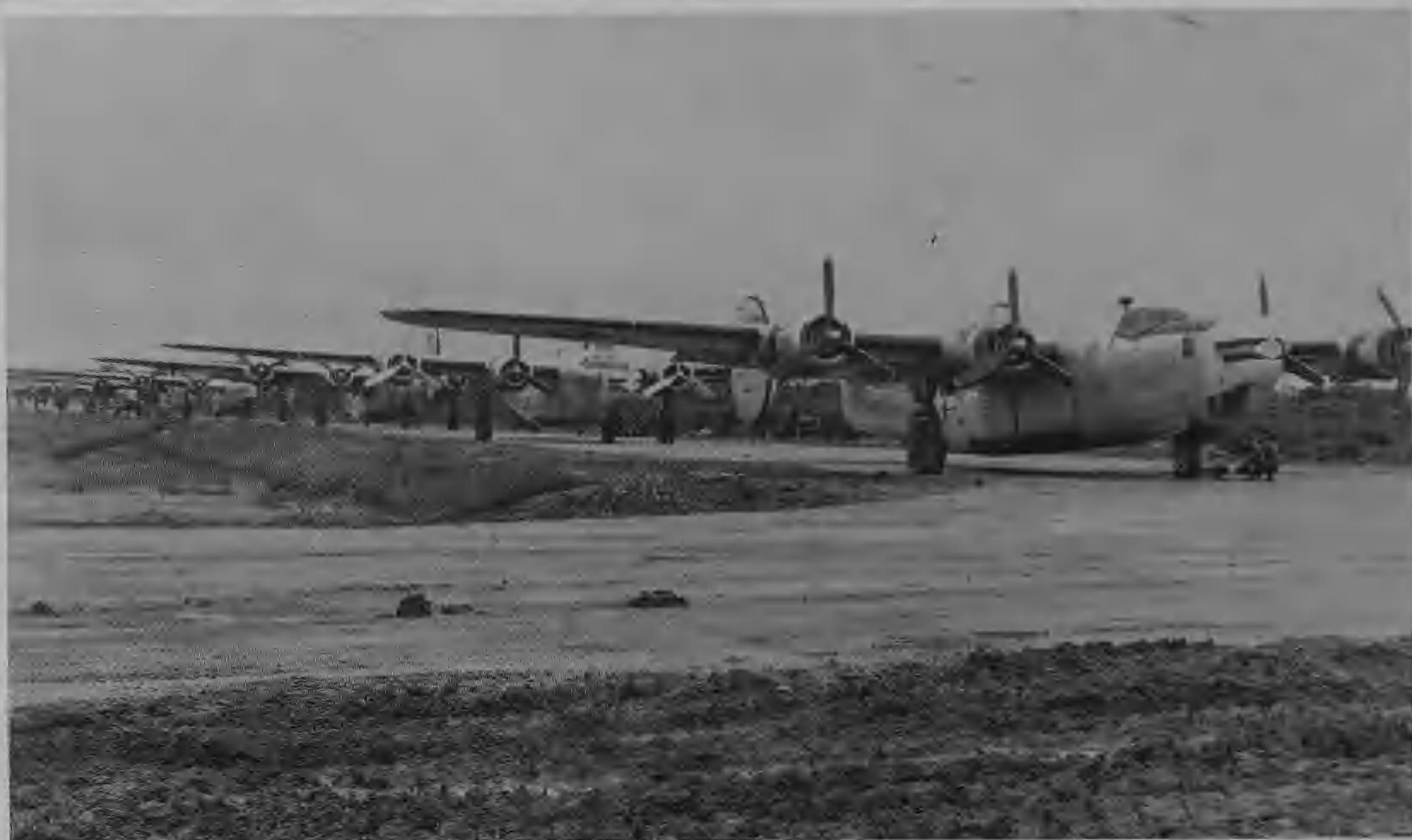
Fleet of C-109 'flying tankers' at a base in India. These converted B-24J/L Liberators had a capacity of 2,900 US gallons and were used very successfully to ferry fuel to advanced bases in China for B-29s. (B-24 Liberator Club)
