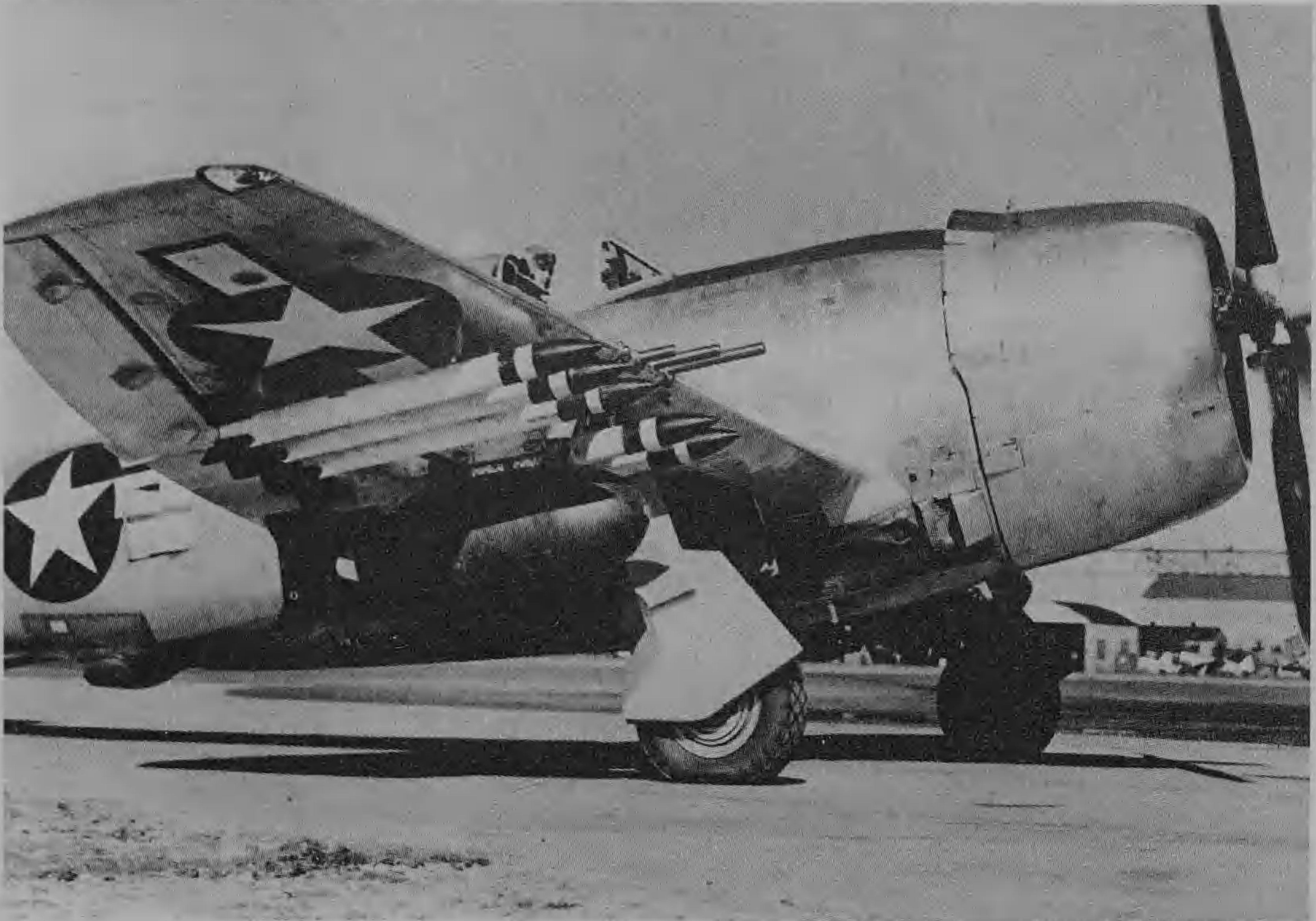
Republic P-47 Thunderbolt, armed with eight .50 in machine-guns in the wings, and underwing .5 in rockets. (USAF)
