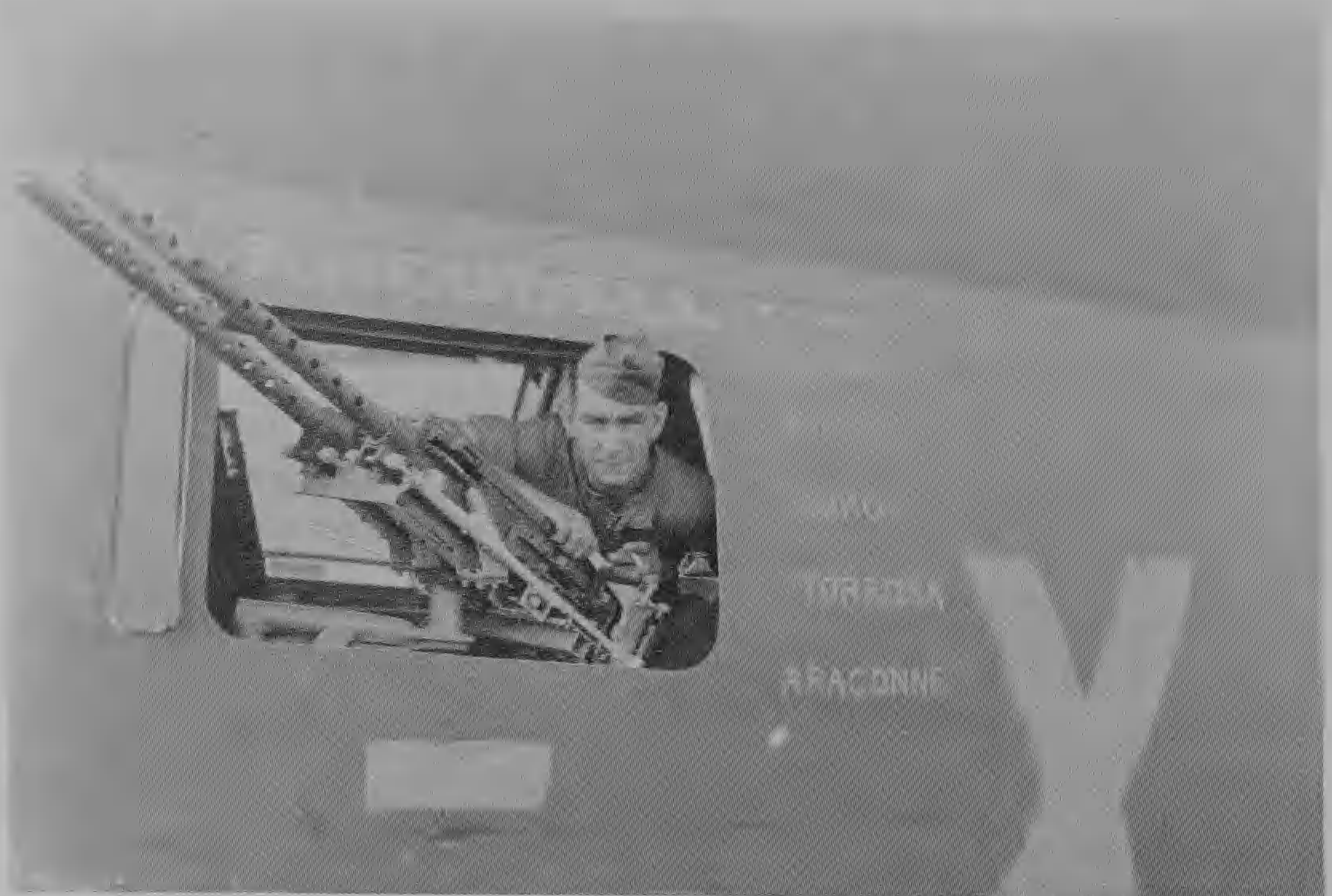
Field-modified twin .50 in Browning installation in the waist gun position of a 350th BS, 100th BG, B-17. The towns listed are from the time the gunner, Corporal Jerome E. Ferroggiaro, spent fighting in the Spanish Civil War. 'RHEUDELL' perhaps refers to the Indian waist gunner, 'Paddy' Blaizier. An open waist hatch was a very cold place to be at altitude, and the wind deflector helped. (Thorpe Abbotts Memorial Museum)
