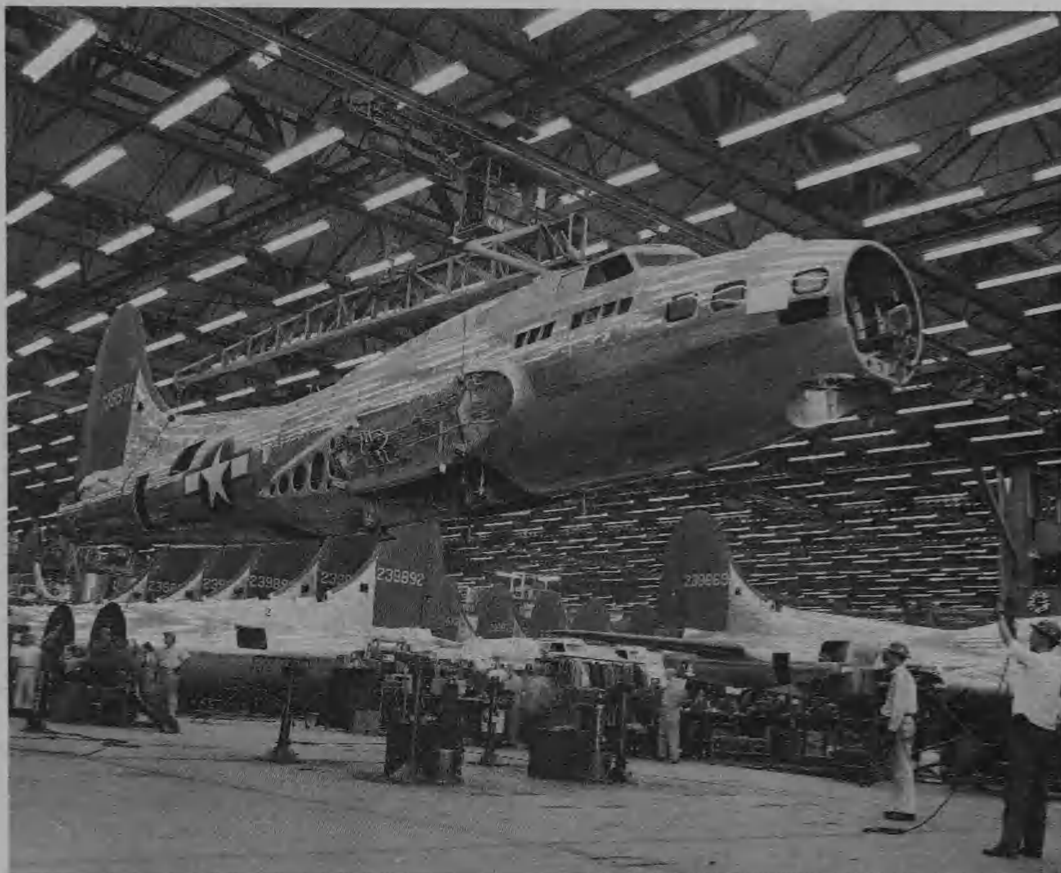
B-17s were built at three wartime plants and were identified by their respective block number designations: Boeing Aircraft at Seattle, Washington (B-17-BO); Douglas Aircraft, Long Beach, California (B-17-DL), and Lockheed-Vega, Burbank, California (B-17-VE). These are B-17G-5-VE models from the 42-39758/40057 batch, ordered in 1942 and built by Vega. (Lockheed-California)
