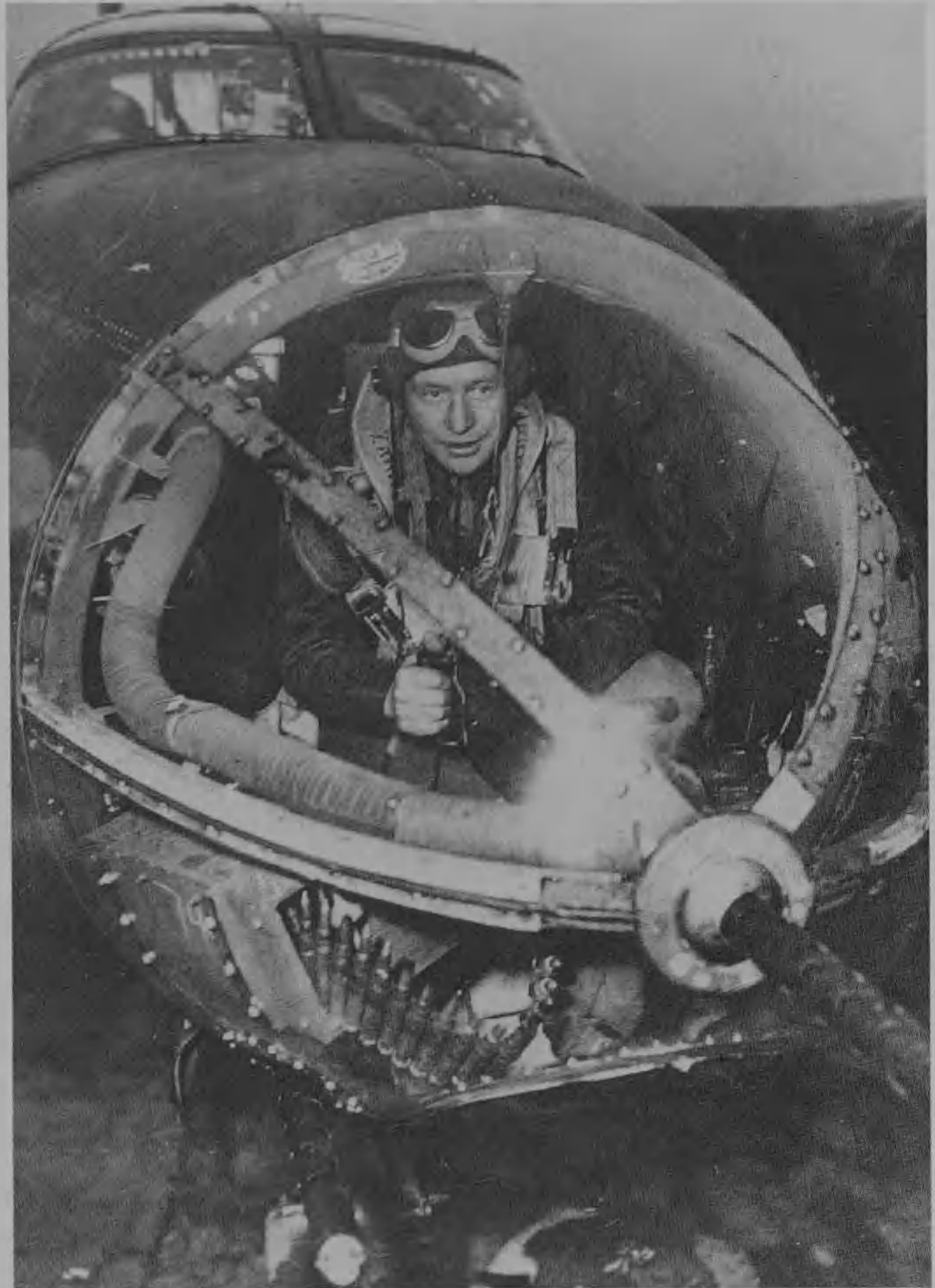
2nd Lt. William Zarhrte of Wisconsin wearing B-7 goggles, manning the flexible nose gun of a B-26 Marauder. The gun to his lower right is a fixed weapon which is fired by the pilot from the flight deck. (USAF)
