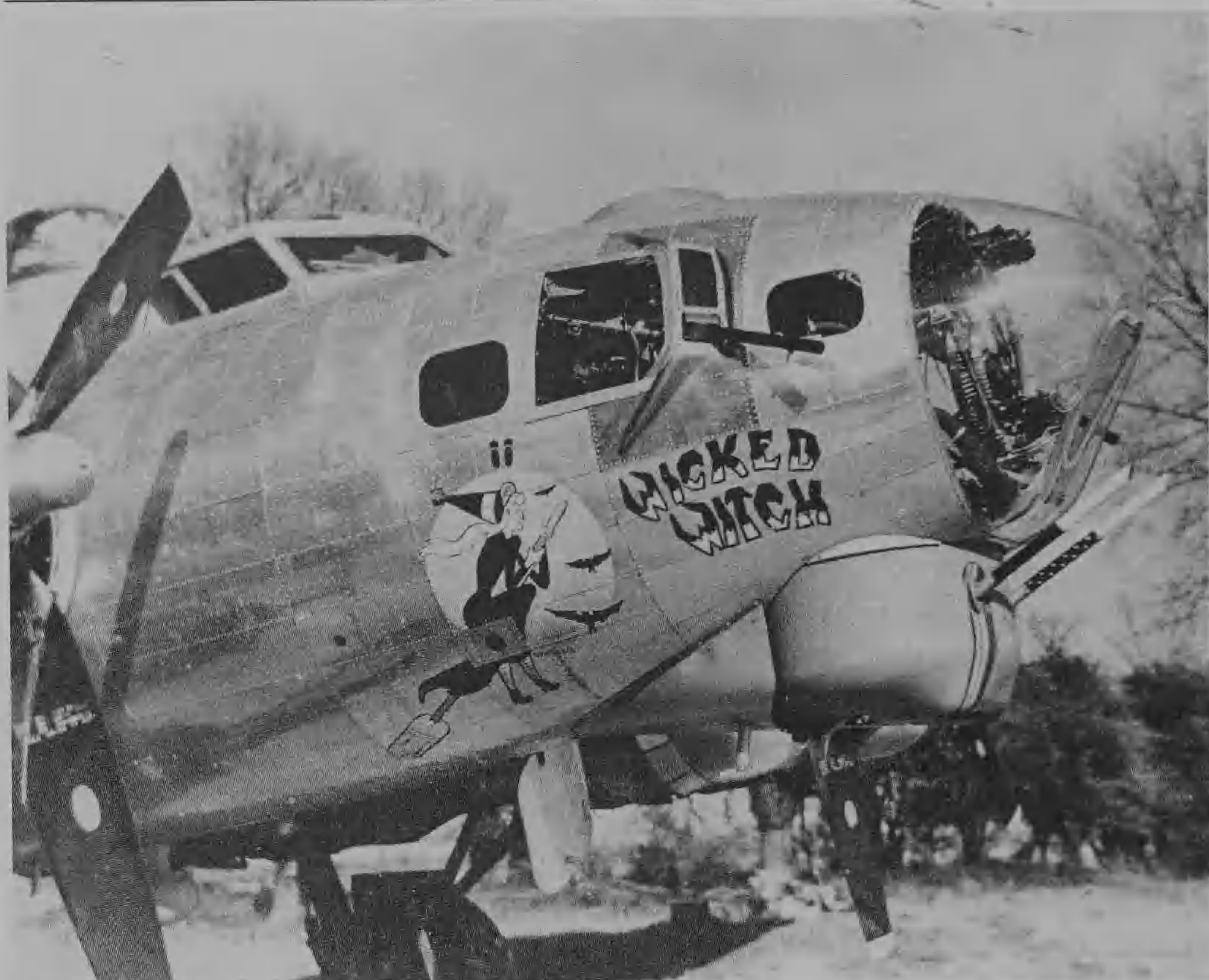
B-17G Wicked Witch , 91st BG, 8th AF, showing the chin turret installation which added much needed frontal firepower to help combat head-on attacks by the Luftwaffe. (USAF)
