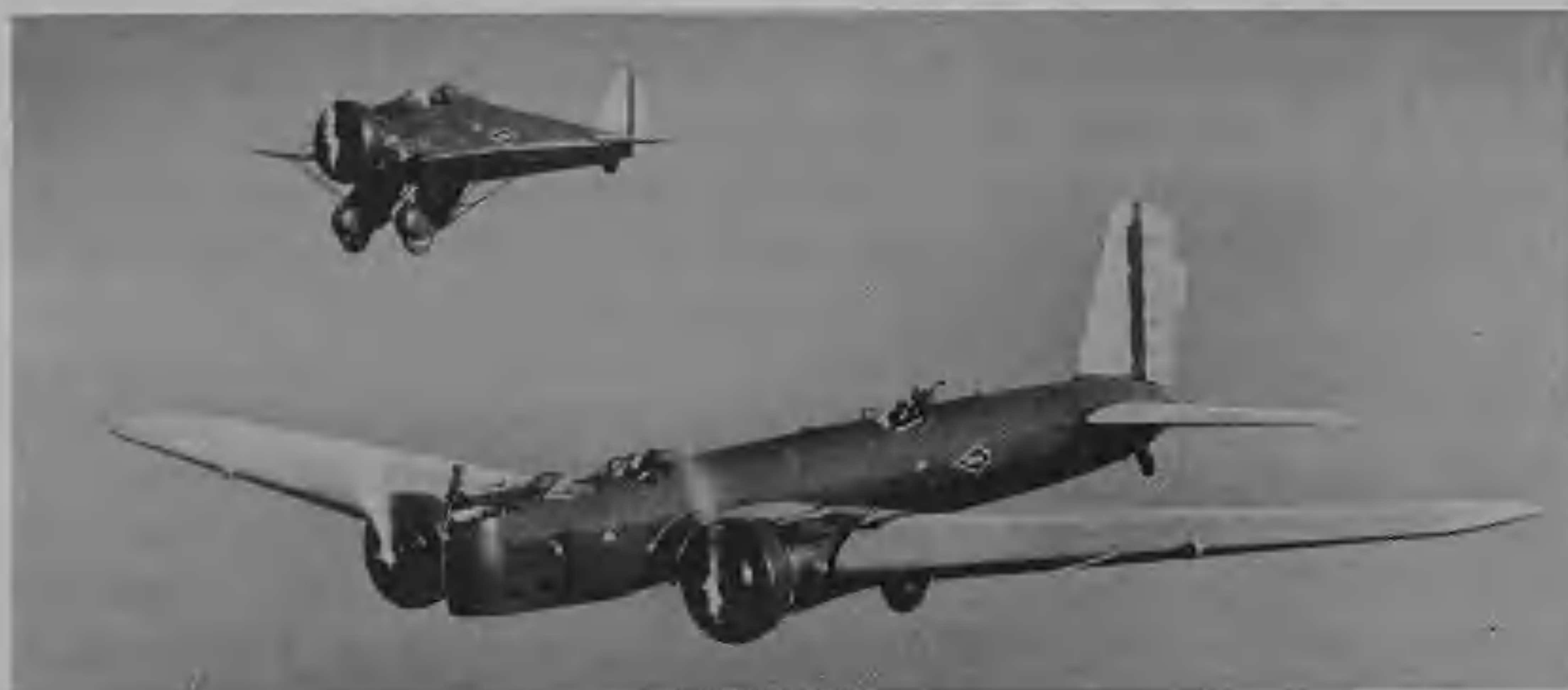
Boeing Y1B-9A (Model 246), one of five service test aircraft, in flight with a P-26A in 1933. The B-9 was the first Boeing bomber design. Only seven examples were built, the AAC opting instead for the equally revolutionary Martin B-10. (Boeing)
