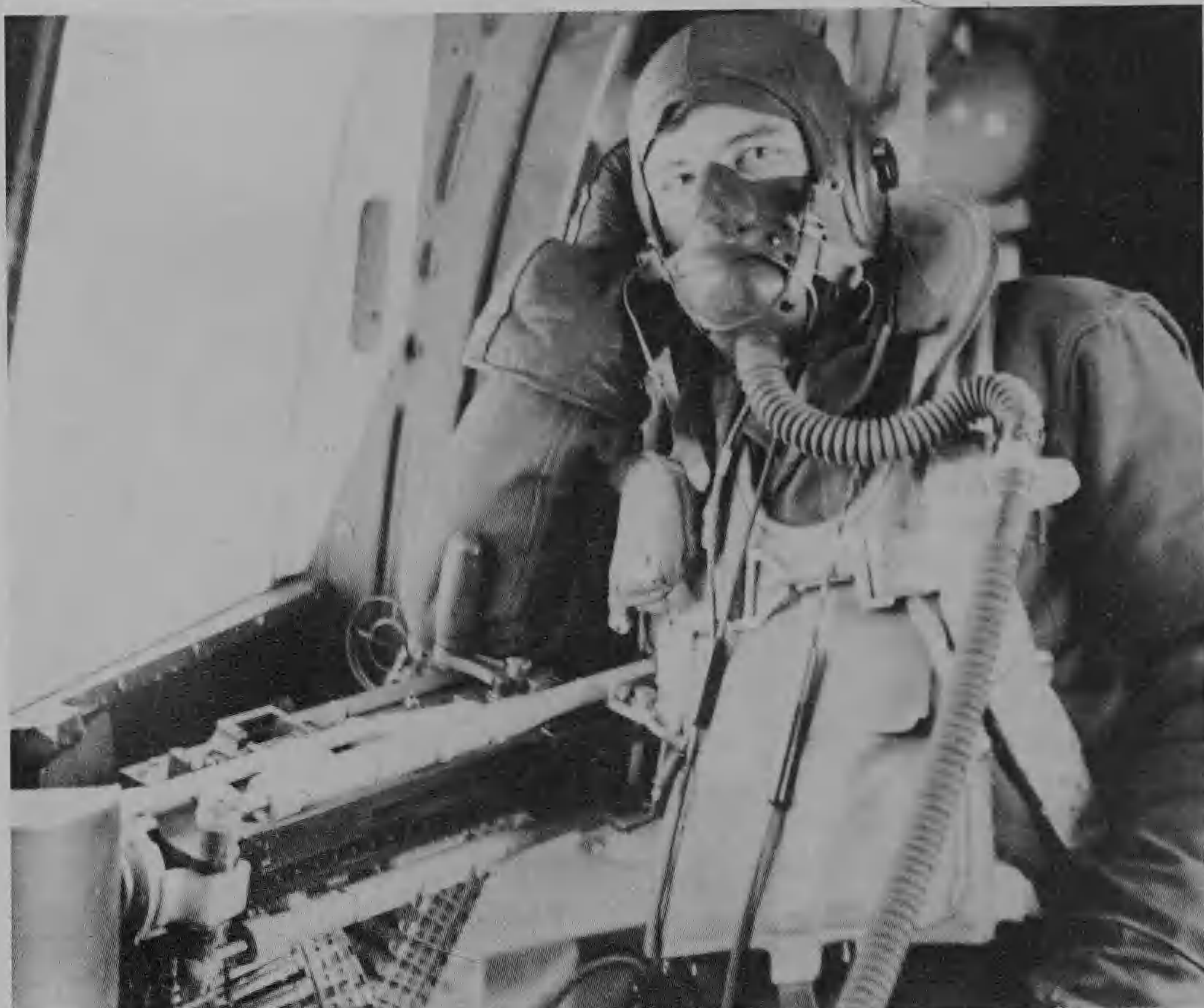
B-24 waist gunner wearing an A-11 winter flying helmet, F-2 electric gloves, B-4 life preserver and A-14 oxygen mask. A type A-3 oxygen indicator on a panel in the aircraft told the recipient how much pressure was being exerted in the system. A warning light would glow when the pressure reached 100 lb. (USAF)
