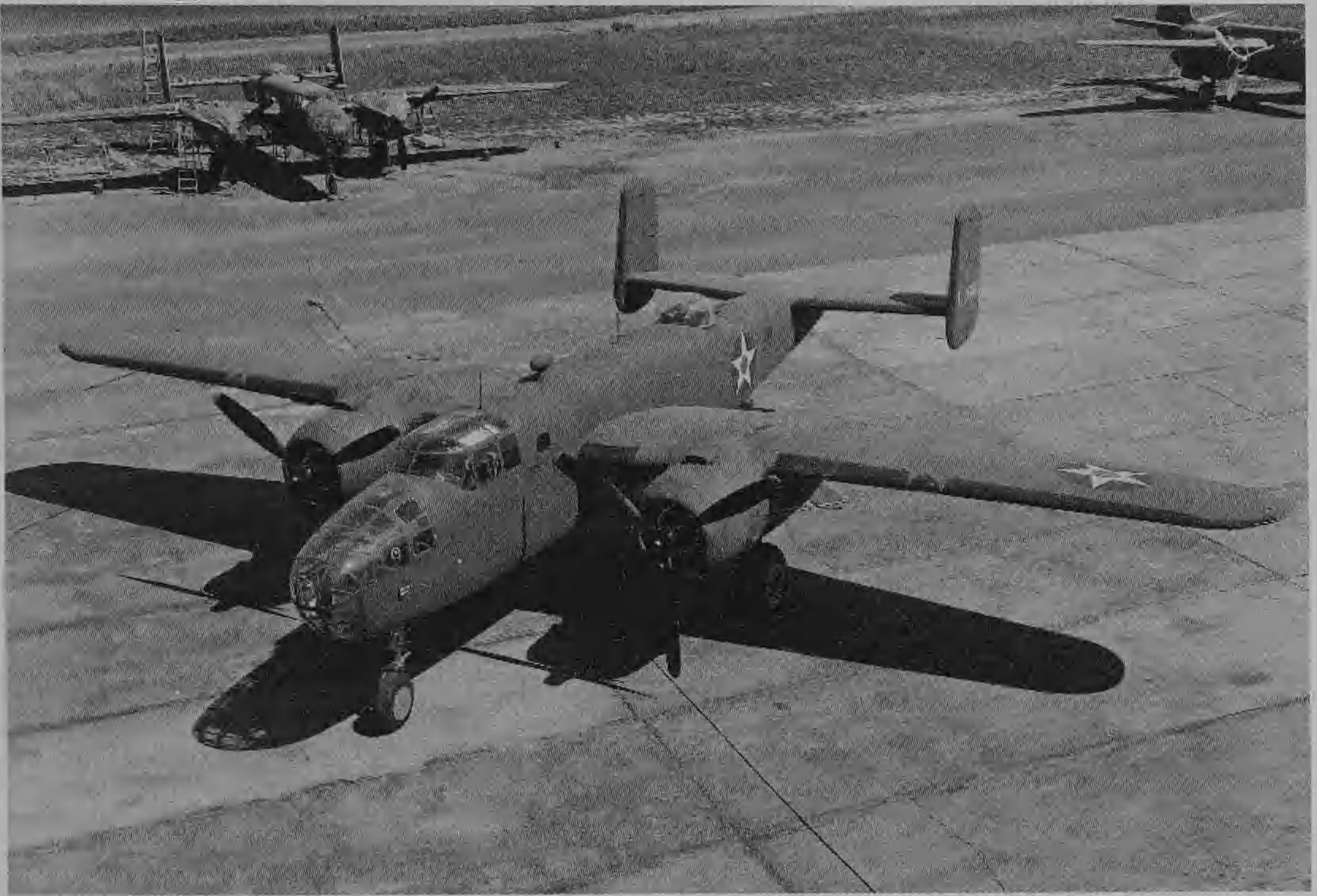
B-25C Mitchell 41-12633 and an A-20 on the line in very early war markings. Deliveries of the B-25C began in 1941. The B-25C had Bendix electric mid-upper and retractable underbelly turrets. The tail gun was deleted. (via Mike Bailey)
