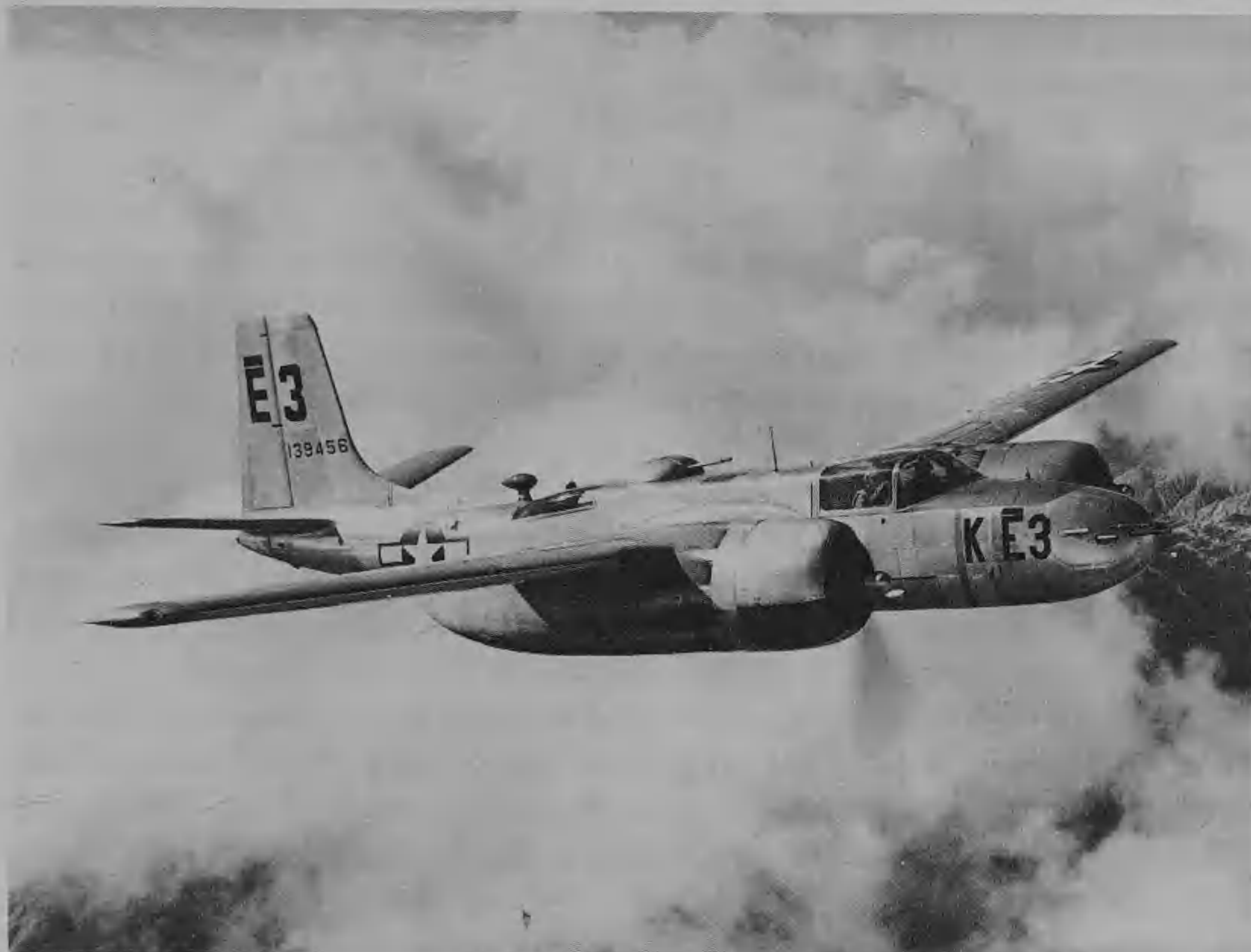
A-26B-DL Invader 41-39456 with six .50 in machine-guns in the nose and remote-controlled dorsal and ventral turrets. Eight more guns could be added – two each side of the nose and four under the wings. (USAF)
