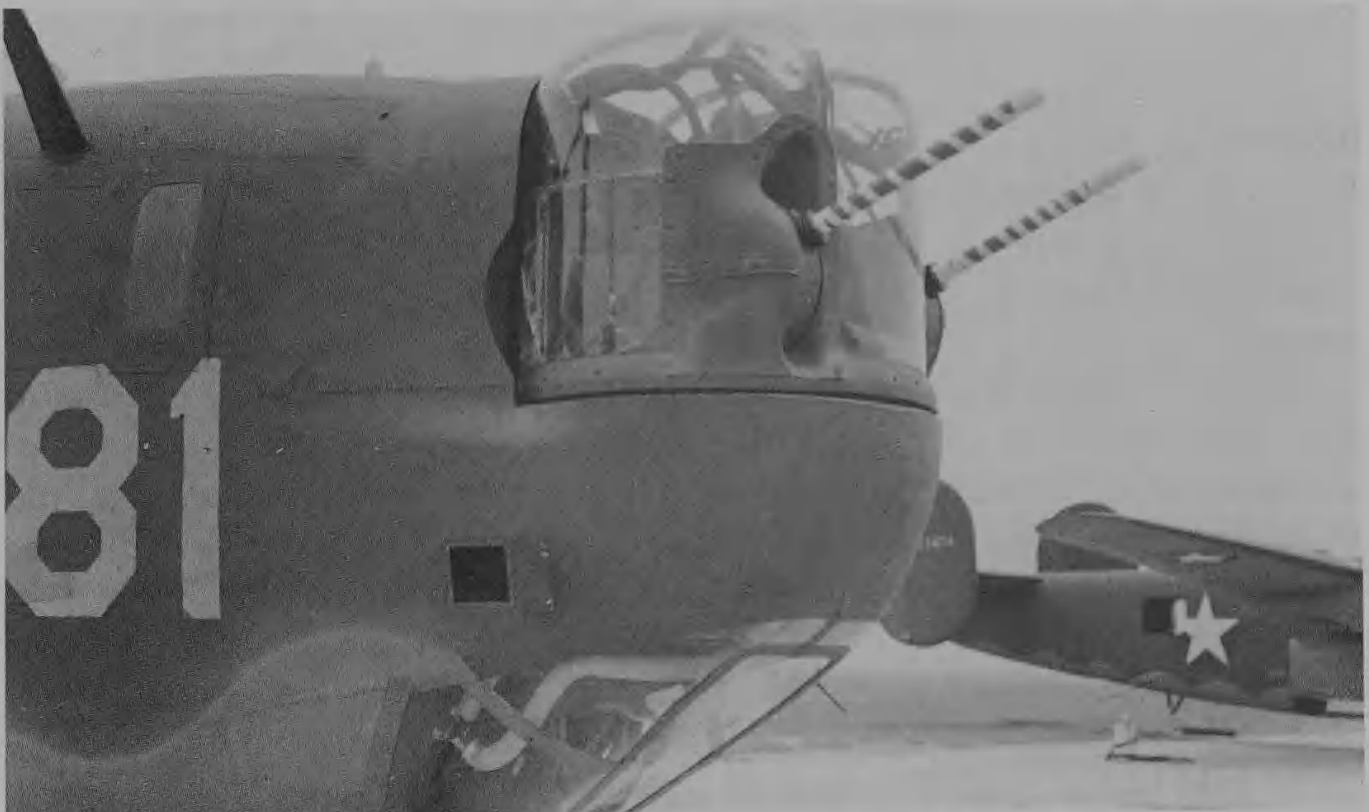
Ford-built B-24H showing the Emerson nose turret and the company's distinctive 'way demarcation line' which separated the OD upper surface and grey lower surface. (Different B-24 manufacturers also had distinctively shaped black anti-dazzle panels atop the noses.) In the bombardier's window, the white heater tube known as the 'Elephant's pecker', which heated the bombsight and optical glass, can be seen. The open entry port is to allow ammunition to be fed into the nose guns, covered here for protection against the elements. (USAF)
