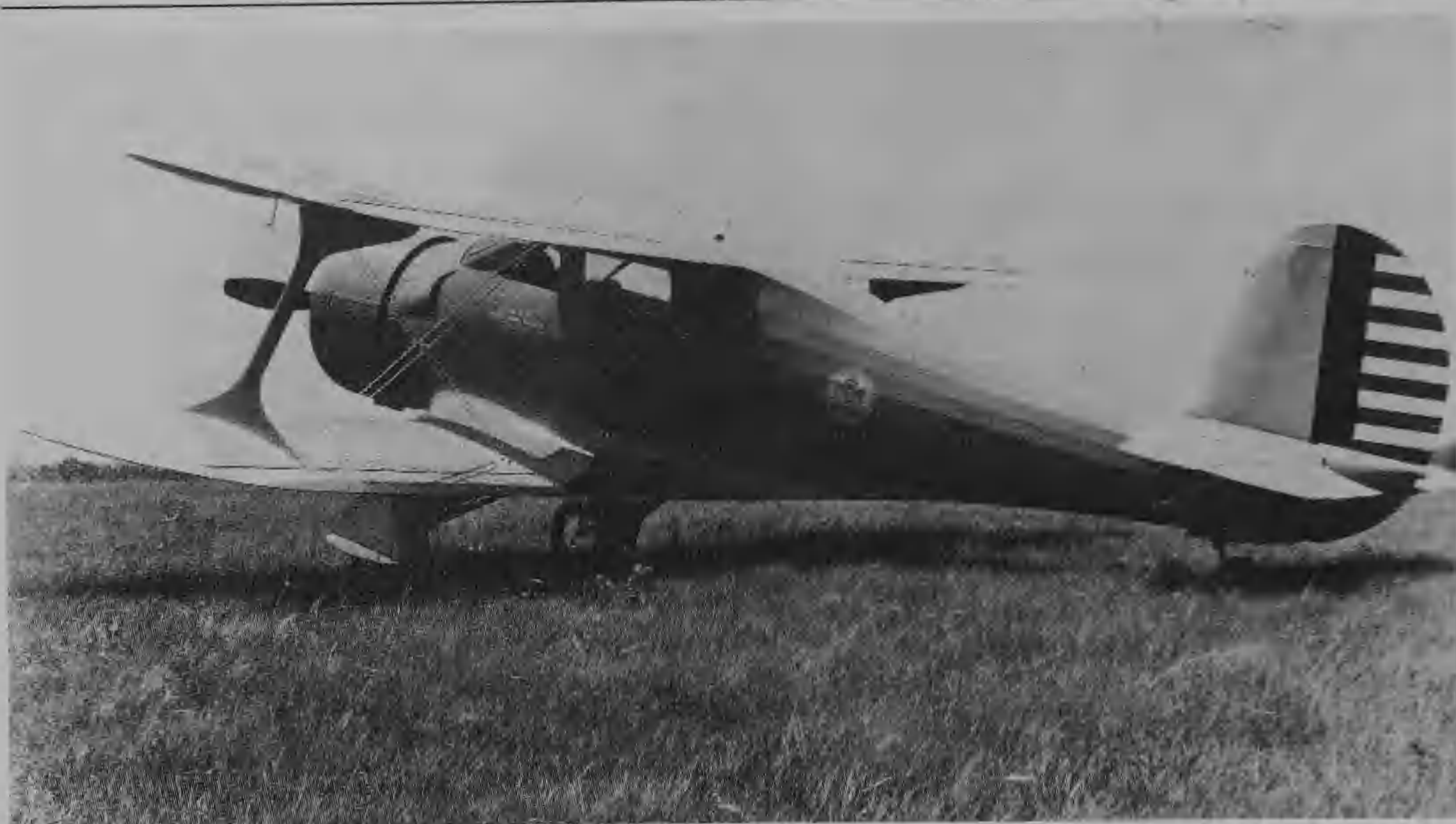
Beechcraft YC-43 39-139 of the US Embassy, London, one of three examples of the pre-war commercial D-17S used by the AAC. (Beech)
