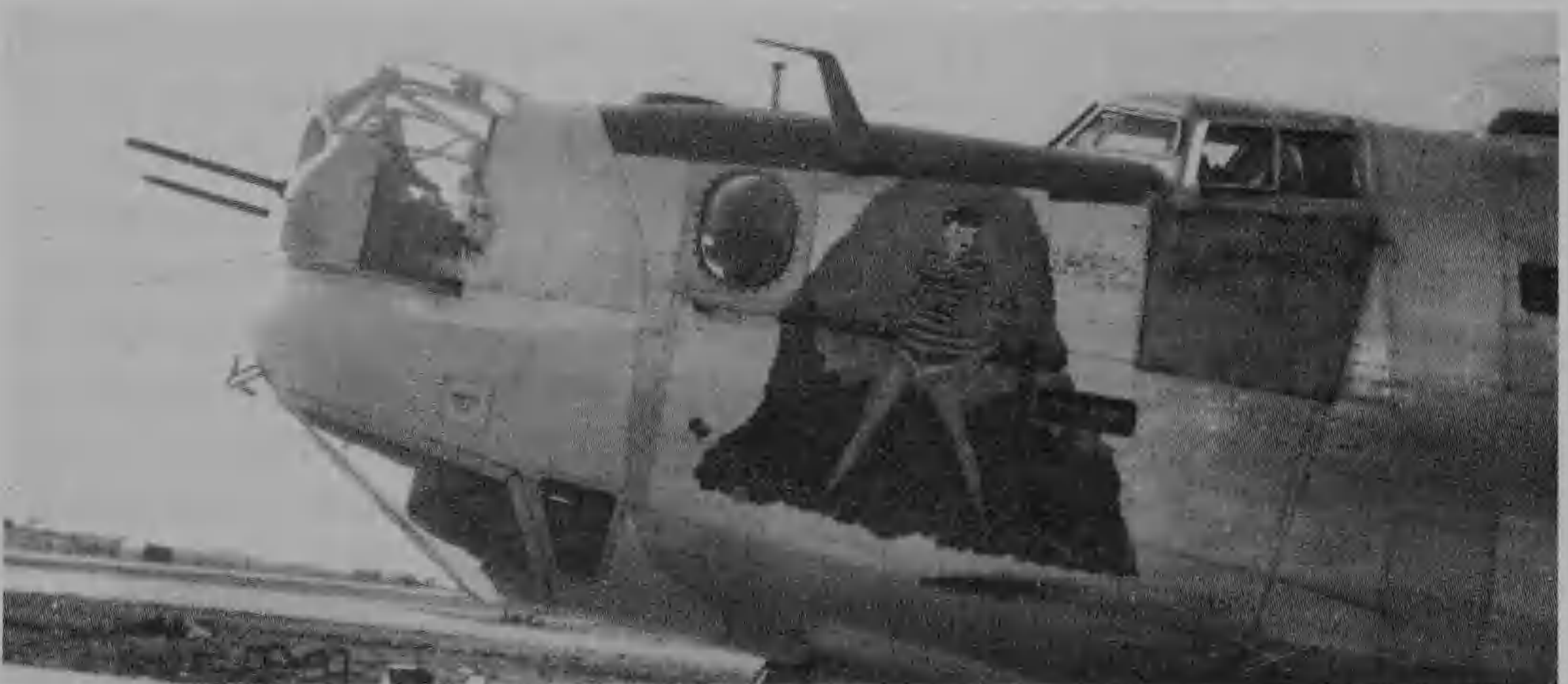
B-24J-1-FO Liberator Miss B-Haven of the 448th BG, Seething. Thick boilerplate obtained from British sources has been fixed to both sides of the pilots' compartment for added protection, while the Plexiglas in the front and side windows of the cockpit has been replaced by armoured glass. (Ford-built Liberators often had, on the flight deck, 'coffin'-style armoured seats which enclosed the head and body of the pilot, but this innovation proved unpopular and was later deleted.) A 'bubble'-style blister window has been installed to improve the navigator's all-round vision. Below the Emerson turret is the 'fishhook' Carpet antenna. (USAF)
