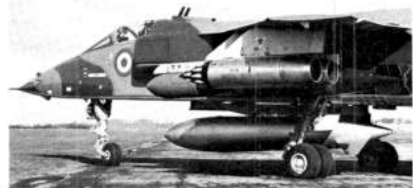
Typical stores 'mix' of fuel tank, bombs and SNEB rocket pods
