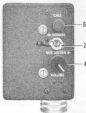
AUXILIARY INTERPHONE CONTROL PANEL
