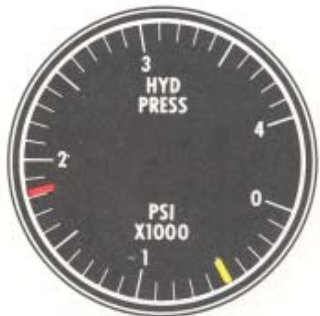
EMERGENCY BRAKE HYDRAULIC PRESSURE
