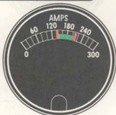
PROPELLER DE-ICING AMMETER PLUS 1010 534
