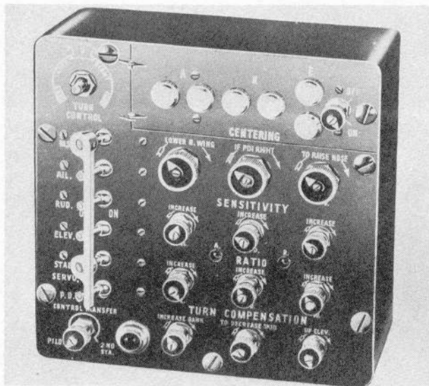
Figure 8 — Automatic Pilot Controls Panel
