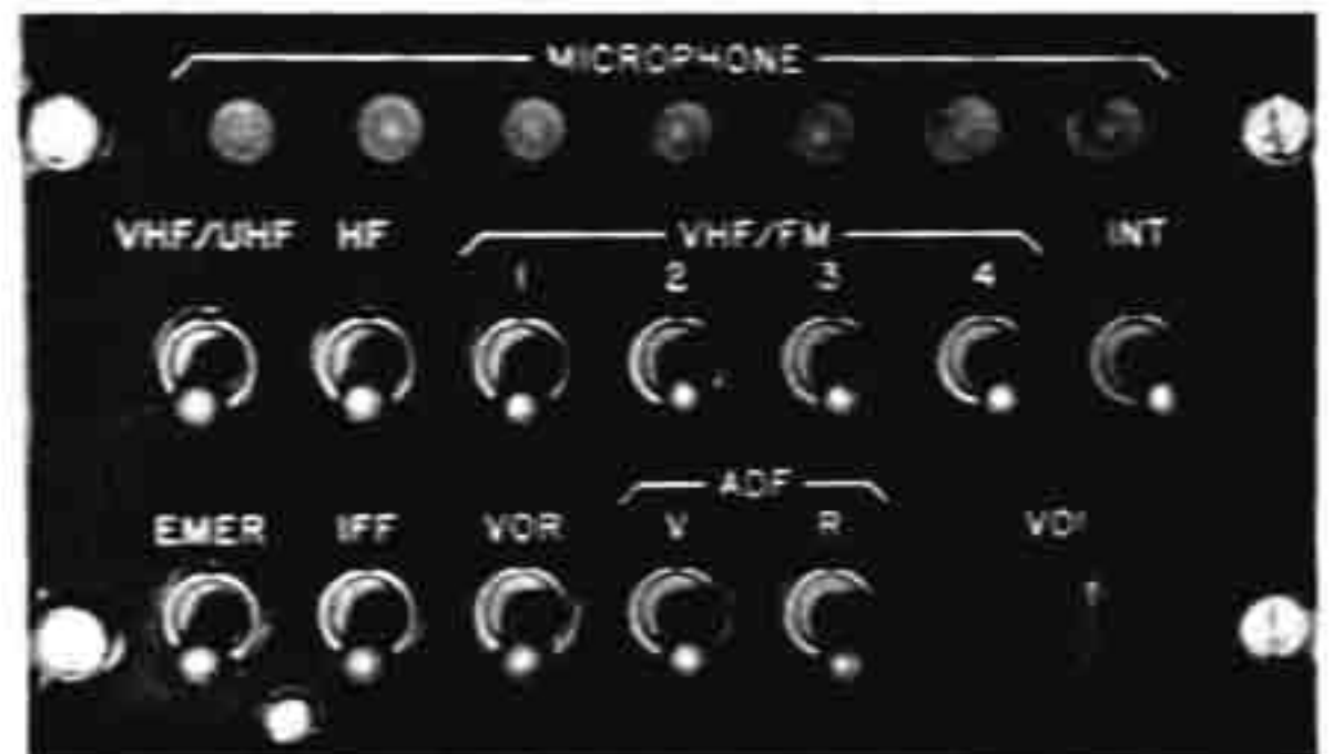
Fig. 1-36 Signal Distribution Panel
