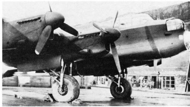
(Above) A Lancaster B Mk III serving with No 617 Squadron (after code letters had been changed from "AJ" to "KC"), with deepened bomb-bay to accommodate the 12,000-lb (5 443-kg) Tallboy bomb. (Below) The first Lancaster modified to carry the 22,000-lb (9 980-kg) Grand Slam, at Boscombe Down for trials.
