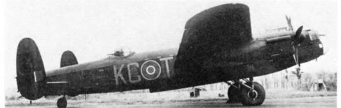
(Above) A Lancaster B Mk III serving with No 617 Squadron (after code letters had been changed from "AJ" to "KC"), with deepened bomb-bay to accommodate the 12,000-lb (5 443-kg) Tallboy bomb. (Below) The first Lancaster modified to carry the 22,000-lb (9 980-kg) Grand Slam, at Boscombe Down for trials.
