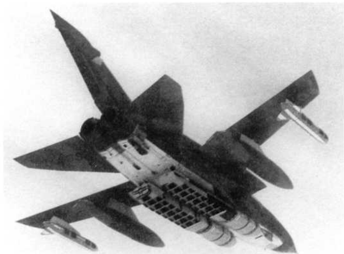
One of the important additions to the RAF's armoury, recently ordered into production, is the JP233 airfield denial weapon, seen here under test on a Tornado GR Mk 1.
