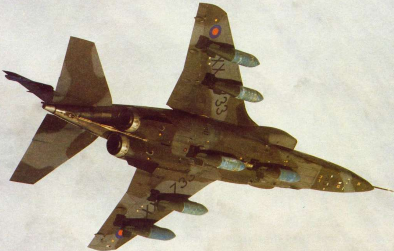
The Jaguar shares with the Harrier responsibility for providing No 38 Group with its attack capability. This example from Coltishall-based No 6 Squadron is carrying six 1,000-lb (454-kg) bombs on fuselage and wing strongpoints.
