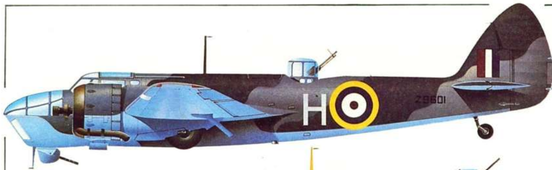
(Right) The Blenheim V, distinguished from the Mk IV by its changed nose contours, was flown in the Tunisian campaign by Nos 18 and 114 Squadrons.
