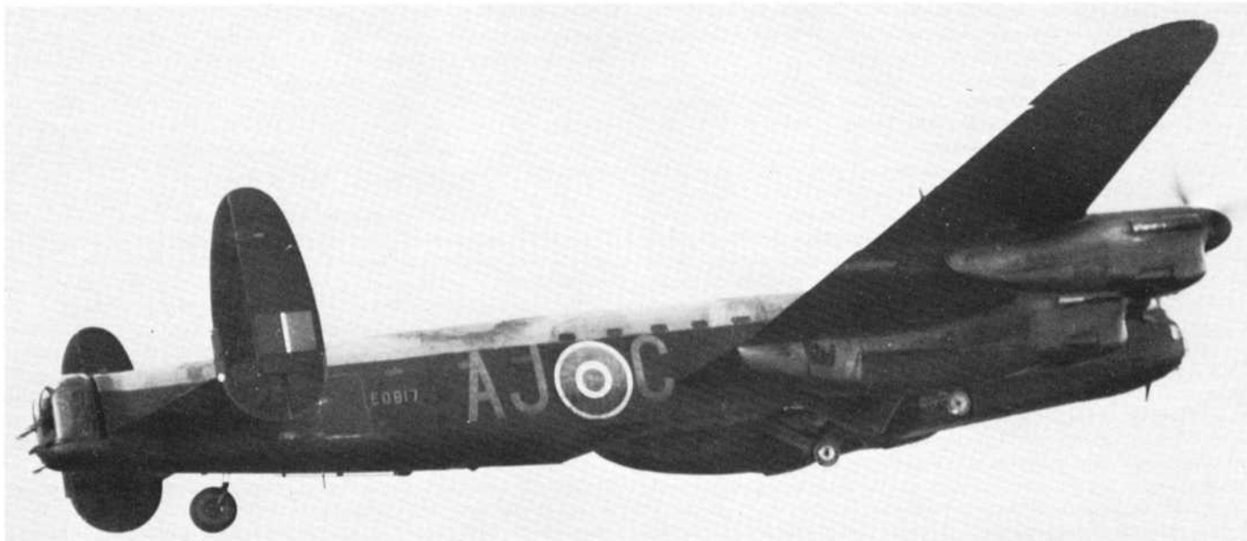
(Above) ED817 was one of 23 Lancasters modified to carry the "Upkeep" weapon used to break the Ruhr dams, but did not participate in the raid itself. This photograph clearly shows the struts between which the bomb was carried, to be spun up before dropping. (Below right) This rare shot of the Mohne dam, photographed shortly after the raid, was taken from a German serviceman in Normandy in 1944 and offered for publication here nearly 40 years later!
