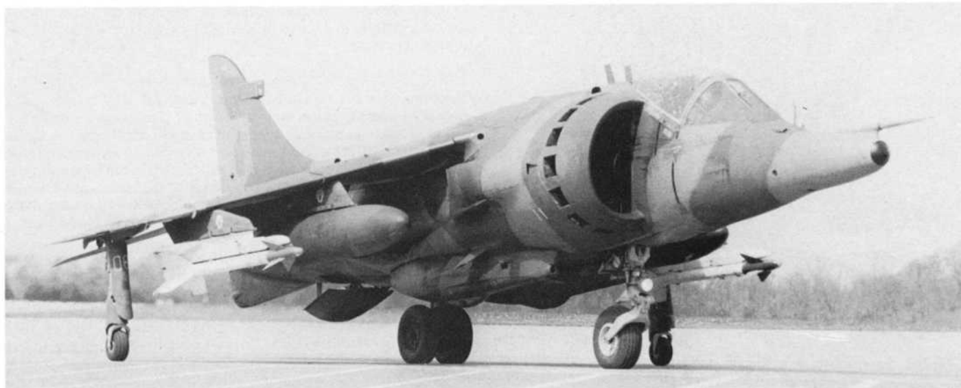
The armament of the Harrier GR Mk 3 was enhanced, before aircraft of No 1 Squadron were despatched to the South Atlantic, by adapting the outboard wing pylons to carry Sidewinder AAMs as an alternative to bombs or rocket pods. All GR Mk 3s have subsequently been modified to permit Sidewinder carriage.
