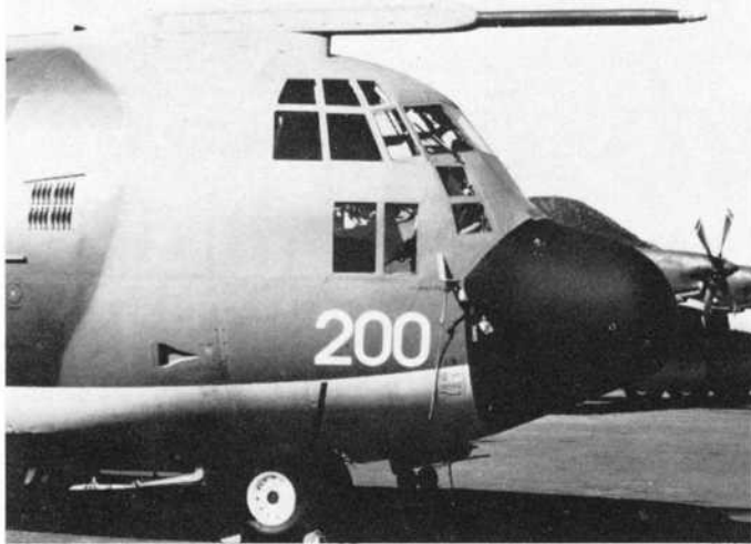
In the course of the Falklands conflict, both the Nimrod MR Mk 2 (above) and Hercules C Mk 1 (below) were given AAR capability. Sixteen of each type are now in service with probes.
