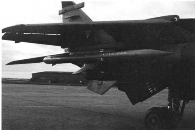
Future options for No 38 Group Jaguars are illustrated here as a trial installation. They are (above) the ALQ-101 ECM pod and (below) the Phimat chaff and flare dispenser.
