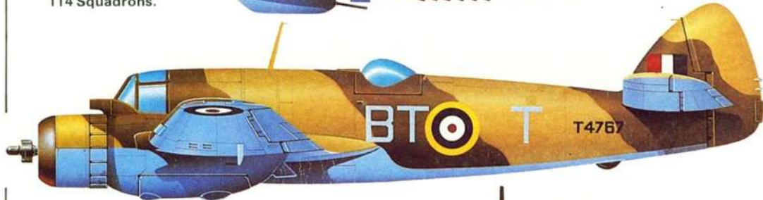
(Right) The Blenheim V, distinguished from the Mk IV by its changed nose contours, was flown in the Tunisian campaign by Nos 18 and 114 Squadrons.
