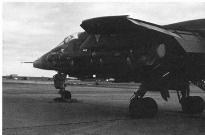
Future options for No 38 Group Jaguars are illustrated here as a trial installation. They are (above) the ALQ-101 ECM pod and (below) the Phimat chaff and flare dispenser.
