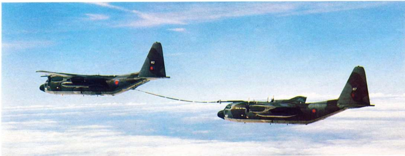
(Above) A Hercules C Mk 1, modified to have a refuelling probe, takes on fuel from a Hercules C Mk 1(K) tanker. Both conversions were made by Marshall of Cambridge (Engineering) at short notice during the Falklands campaign. (Below) Another view of a Hercules tanker.
