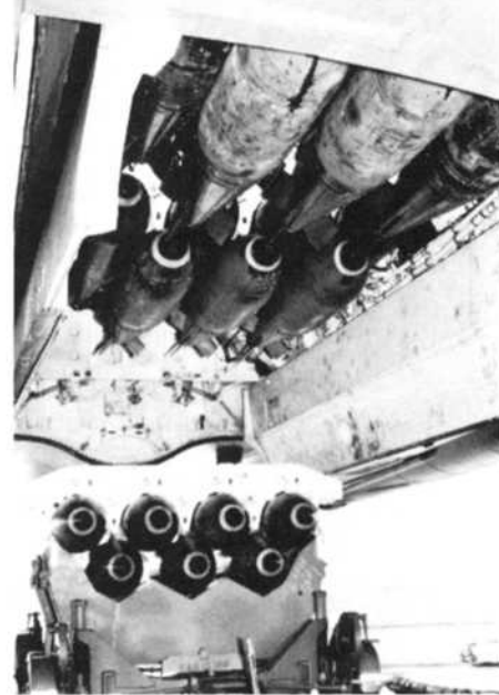
(Below) Two of the Vulcan B Mk 2s deployed at Wideawake for the Black Buck missions, and (above right) 1,000-lb (454-kg) HE bombs being loaded into the Vulcan's weapons bay.
