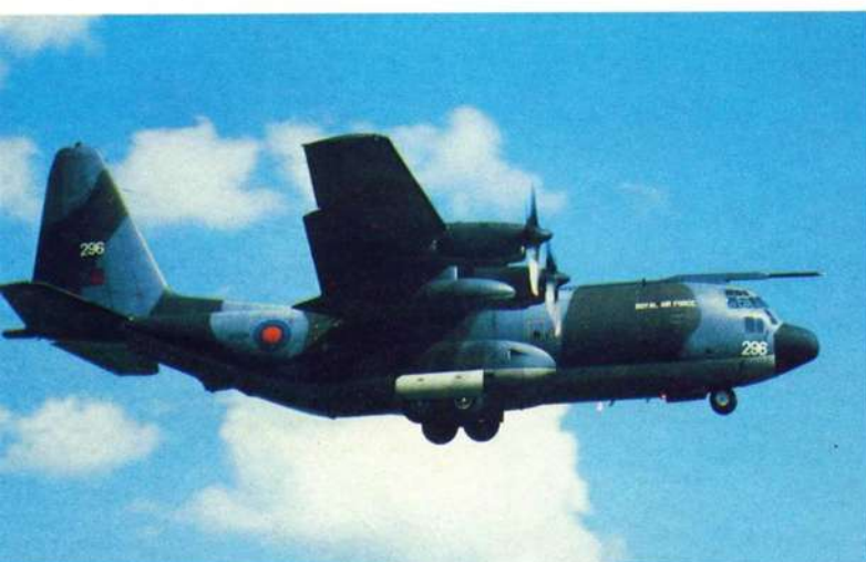
(Above) A Hercules C Mk 1, modified to have a refuelling probe, takes on fuel from a Hercules C Mk 1(K) tanker. Both conversions were made by Marshall of Cambridge (Engineering) at short notice during the Falklands campaign. (Below) Another view of a Hercules tanker.
