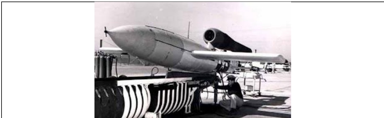
The Republic-Ford JB-2 differed from the V-1 in minor details (USAF/Wikipedia)
