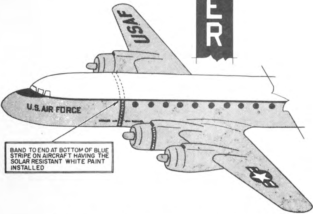
Figure E-10. Propeller Warning Stripes and Signs
