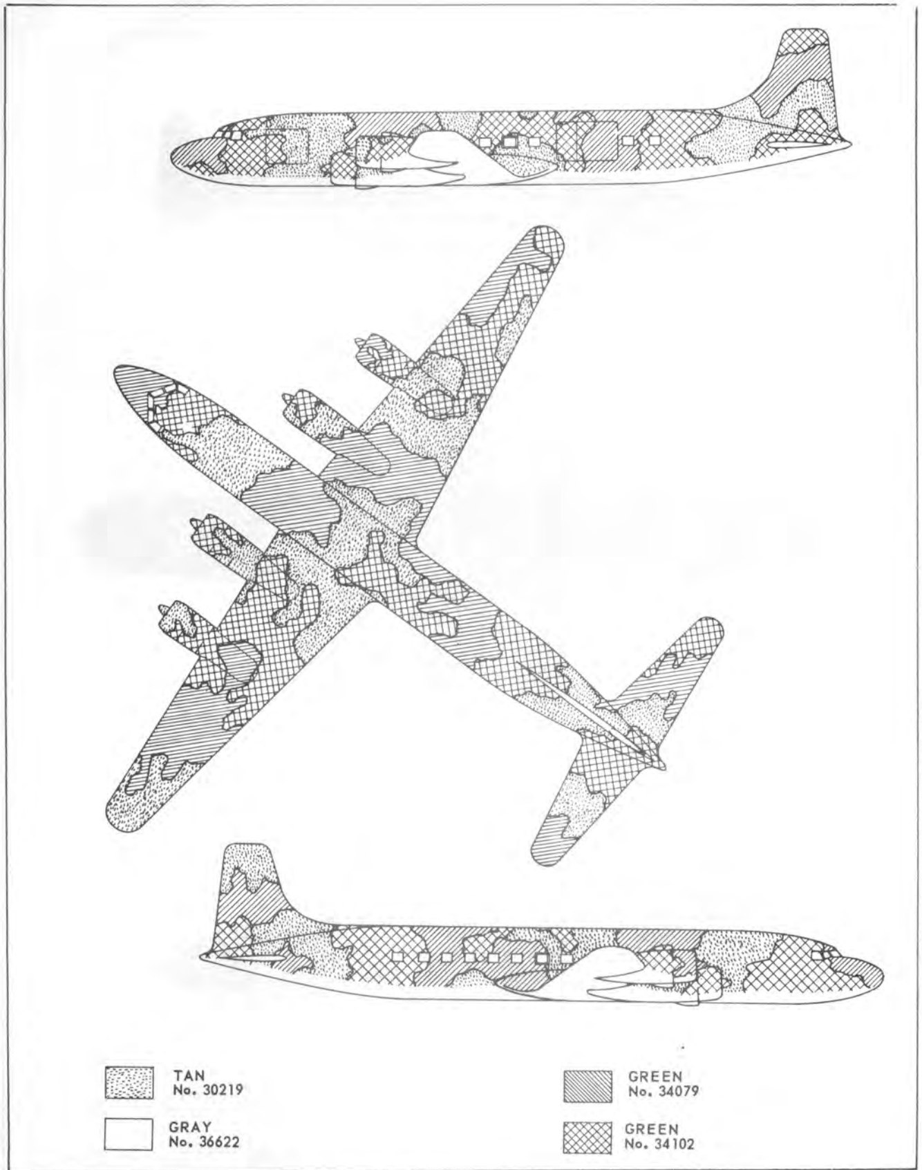
Figure D-13. C-118 Aircraft Camouflage Pattern
