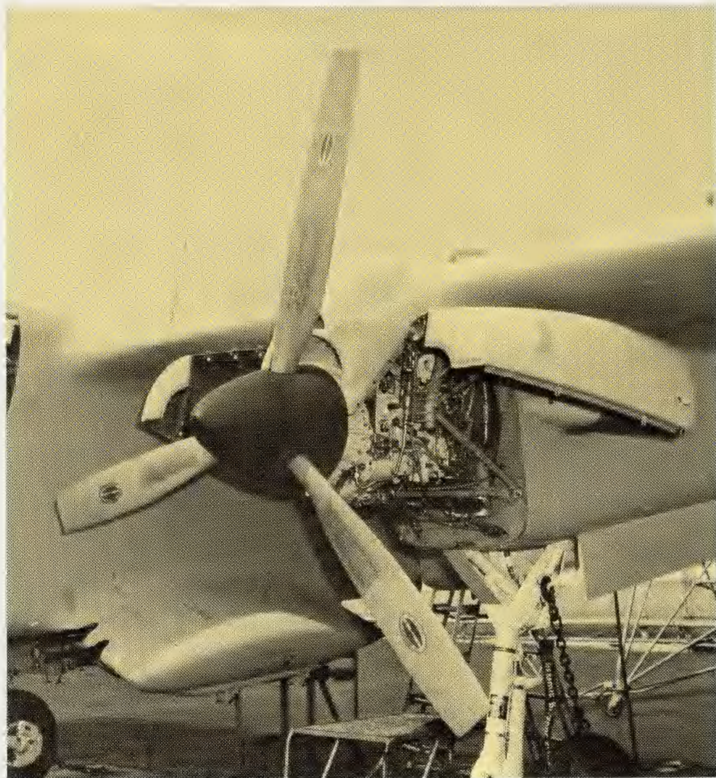
SWING-OPEN COWLING PROVIDES ACCESS TO ENGINE COMPONENTS
