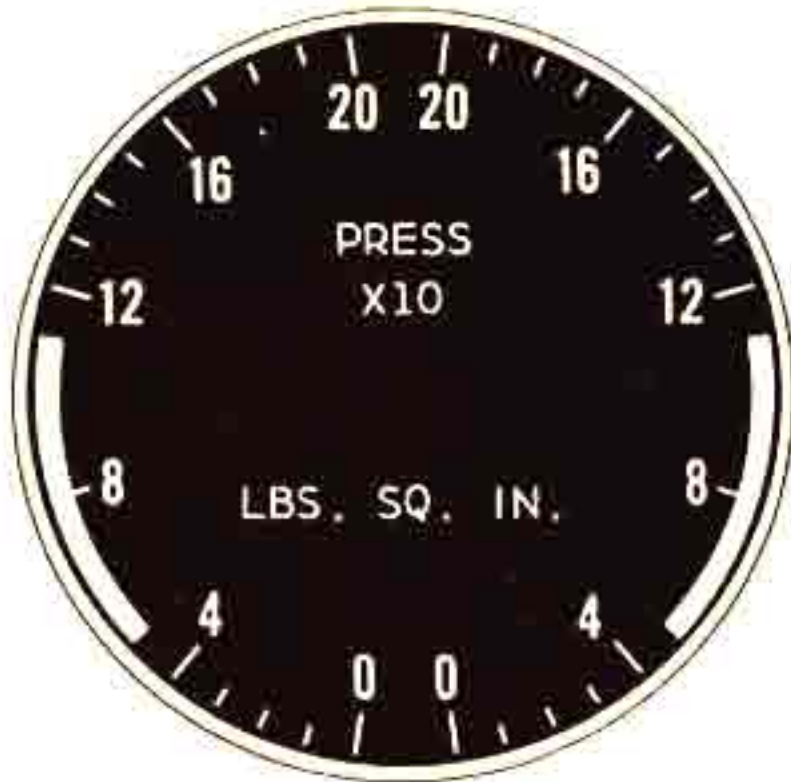
OIL PRESSURE □ 50 To 110 PSI Operating Range
