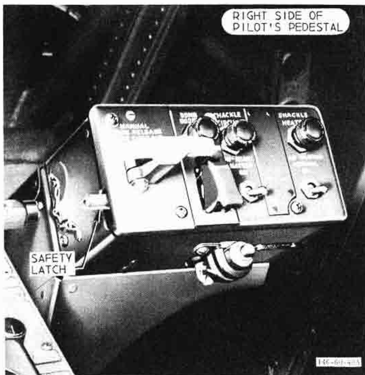
Figure 4-3. Master Bomb Control Panel
