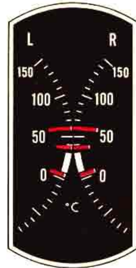
CARBURETOR AIR TEMPERATURE ■ 5° C Minimum □ 8° C To 30° C Operating Range ■ 38° C Maximum, Dry ■ 60° C Maximum, Wet
