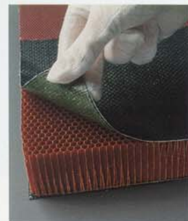
The Starship's extraordinary strong composite structure is essentially a sandwich constructed from sheets of graphite/epoxy on top and bottom over structural adhesive, bonded to a lightweight aramid fiber honeycomb core. In areas where extra strength is needed, additional plies of graphite are layered on.
