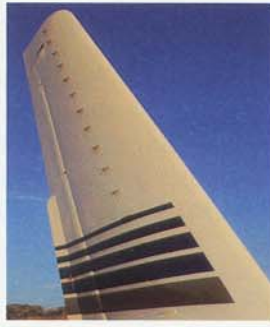
Rows of wedge-shaped vortilons keep the wings and tipsails keep flow attached to the airfoil surfaces during extreme speed/high angle of attack, further improving altitude handling and stability.
