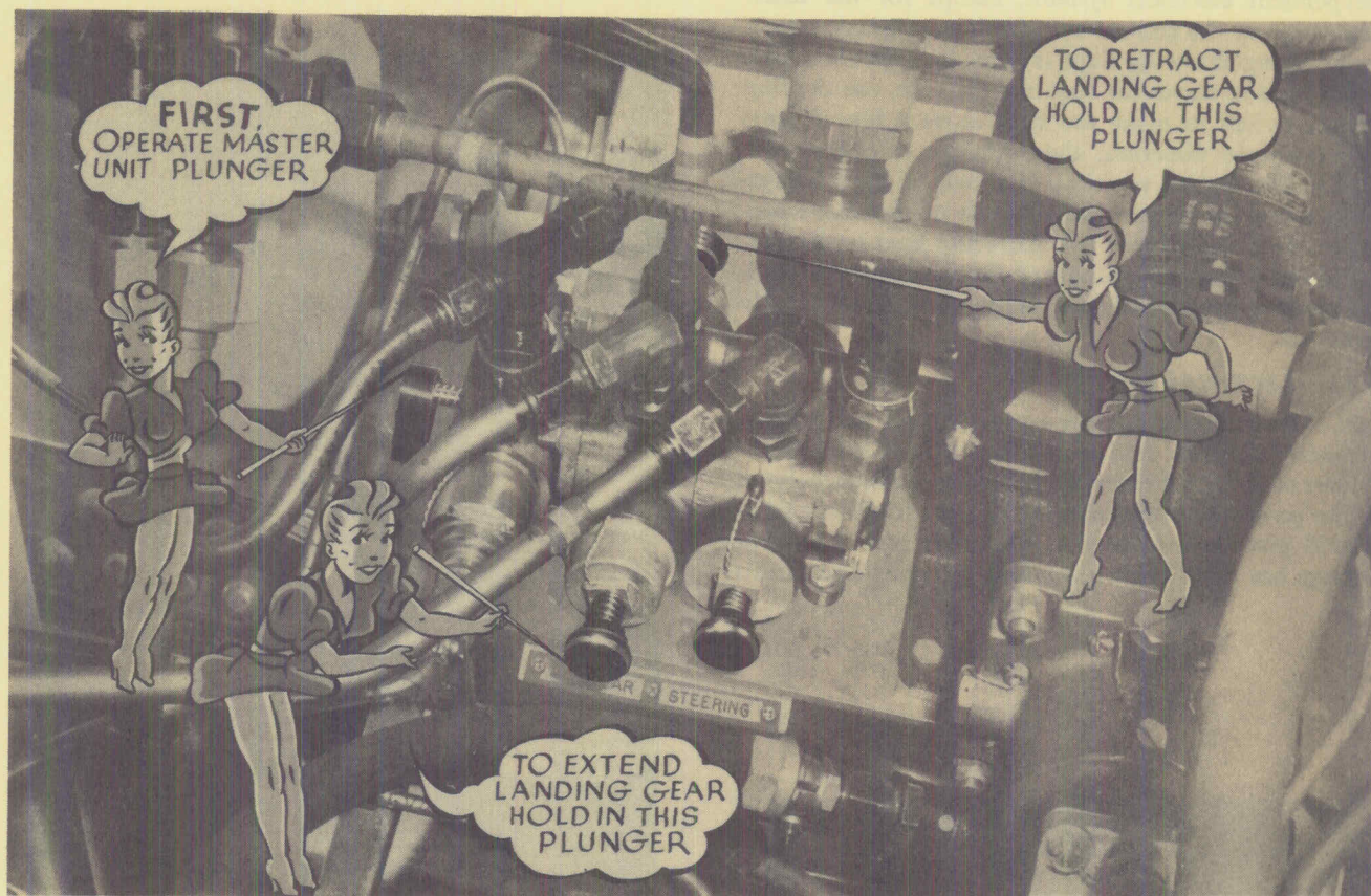
Figure 3-8. Main Selector Valve Manual Controls (In Right Rear of No. 2 Bomb Bay)
