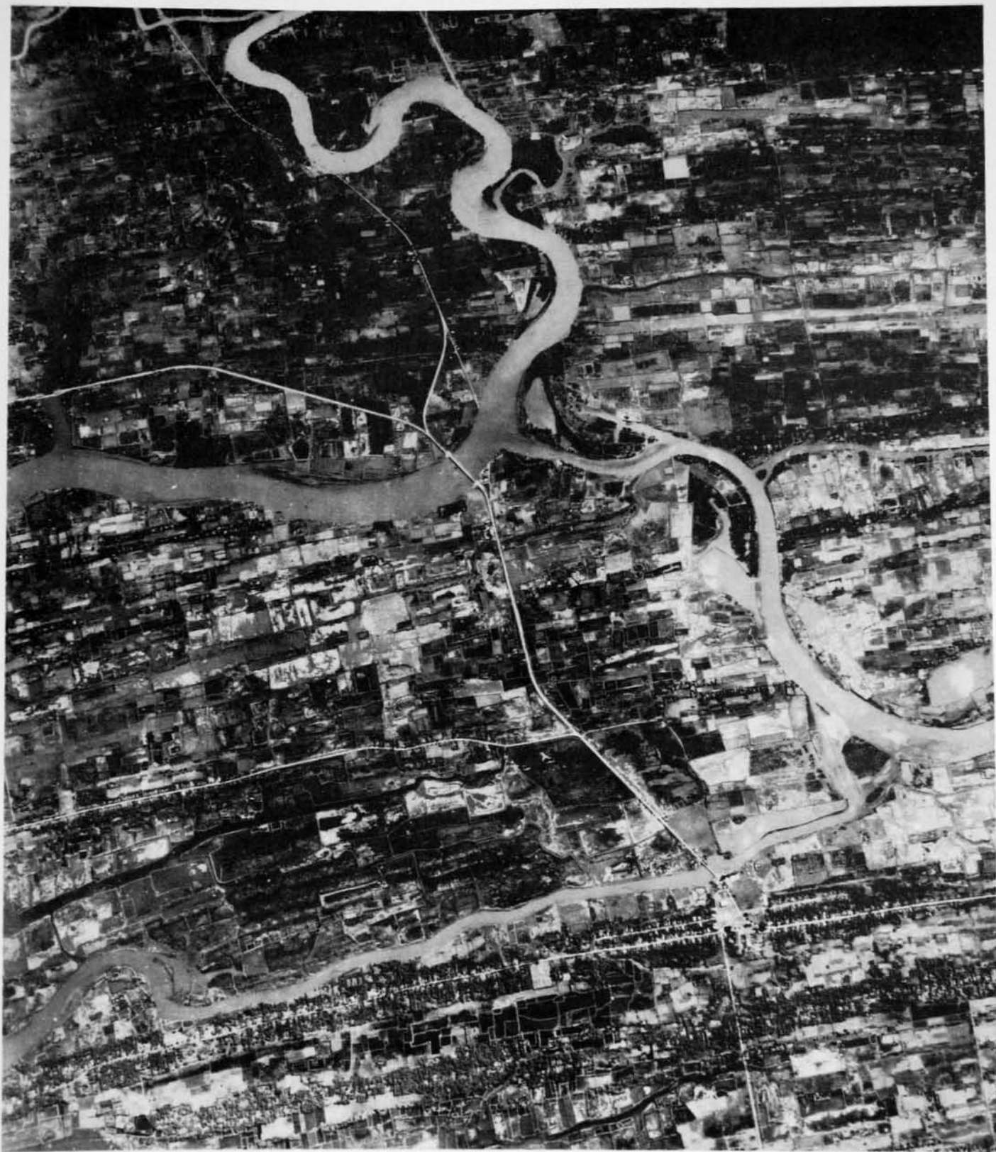
STREAM JUNCTION shown by these old meandering rivers plus highway bridge and ford alongside are typical check points that can be used where there is an old stage of erosion.
