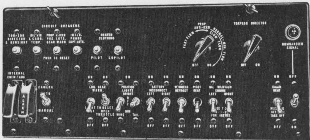
Figure 20—Pilot's Switch Panel
