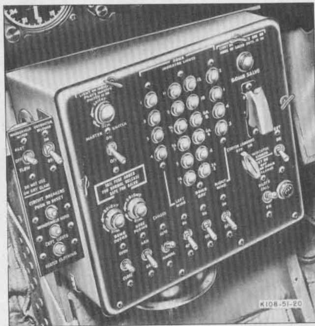
Figure 47—Bombardier's Control Panel—Late Airplanes
