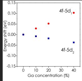
A progressive shift of 4f-5d Ce transitions was evidenced by optical absorption measurements.
