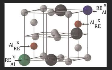
Atomistic simulations showed that the addition of Ga to  $RE_3Al_5O_{12}$  garnets generally lowers the cation antisite defect formation energy, thus suggesting that **Ga additions** should lead to a **higher concentration** of **antisite defects**
