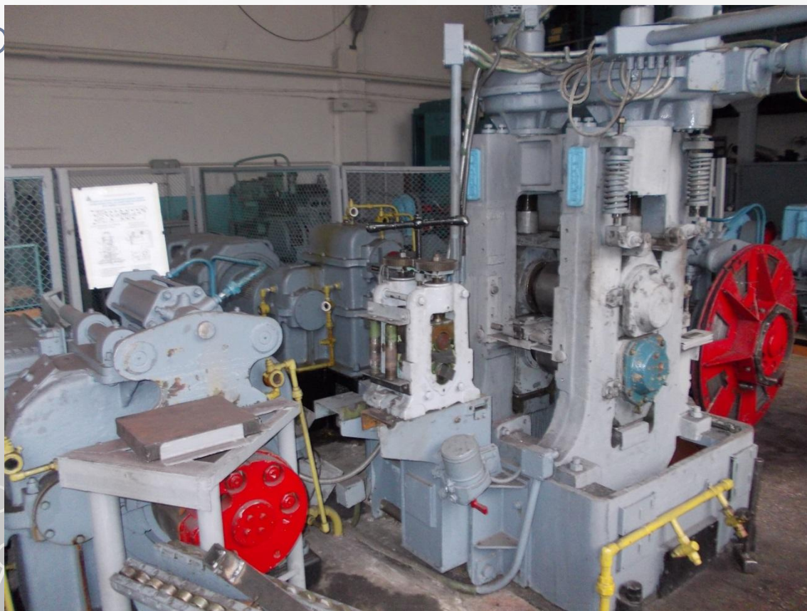
Rolling blanks from BT1-0 on the mill 200 (DSEA) with temperature control
