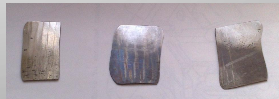
Samples after rolling along to H = 2.2 mm and across H=1,5...1,2 mm, B=26...33 mm, L=52 mm
