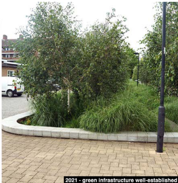
Concrete block permeable paving in conjunction with green infrastructure transforms Bridget Joyce Square, London.
