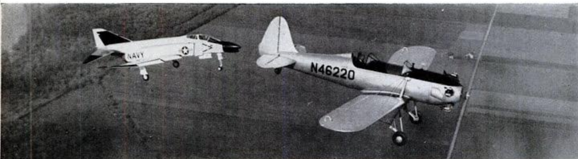
F4H demonstrates its remarkable low-speed ability by flying in formation with a Ryan PT-22, WW II primary trainer. Phantom easily maintained 118 kts.
