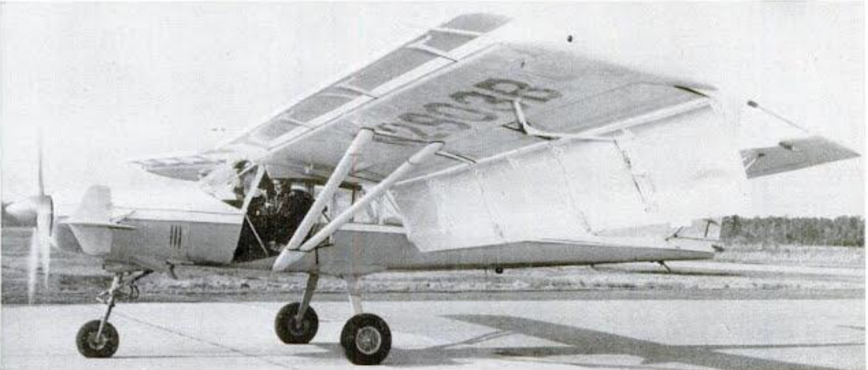
Low-speed flight is achieved by use of slotted leading edge combined with full-span wing flaps in the 4,200-pound gross weight aircraft.
