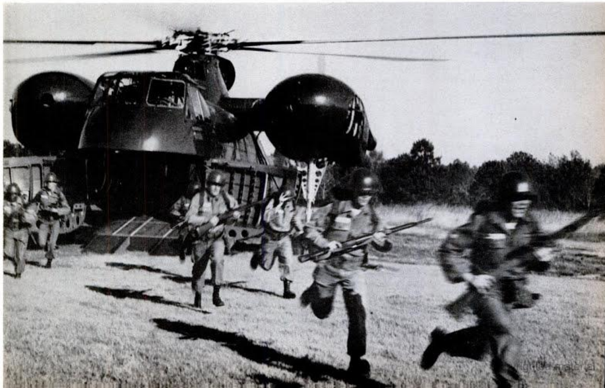
Twin-engine Sikorsky H-37 Mojave carries up to 23 troops on combat missions. Alternate load: 24 litters. Top cruise speed loaded is 80 knots.
