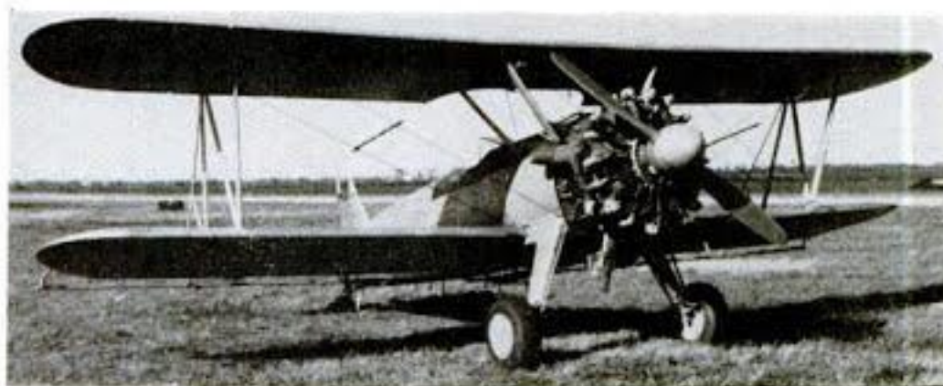
POWERFUL DUSTER (Right). Boeing-Stearman PT-13 powered by a 650-hp Pratt & Whitney R1340 engine has near helicopter performance at takeoff, stalls at 50 mph IAS with full load. Used for agricultural work, it doubles the swath speed of same craft with 450-hp engine. Conversion was made by Sequin Aviation, Sequin, Tex. for approximately $2,000 including surplus engine and propeller. Engine mount was shortened and the oil tank relocated behind the rear cockpit.
