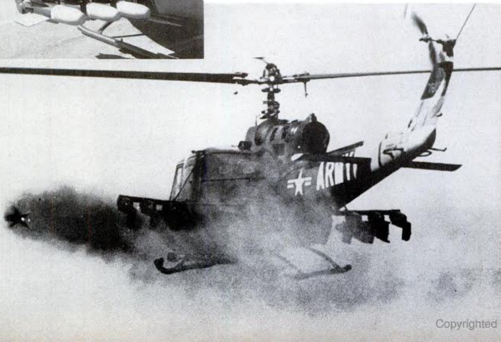
Below: Turbine-powered Bell HU-1 fires Nord SS-11 guided wire anti-tank missile. Left: Three are mounted in racks on each side of rotorcraft.
