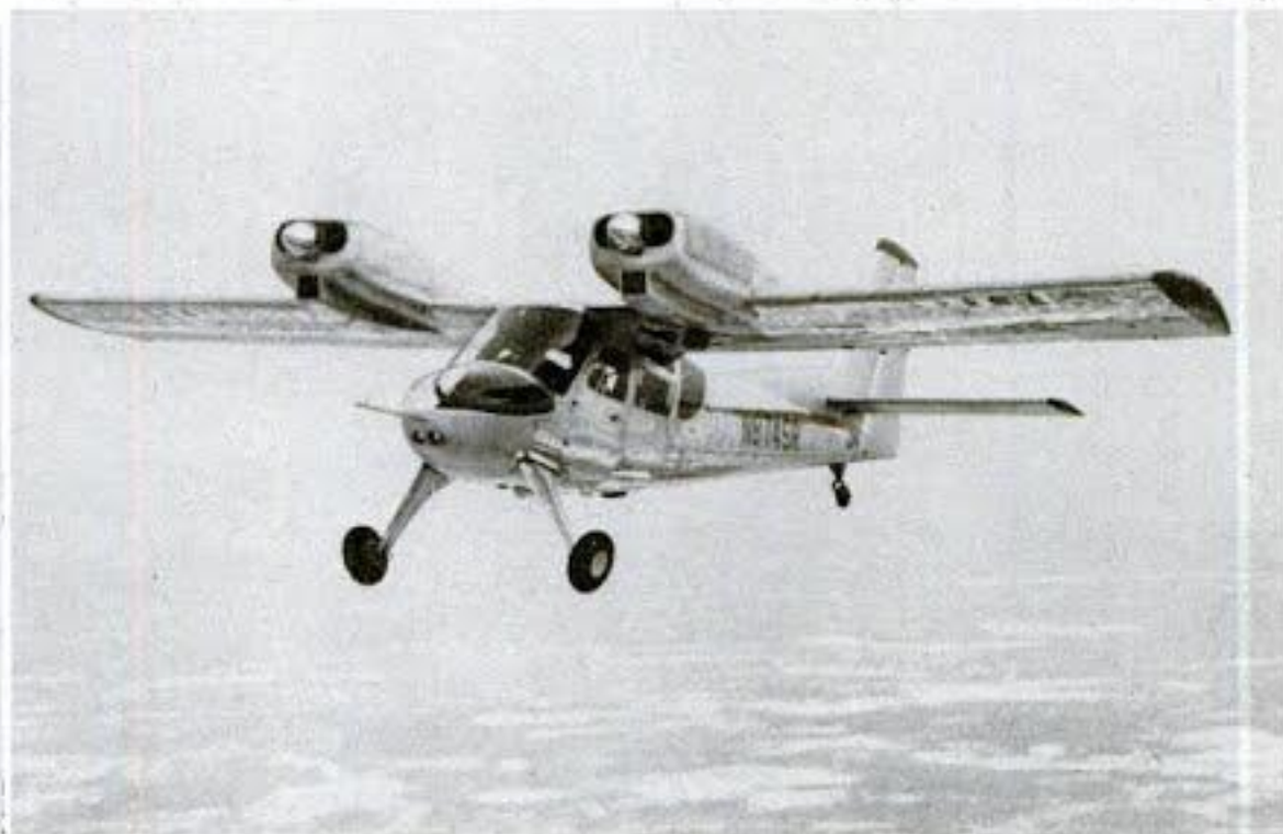
HELIO 500 (Above). Twin-engine STOL aircraft designed and built by Helio Aircraft Corp., Norwood, Mass. utilizes same high lift devices as the single-engine Helio Courier. Aircraft is powered by two Lycoming O540 engines of 250 hp each. Takeoff distance over 50-foot obstacle, 530 feet. Landing distance over 50-foot obstacle, 665 feet. Maximum speed 181 mph., minimum speed is 36 mph. Note overhead throttles in photo of cockpit.
