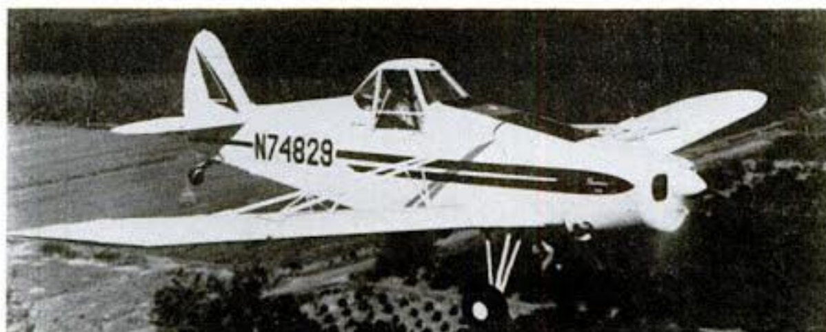
POWERFUL DUSTER (Right). Boeing-Stearman PT-13 powered by a 650-hp Pratt & Whitney R1340 engine has near helicopter performance at takeoff, stalls at 50 mph IAS with full load. Used for agricultural work, it doubles the swath speed of same craft with 450-hp engine. Conversion was made by Sequin Aviation, Sequin, Tex. for approximately $2,000 including surplus engine and propeller. Engine mount was shortened and the oil tank relocated behind the rear cockpit.
