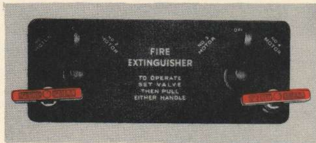
Figure 37—Engine Fire Extinguisher System Controls
