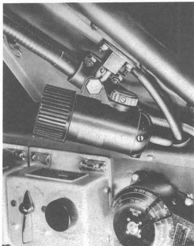
Figure 270 — Cockpit Light Installed
