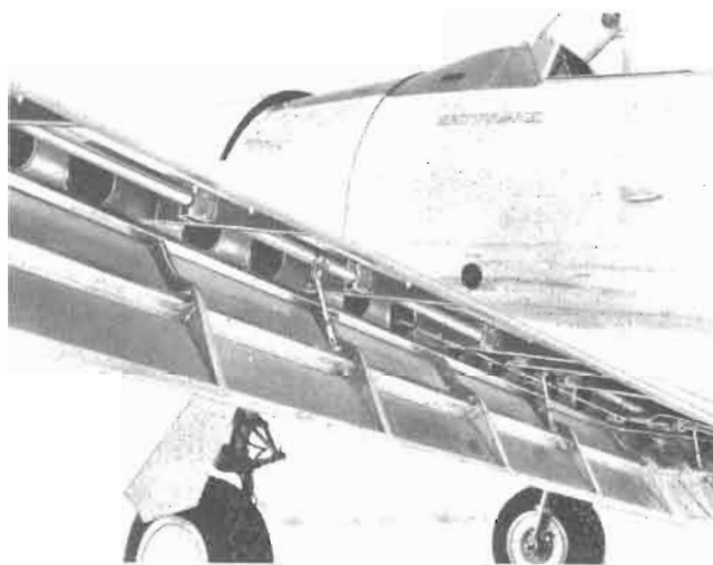
Figure 71 — Wing Flaps Installed
