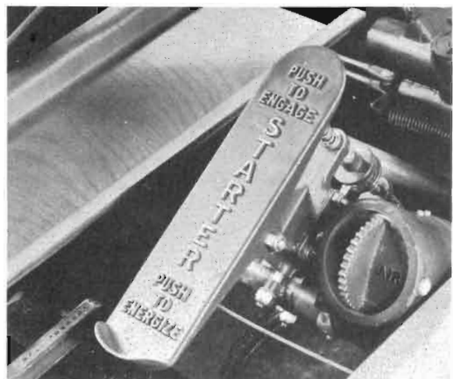
Figure 266 — Starter Foot Pedal Installed
