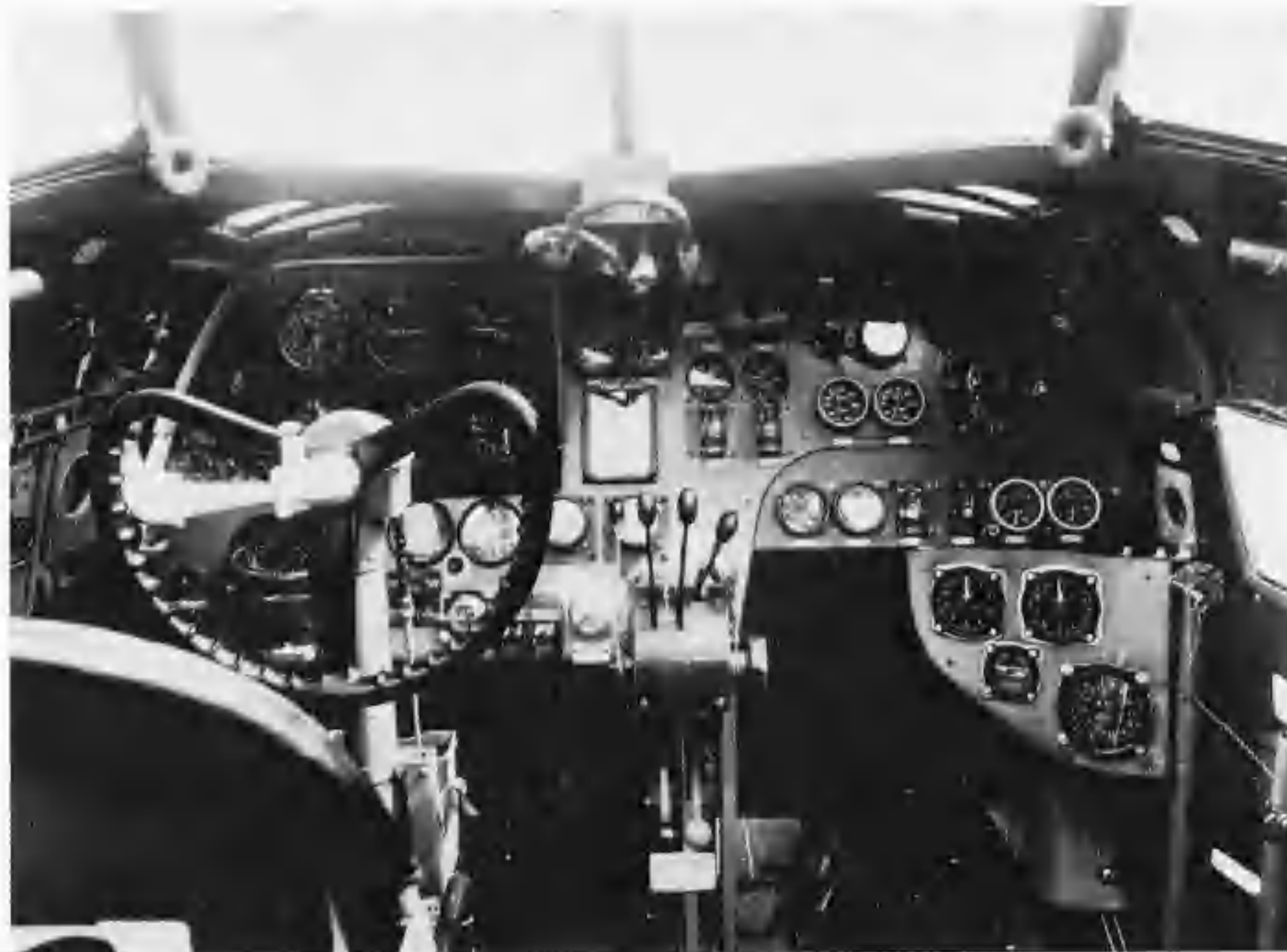
The cockpit of a Whitley Mk V used as a glider tug is shown in this photo. The crawlway to the bomb-aiming position in the nose has been partially blanked-off, as it was no longer needed in this aircraft.
