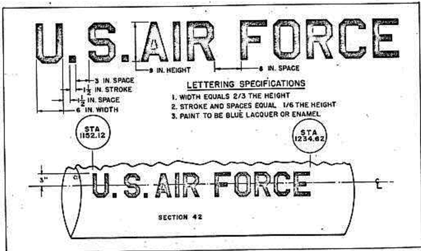
Figure 3-60. Location of Missile Markings CIM-10A.
