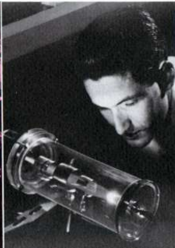
Ion accelerator used by NASA scientist
