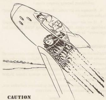
Air starts using rpm greater than 25% will probably result in excessive and damaging exhaust temperatures.
