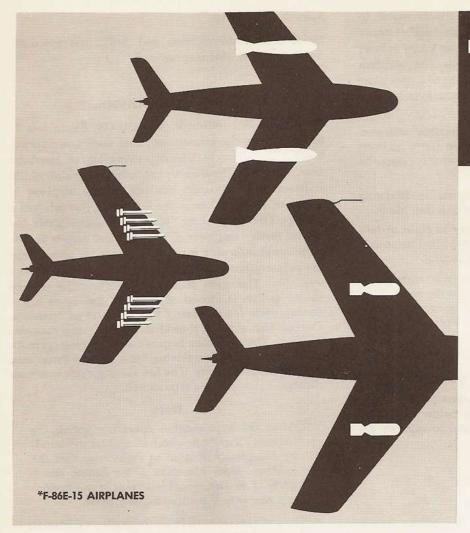
possible armament and drop tank installation
