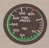
(Fuel pressure gage with expanded scale)
