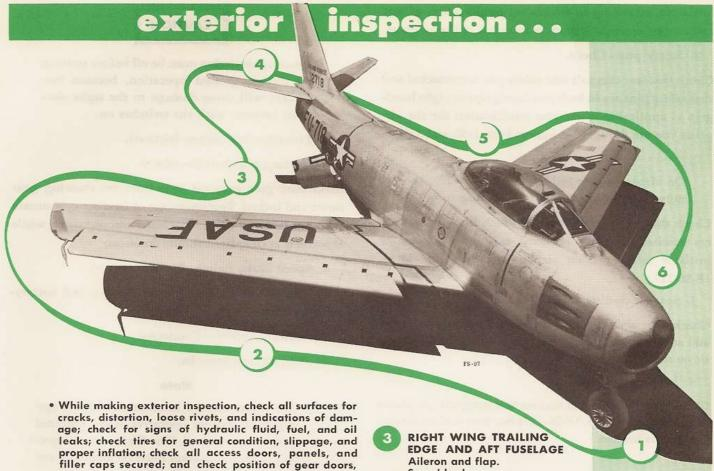
gear strut extension, and condition of wheels. Accumulator gage pressures (given on placard next to gage) are for 70°F; pressure will be higher on hotter days.
