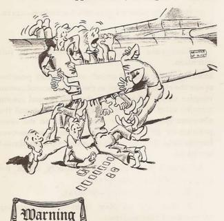
Before operating speed brakes, be sure aft fuselage area is clear, as the speed brakes move rapidly and forcefully and could injure any personnel in their path.
