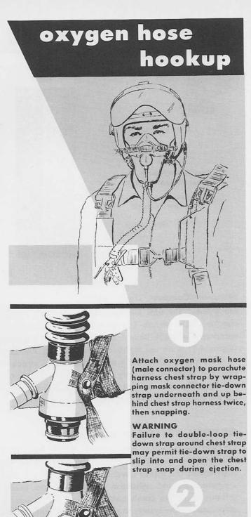
Attach seat oxygen hose to oxygen mask hose. Listen for click and visually check (or feel) that sealing gasket is only half exposed.
