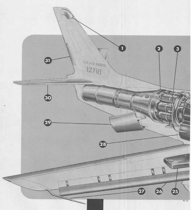
Command Radio Antenna J47-GE-13 Engine
