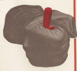
SQUEEZE TRIGGER TO EJECT SEAT.
