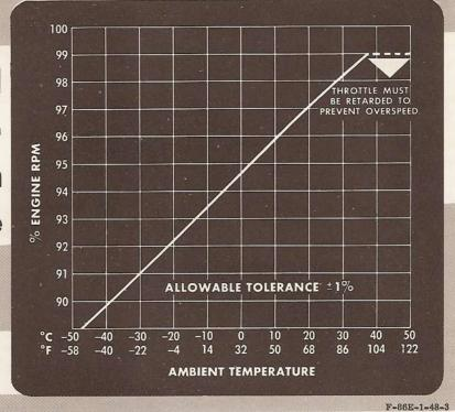
Chart shows variation (due to temperature change) in engine rpm when operating on emergency fuel system with throttle in full **OPEN** position.
