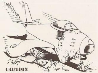
If a hard landing is made while external loads are carried, the airplane should be inspected prior to the next flight for signs of structural damage.
