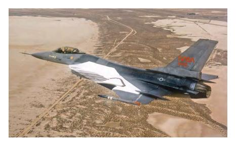
F-16XL-1 with the active suction glove on the left wing that was used for research into supersonic laminar flow control. The grey titanium active suction panel is visible on the inner region of the white wing glove. The passive outer leading edge of the wing glove is painted black in the region where a liquid-crystal sensor array was located. A video camera in the wingtip pod was used to record the liquid-crystal patterns. (NASA)
