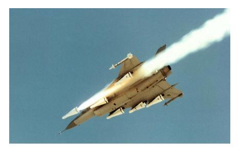
An unguided AGM-65 Maverick missile was launched from F-16XL-1 store station 3 on March 29, 1985. Weapons carried on this flight included four dummy AIM-120s, two AIM-9Ls, and six AGM-65 missiles. (USAF)
