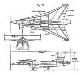
This SCAMP concept featured an all-moving vertical tail and full-span leading-edge flaps on both the inboard and outboard wing segments of its highly swept crankedarrow wing. (Lockheed Martin)
