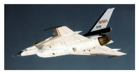
The F-16XL-2 in flight showing its Langley-tested shock wave fence under the port wing. (NASA)
