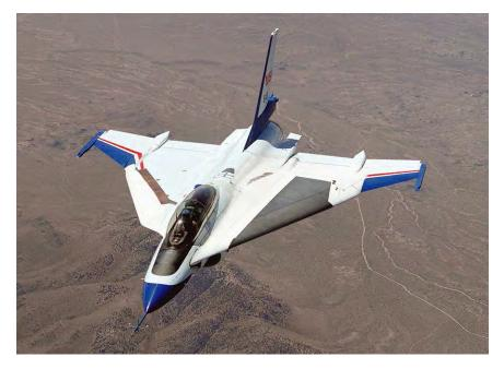
F-16XL-2 flying with a supersonic laminar flow control suction glove leading edge, April 1996. (NASA)
