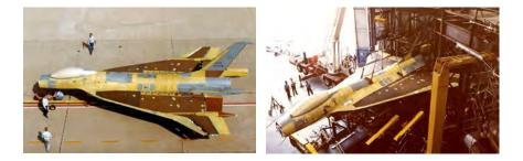
On left: The first F-16XL, 75-0749, is seen in April 1982 after its removal from its assembly fixture. The composite wing skins and wing-fuselage mounting bolt locations are evident. On right: The F-16XL-1 is seen being prepared for static structural proof testing in the spring of 1982. (Both images Lockheed Martin)
