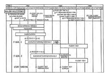
The F-16XL flight demonstrator design, fabrication, assembly, and flight-test program schedule, as depicted on a GD chart circa 1980. (Lockheed Martin)
