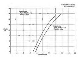
Flight envelope restrictions and maneuver limits were imposed on F-16XL-1 during the DFCS evaluation. (NASA)
