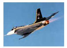
F-16XL-1 was used in its basic unmodified aerodynamic configuration for the CAWAP flight-test effort. (NASA)
