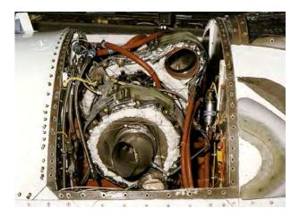
The engine bleed air–powered turbocompressor used with the active SLFC suction system was installed in F-16XL-2's ammunition bay, formerly used to house the 20-mm rounds used by its M61 Vulcan cannon. The overboard flow vent that exited on the upper right side of the aircraft is in the foreground. (NASA)
