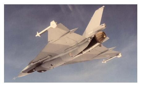
The F-16XL-2 had a fake "canopy" and air refueling receptacle markings painted on its underside to visually disorient opposing fighter pilots as to the true orientation of the aircraft. The circular white markings were intended to represent pilots' helmets when seen from a distance. (USAF)
