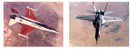
On left: General Dynamics YF-16 prototype over the Mojave during the Lightweight Fighter (LWF) competitive fly-off. On right: The Northrop YF-17, which, despite losing the LWF competition, evolved into the subsequent F/A-18 naval strike fighter. (Both images USAF)
