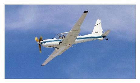
A NASA Lockheed YO-3A was used to measure the sonic boom signatures emanating from a Lockheed SR-71 flying at supersonic speed at much higher altitudes. (NASA)
