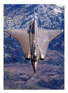
A two-place Saab Sk 35C Draken trainer of the National Test Pilot School cruising over the Sierra Nevada range on a training flight from Mojave Air and Space Port, Mojave, CA. Its "cranked-arrow" double-delta wing is readily apparent; the configuration anticipated by over a quarter century the cranked-arrow planform of the General Dynamics F-16XL. (National Test Pilot School photograph, courtesy Gregory V. Lewis and Russ Stewart)
