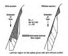
F-16XL-1 with an active suction glove installed on the left wing demonstrated limited laminar flow at supersonic conditions during flight testing conducted in 1991–1992. (NASA)
