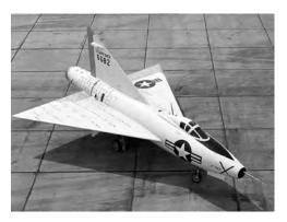
The Convair XF-92A Dart, progenitor of all American delta-wing aircraft, on the ramp of the NACA High-Speed Flight Research Station (now the Dryden Flight Research Center) in 1953. The wing and aft fuselage were tufted for flow visualization studies. Despite its "F" for "Fighter" designation, this was strictly a transonic research aircraft. (NASA)
