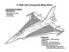
Composite wing skins increased structural strength, saved weight, reduced manufacturing cost, and improved durability. (Lockheed Martin)
