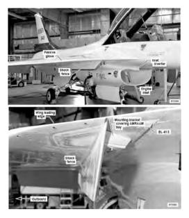
Initially, the F-16XL-2 had a 10-inch-tall shock wave fence under its starboard wing, as seen above. (NASA)
