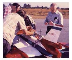
A radio-controlled 0.18-scale drop model is prepared for release from a NASA Bell HU-1 helicopter at the Plum Tree Island test facility in 1983. (NASA)
