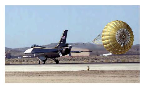
F-16XL-1 is seen during landing rollout with its drag chute deployed and the speed brakes on either side of the engine nozzle in the open position. (NASA)
