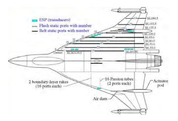
An extensive suite of pressure instrumentation systems was installed on F-16XL-1 during the CAWAP test effort. (NASA)
