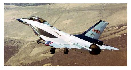
Research pilot Dana Purifoy flew the highly modified F-16XL-2 on its first flight with the asymmetrical wing configuration on October 13, 1995. Wingtip-mounted flutter excitation vanes are fitted on both wingtip missile launchers. (NASA)
