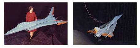
On left: NASA Langley's Sue Grafton is shown with the 0.18-scale captive free-flight wind tunnel model used to validate F-16XL aerodynamic and flight control modifications. On right: the 0.18-scale F-16XL model is seen during free-flight testing in the NASA Langley Full-Scale Tunnel. (Both images NASA)
