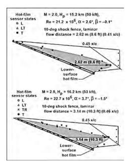
The maximum extent of supersonic laminar flow on the F-16XL-2 active suction wing glove was achieved at Mach 2.0 at an altitude of 53,000 feet. (NASA)
