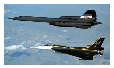
F-16XL-1 was used for sonic boom probing tests with the NASA SR-71. The F-16XL's speed brakes are extended in this photo taken at subsonic speed; however, the F-16XL had a difficult time maintaining formation with the SR-71 above Mach 1.5. (NASA)
