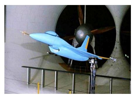
A 0.18-scale instrumented F-16XL model was tested in the NASA Langley 30- by 60-foot Full-Scale Tunnel to obtain precise vortical data for comparison with airflow results predicted from CFD modeling. (NASA)
