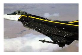
The F-16XL-1 was heavily instrumented for the CAWAP research program. The aircraft is seen during a datacollection run at an angle of attack of 21 degrees at an altitude of 17,500 feet. The surface tufts, pressure belts, and visual reference markings are readily discernible. (NASA)
