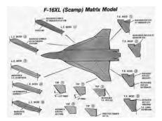
The matrix model could be rapidly modified using a variety of removable leading edges, wingtips, and trailing edges to efficiently assess their effects on aerodynamic characteristics. (Lockheed Martin)
