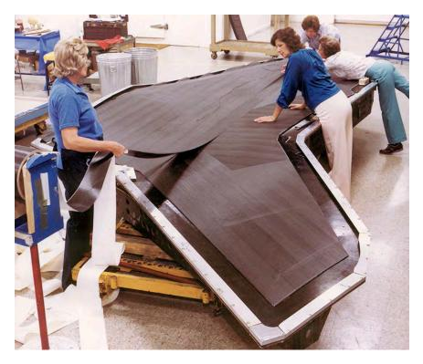
Graphite-bismaleimide laminates were used in various combinations and orientations to build up the composite wing skins. (Lockheed Martin)
