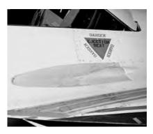
A faired gun trough fairing was added to F-16XL-2 to minimize shock wave influences on the laminar flow wing glove. (NASA)
