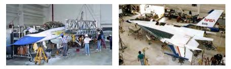
On left: The laminar flow wing glove during the positioning process on F-16XL-2's left wing, February 1995. On right: The F-16XL-2 after the laminar flow wing glove was mounted on the wing and the forward wing fairing was installed. Note how far forward on the fuselage the left wing extended. (Both images NASA)
