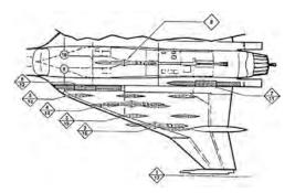
A complex hard-point arrangement was developed for the F-16XL to enable external stores to be mounted in dense conformal arrangements. (Lockheed Martin)
