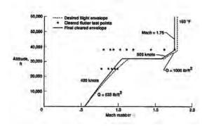
The F-16XL-1 flutter envelope approved for use during the SLFC research program. The vertical axis shows aircraft altitude in thousands of feet. (NASA)
