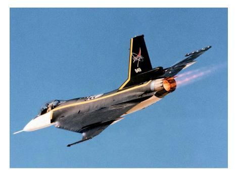
$\ensuremath{\mathsf{F-16XL-1}}$  was used in its basic unmodified aerodynamic configuration for the CAWAP flight-test effort. (NASA)
