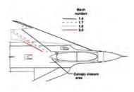
The canopy-closure shock wave impingement locations on the upper surface of F-16XL-2 are illustrated for several representative cruise Mach numbers. (NASA)
