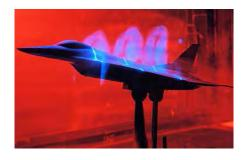
A 1/25-scale F-16XL-1 model was tested in the Basic Aerodynamics Research Tunnel at NASA Langley Research Center in 1992. Laser light sheets illuminate the vortex flow field around the model. (NASA)
