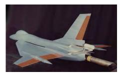
F-16XL model fitted with the "Quadra Pod" spin recovery parachute installation during wind tunnel testing at NASA Langley in May 1982. (NASA)
