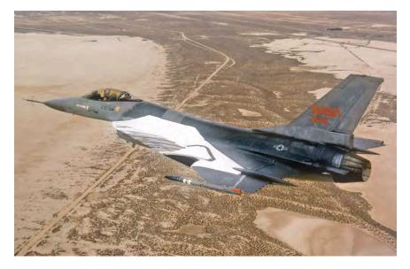
F-16XL-1 with the active suction glove on the left wing that was used for research into supersonic laminar flow control. The grey titanium active suction panel is visible on the inner region of the white wing glove. The passive outer leading edge of the wing glove is painted black in the region where a liquid-crystal sensor array was located. A video camera in the wingtip pod was used to record the liquid-crystal patterns. (NASA)
