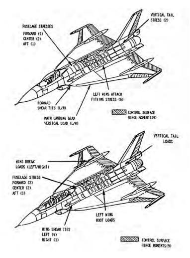
Sensors for determining structural loads on the airframe were positioned at different locations on F-16XL-1 and F-16XL-2 as shown in these GD drawings. (Lockheed Martin)
