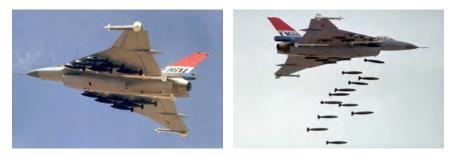
On left: The F-16XL-1 flying a test mission on August 18, 1982, with 12 500-pound Mk-82 bombs, 4 fuselage-mounted AIM-120 AMRAAMs, and 2 wingtip-mounted AIM-9 Sidewinder missiles. On right: On August 24, 1982, the F-16XL-1 successfully released 12 500 pound Mk-82 bombs from individual low-drag ejector bomb racks. (Both images USAF)
