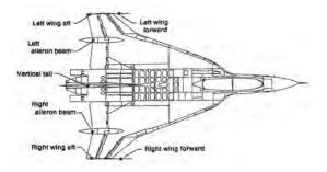
Accelerometer locations on the F-16XL airframe for use in flutter testing. (NASA)
