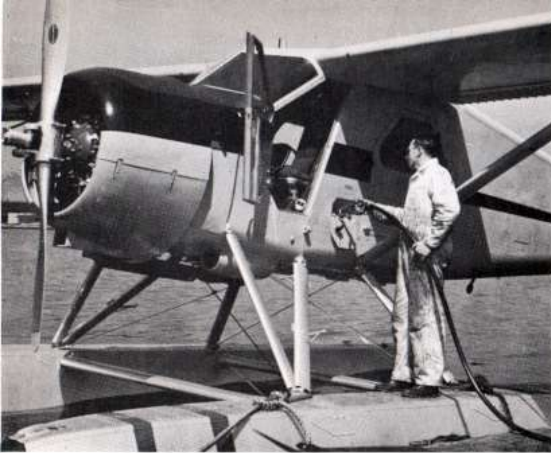
Fuel filler caps are located at ground level—eliminating necessity for climbing up on the wings to re-fuel.
