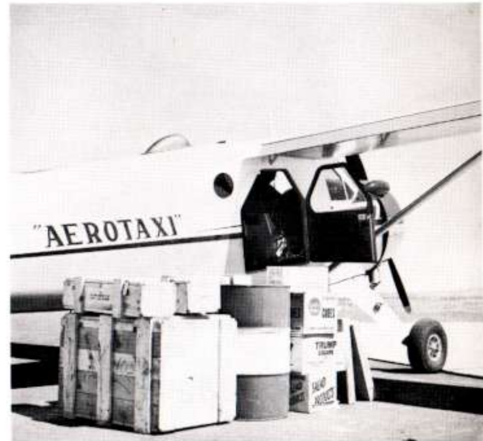
The cabin doors (39 inches wide by 40 inches high) are easily removable and permit 45-gallon gas drums to be rolled in sideways or pushed in upright.
