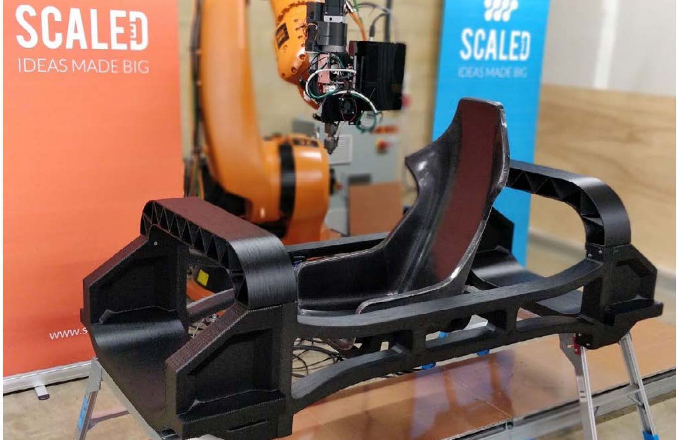
3D printed concept vehicle chassis with carbon fibre seat made from 3D printed tool. In the background, robot 3D printer.
