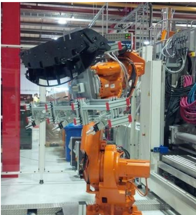
Robotic injection moulding machine tending, and mould tool insert loading for JLR spoilers.
