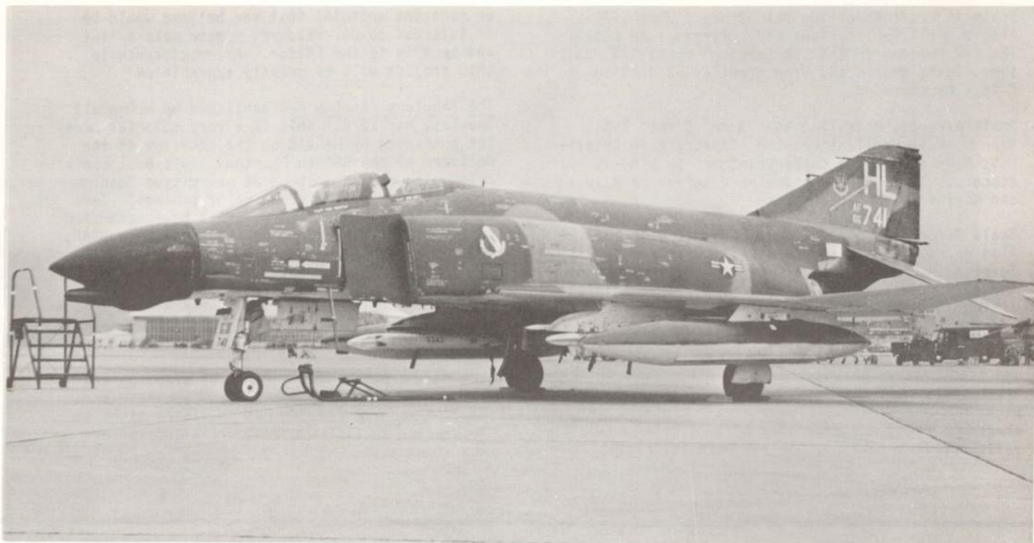
ABOVE: Nice shot of a 34th TFS F-4D taken at Hill AFB. Note placement of the many stencils that were common on the Phantom. Aircraft is painted in standard SEA camouflage scheme. Photo T. Taylor.
