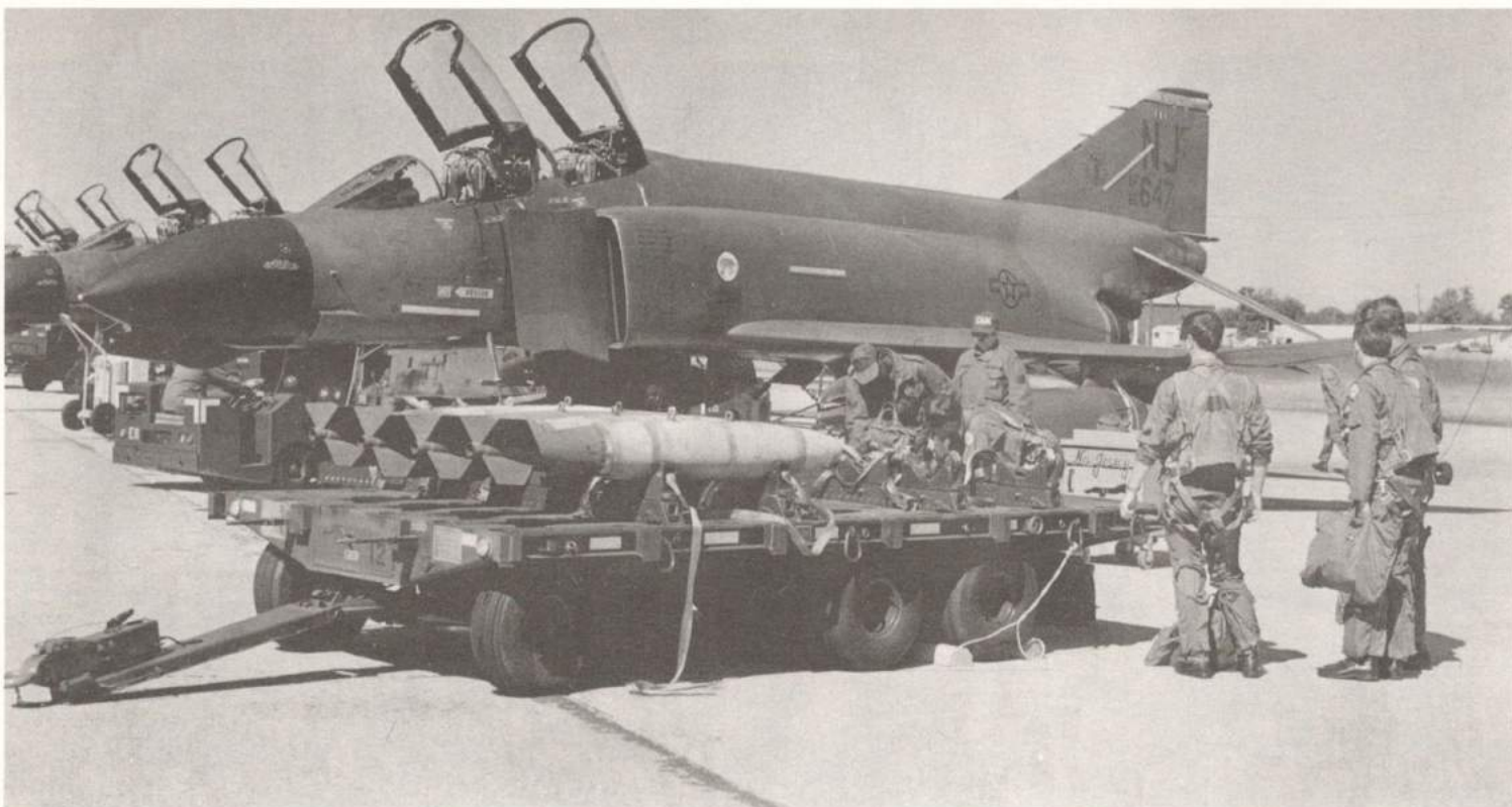
BELOW: Weapons personnel loading Mk.82 bombs on F-4Ds of the 108th TFW. Aircraft were participating in a surge and were loaded with weapons and fuel and were airborne again in 30-40 minutes. Photo by Don Sperring/A.I.R.
