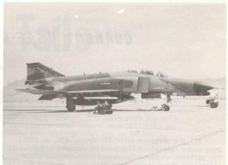
F-4G-45-MC 69-7582. 81 TFS 52 TFW based at Spangdahlem AB, Germany. This aircraft was taking part in Red Flag at Nellis AFB, NV in June 1983. Canopy frame is black edged in yellow. The fin tip is yellow. Note the F-15 centerline tank which is carried by the Gs. These tanks can take more G forces than the standard F-4 tanks. Photo J. Geer.
