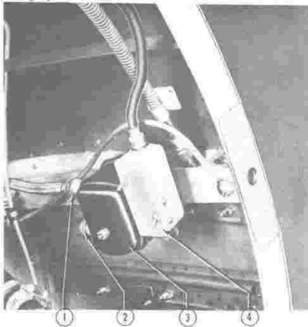
1. Electrical Connection to Magneto 3. Induction Vibrator 2. Alternate Electrical Connection 4. Radio Noise Filter
