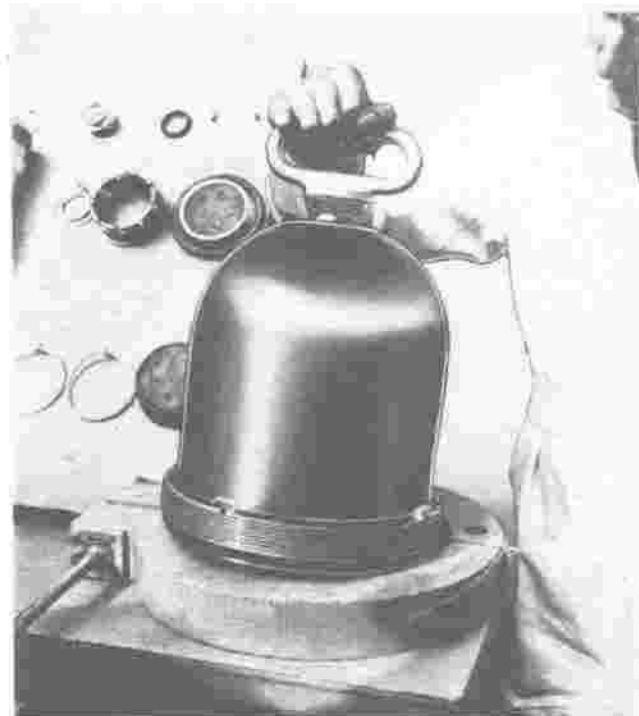
Figure 191—Installing Dome Lifting Handle in Breather Hole
