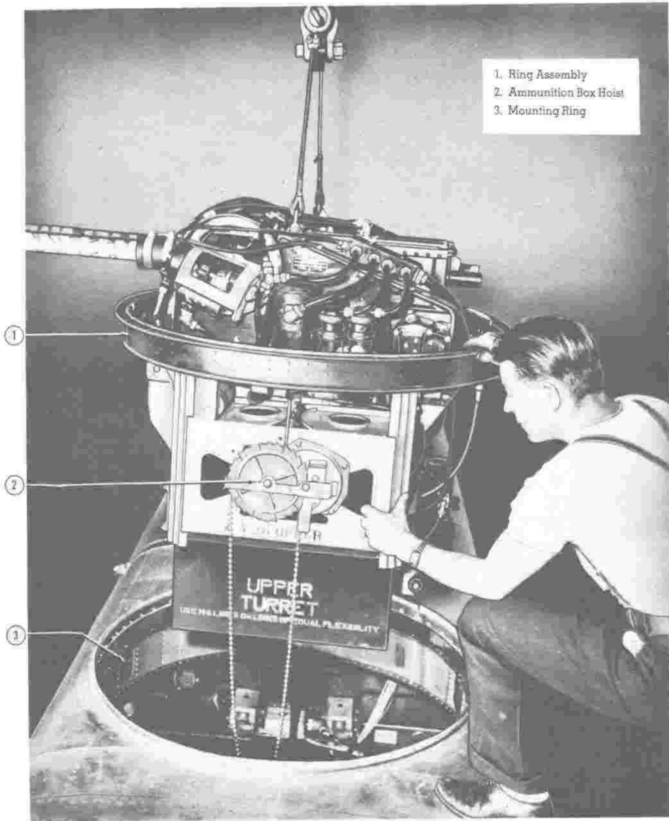
Figure 388 — Hoisting Upper Turret For Installation
