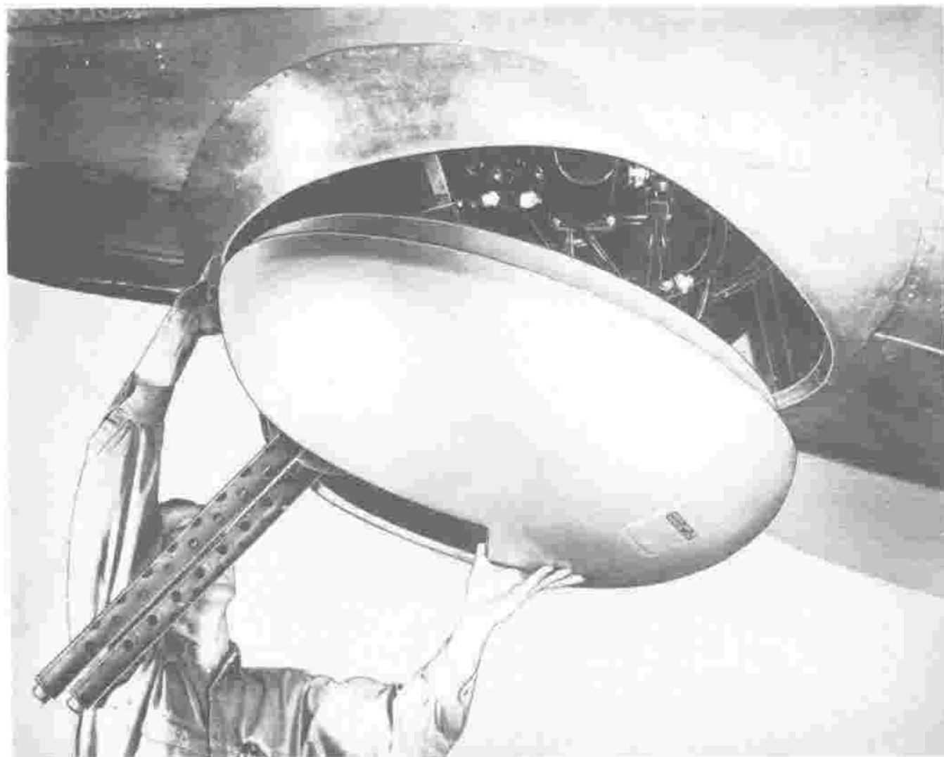
Figure 417 — Dome Removal (Lower Turret)
