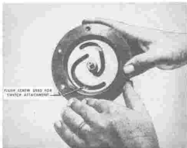
Installation of Cam in Body
