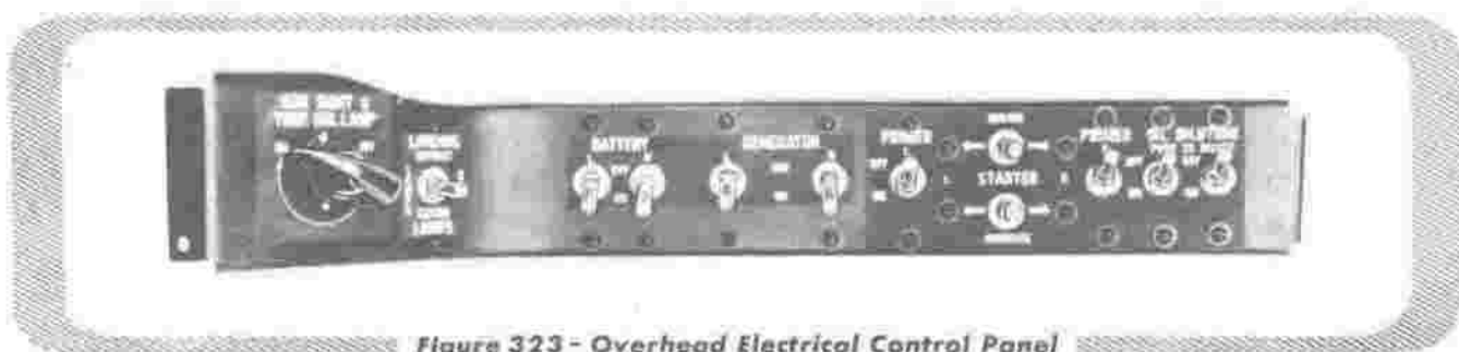
Figure 323 - Overhead Electrical Control Panel
