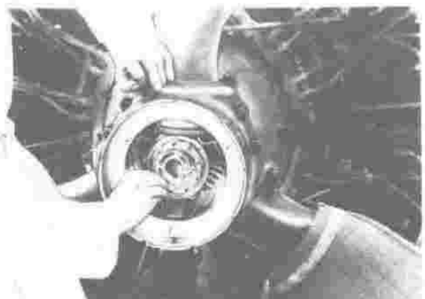
Figure 187—Installation of Oil Transfer Plate and Shaft Oil Seal Gasket—Engine Furnished Parts Previously Installed
