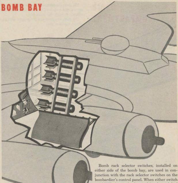
The bomb bay is aft of the pilot's compartment. Provision is made for releasable gasoline tanks in place of a bomb load. One tank may be carried on each side of the bomb truss. Tanks (or bombs) can be released electrically by the bombardier, or can be released by pulling one of the emergency release handles.
