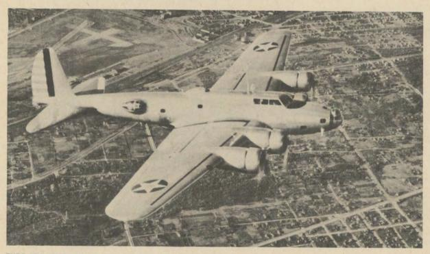
THE B-17A WENT HIGHER: Equipped with turbos, it topped all previous service ceilings, gave maximum performance above 30,000 ft. To range, speed, bomb load, firepower, the B-17 added another advantage: altitude operation.
