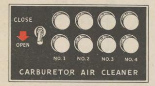
Carburetor air filters must be "ON" ("OPEN") for engine starting and all operations up to 8,000 feet in the B-17F (15,000 feet in the B-17G). Check amber warning light for "ON."
