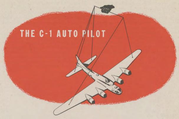
The C-1 autopilot is an electromechanical robot which automatically controls the airplane in straight and level flight, or maneuvers the airplane in response to the fingertip control of the human pilot or bombardier.
