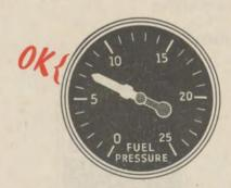
Turn on the booster pumps and check to see that each gives from 6 to 8 lb. pressure. The fuel booster pump is an independent electrically driven source of extra fuel pressure. It takes the place of the wobble pump for both starting and emergencies, and augments the engine-driven fuel pump at high altitudes. As a safety measure, it is always turned on for takeoff and landing, for flights below 1000 feet, and for flights above 10,000 feet.
