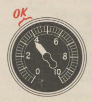
When an engine that operates a vacuum pump (No. 2 and No. 3 Engines) is started, check the rapid response of the flight indicator. With vacuum pump operating, the flight indicator should erect itself within a few moments. Sluggish response at this time indicates poor operation of the instrument. At the same time check (1) vacuum pressure — approximately 3.75" to 4.25"; and (2) both pumps for proper operation.
