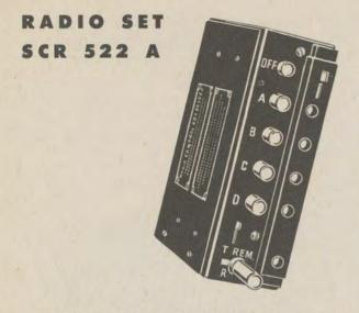
The SCR 522 A VHF (very high frequency) transmitter-receiver radio set provides 2-way radio-telephone communication between aircraft in flight and between aircraft and ground stations. Provision is made for voice communication and continuous audio-tone modulation.
