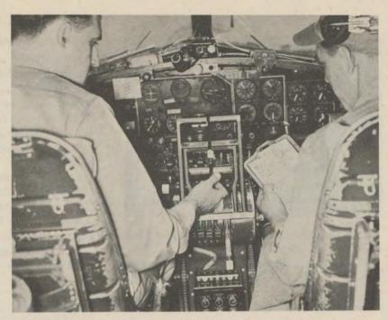
Every B-17 has a checklist on the copilot's side of the cockpit. Individual sections of the cockpit checklist are described at length in the chapters that follow.
