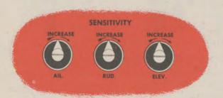
Sensitivity is comparable to a human pilot's reaction time. With sensitivity set high, the autopilot responds quickly to apply a correction for even the slightest deviation. If sensitivity is set low, flight deviations must be relatively large before the autopilot will apply its corrective action.
