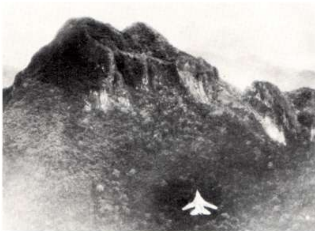
An F-111A, using its terrain-following radar, flies a roller-coaster pattern during a daylight training mission in Thailand. Most actual missions were at night, in weather, and at 200 feet through this kind of landscape.
