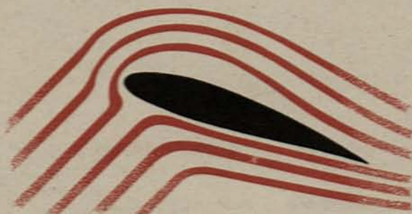
1. Wing close to stalling angle of attack
