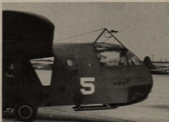
Emergency doors on both sides.
