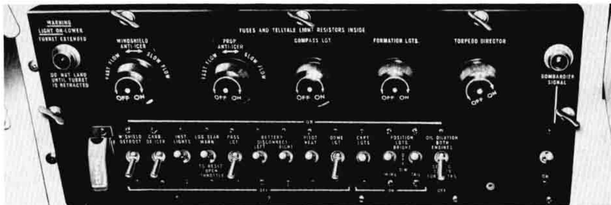
Figure 16—Pilot's Switch Panel
