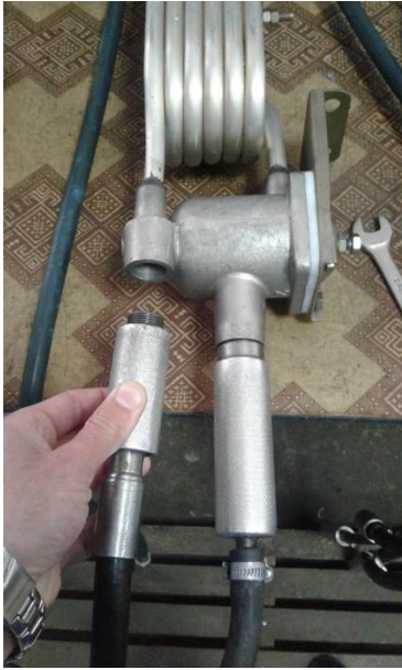
Water and oil separation system. Pressure up to 20 bar
