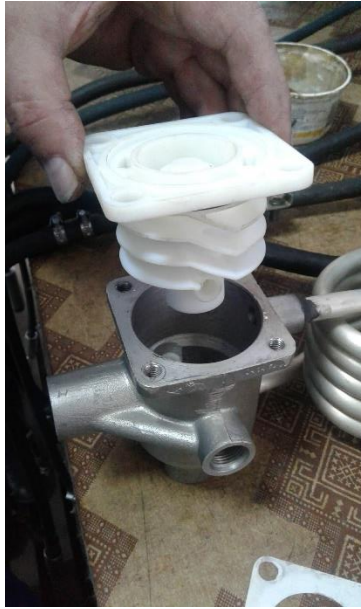
Water and oil separation system. Pressure up to 20 bar
