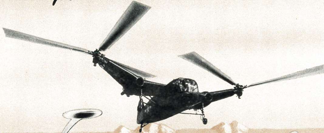
XHJD-1 UTILITY HELICOPTER World's first twin-engine helicopter.
