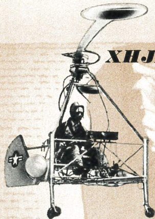
LITTLE HENRY World's first ram-jet helicopter.
