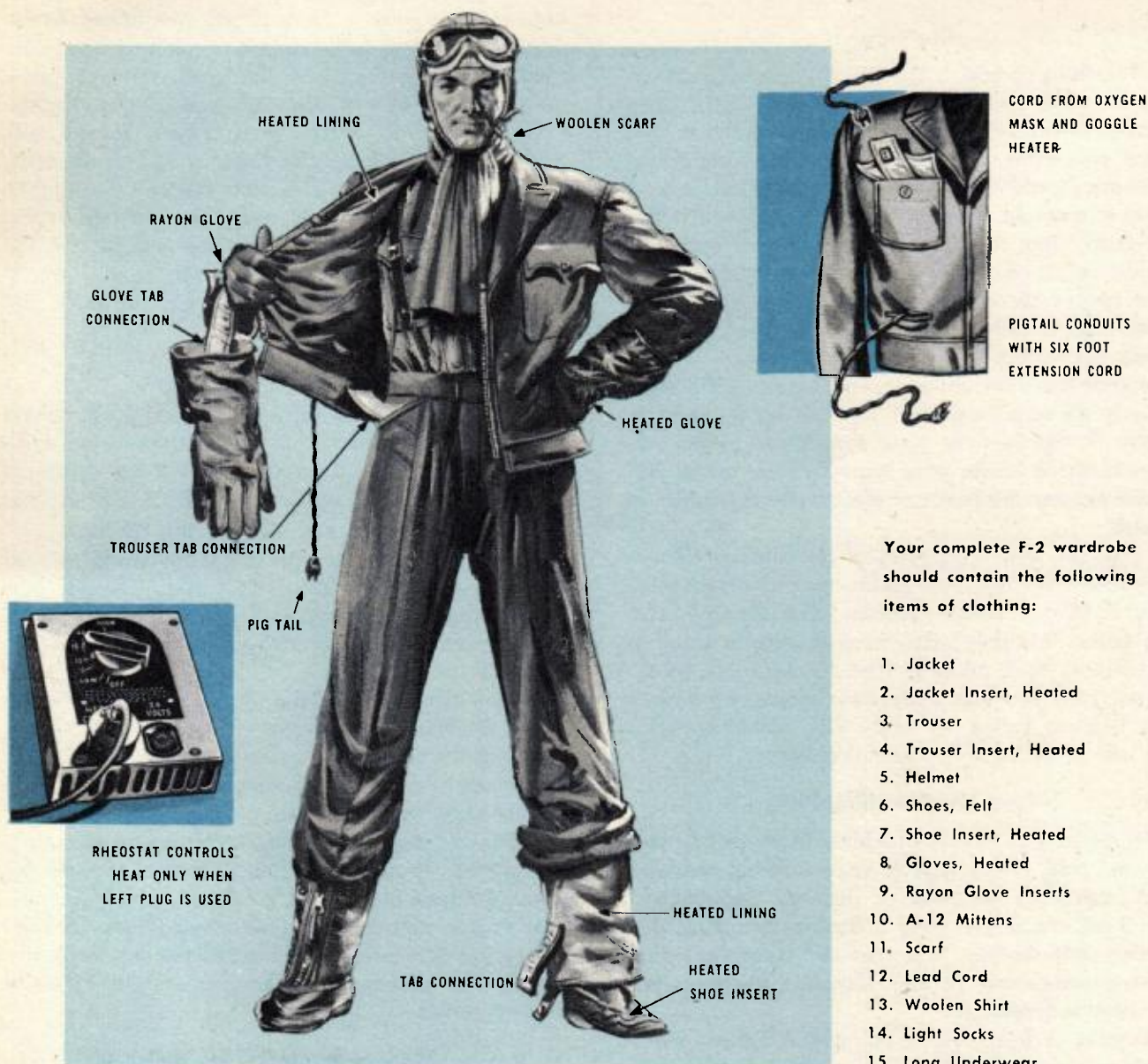
F-2 ELECTRICALLY HEATED FLYING SUIT
