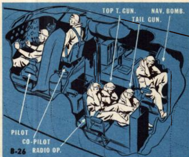
Ditching Positions in the B-26
