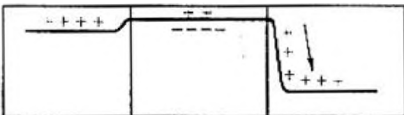
Figure 4-75. PNP Transistor with Signal Applied, making Base More Negative with Respect to Emitter
