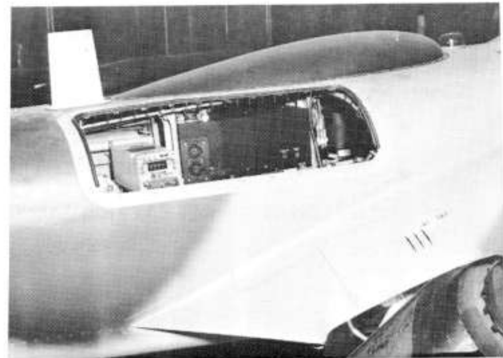
AVIONICS BAY ACCESS
