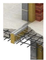
Ancon is leading the way in developing solutions to meet the Government's tough new fire safety requirements for buildings, with the launch of an upgraded range of non-combustible insulated balcony connectors.
