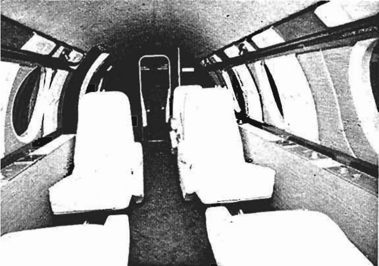
The de luxe interior of the PD-808 when fitted as an executive. Points of note are the level floor, the side shelves incorporating arm rests, ashtrays, cupholders and jotters. The sectional plastic sun screens and the lights and punkahs above are fully adjustable. At the front of the cabin are the radio rack and a bar unit. Through the door can be seen the instrument panel. This photo is of the full-scale mock-up, since the prototype is still full of instruments.
