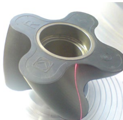
Above left, the large aperture angle and the high numerical aperture of confocal chromatic sensors enable high resolution with a small light spot size. Above right, laser scanners are used for 3D measurement of complex geometries and rotating components. For quality assurance of rotary pistons, the piston surface is measured 360^\circ and compared with the nominal shape within a narrow tolerance.
