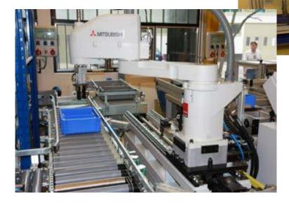
Linear axis including SCARA industrial robotsystem
