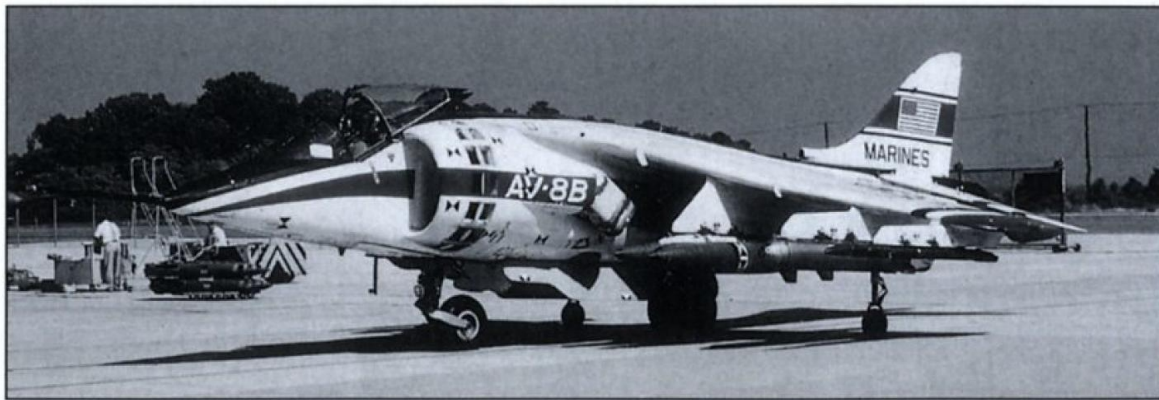
One of the two YAV-8B prototypes, clearly showing both the retention of the original cockpit position and the double set of inlet suction relief doors. (via Gary Madgwick)
