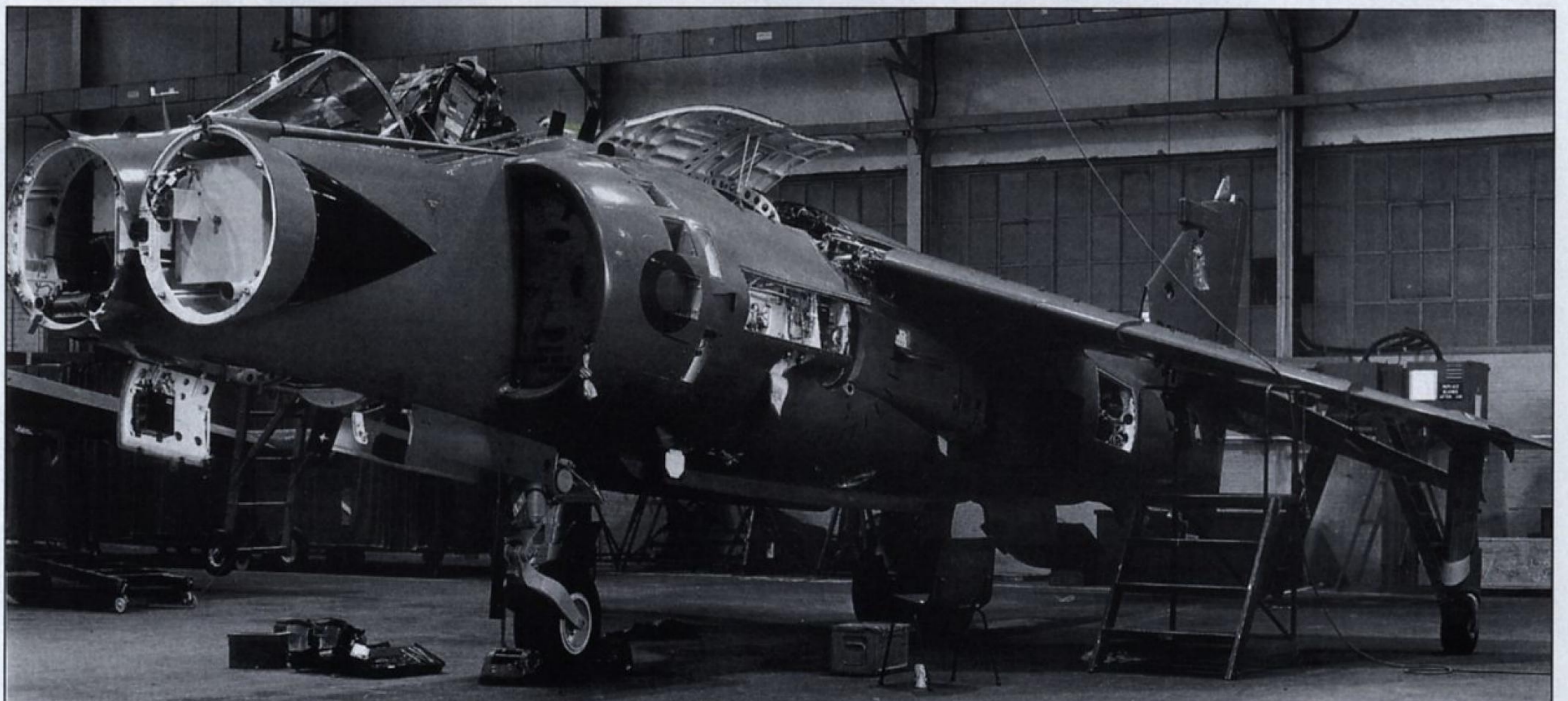
Below: This Sea Harrier FRS.1 ZD580, one of three post-Falklands attrition replacement aircraft, is seen undergoing fitting of equipment at Dunsfold prior to delivery, and reveals some very useful detail of its access panel locations and their internal features. (MoD)
