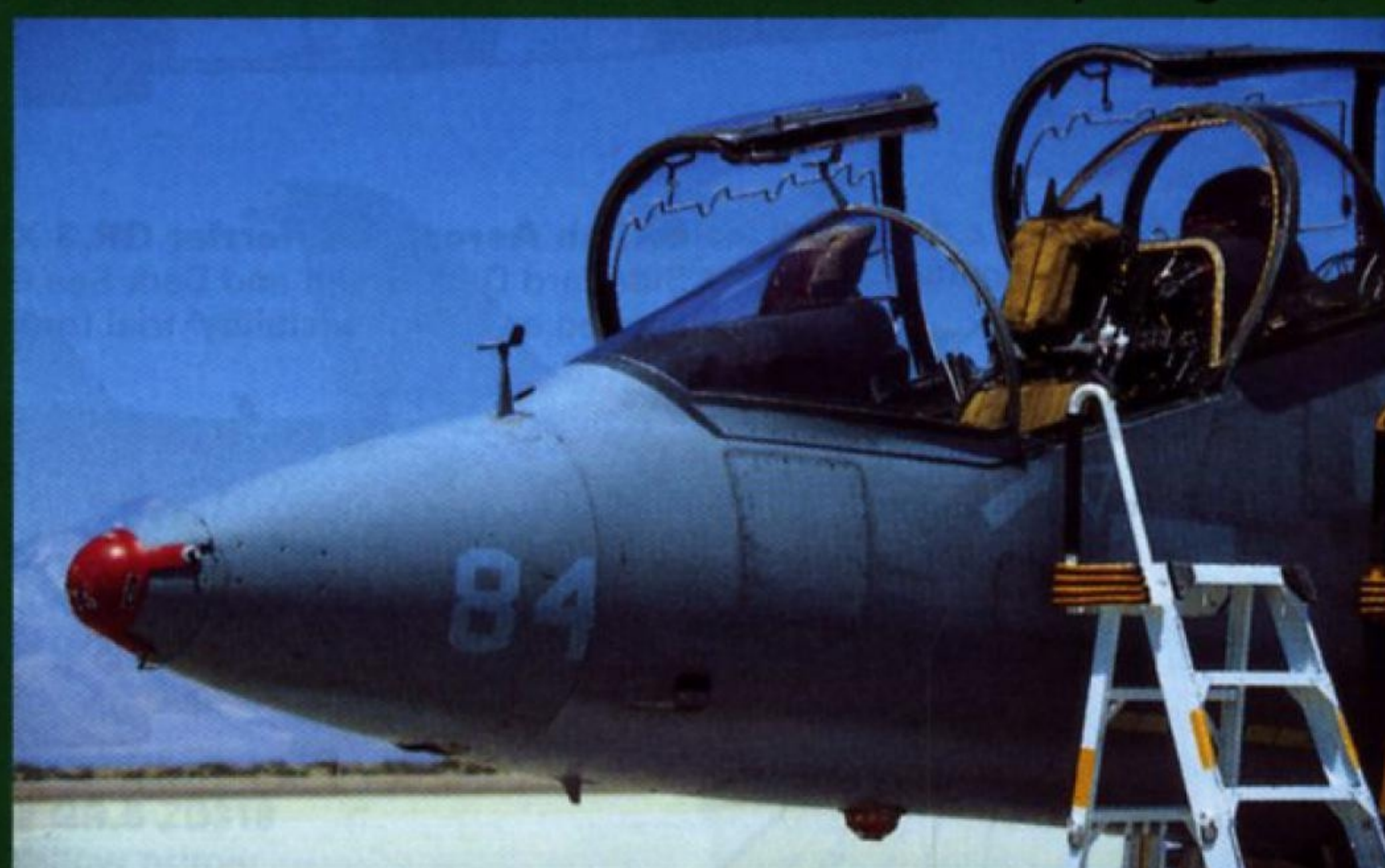
Nose of the China Lake TAV-8B, showing to good effect the side-ways-opening canopies of the two-seat aircraft. (Neville Dawson)
