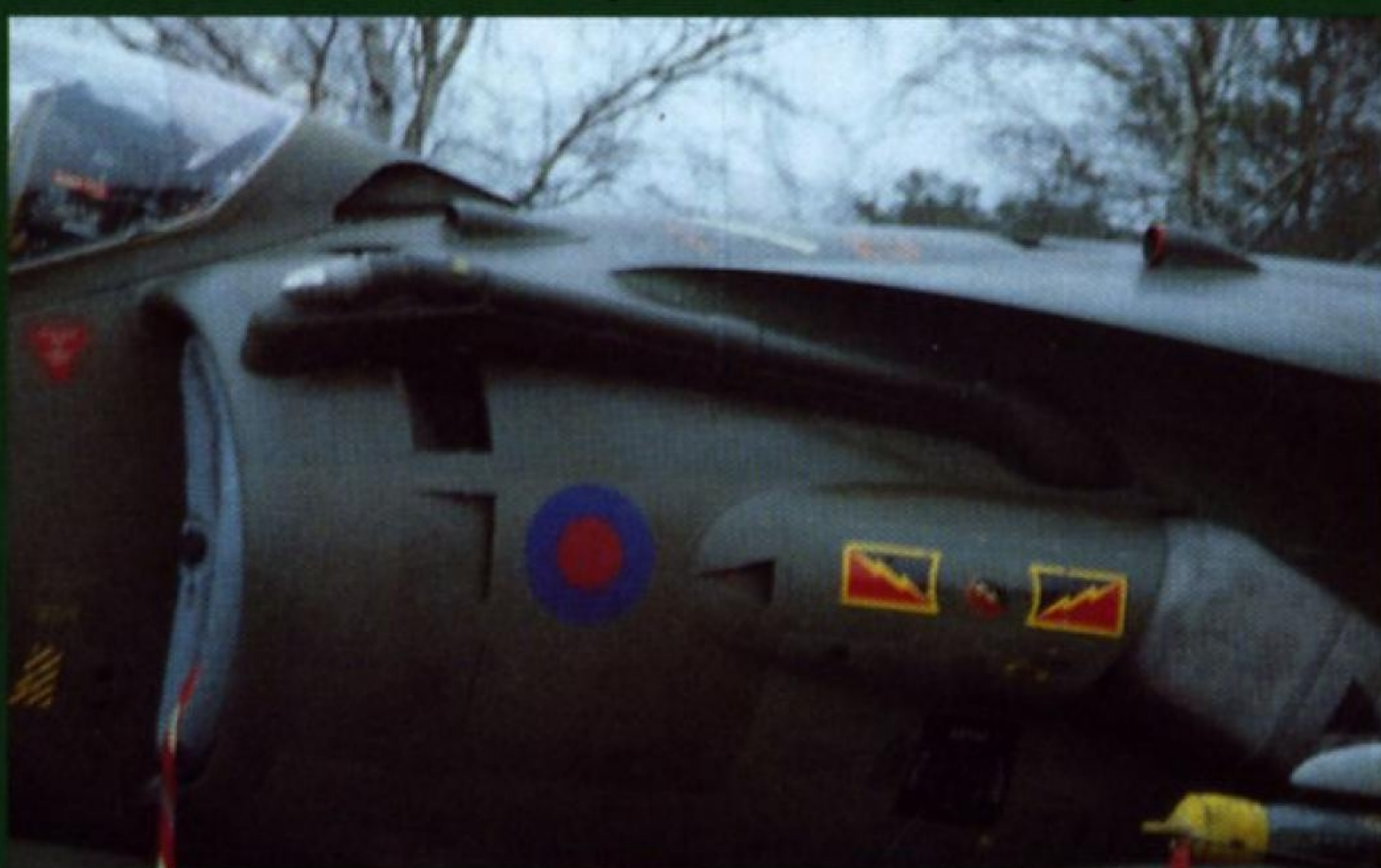
Port air intake area of a No. 4 Squadron GR.7, showing clearly the optional inflight-refuelling probe. (Gary Madgwick)
