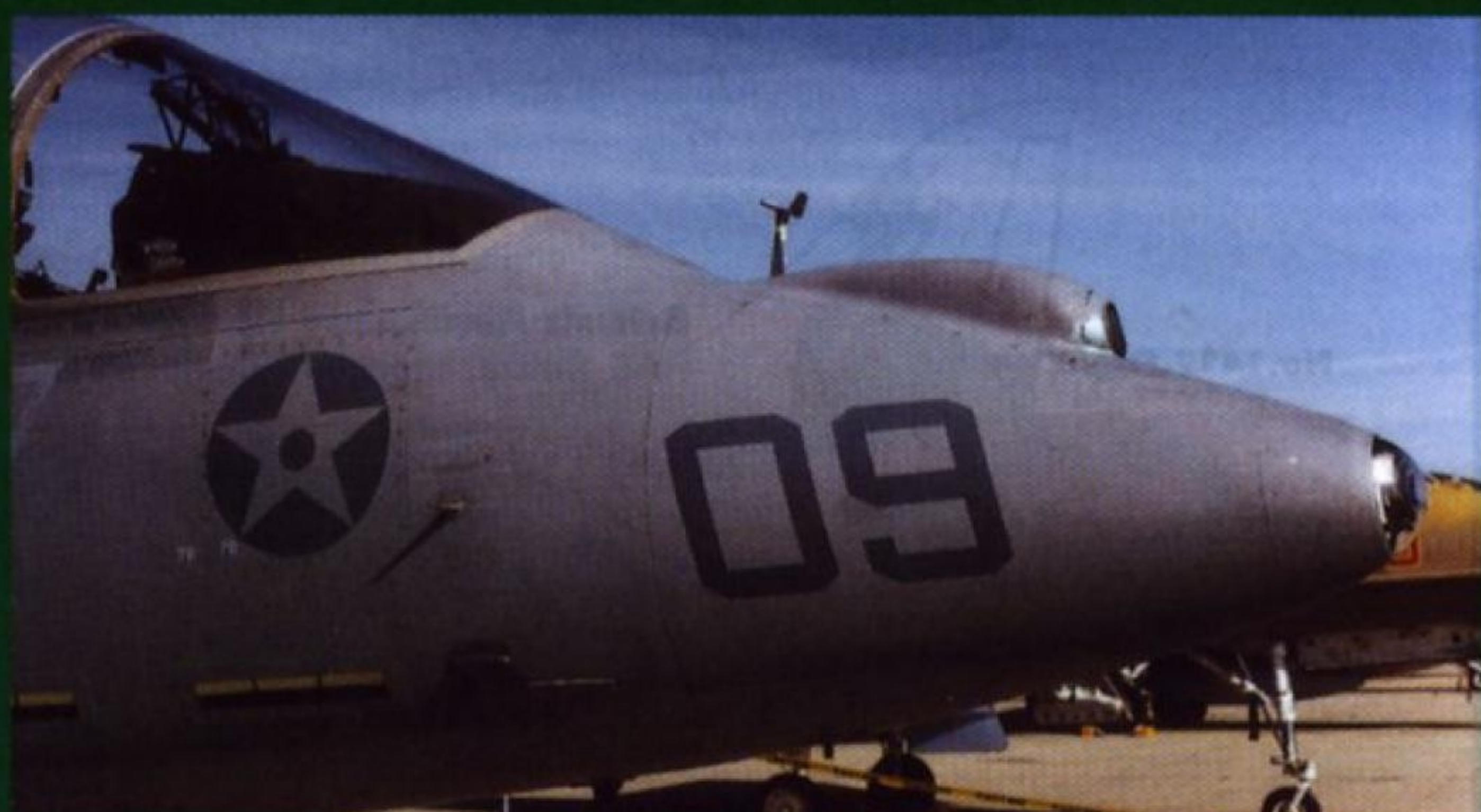
Nose area of an AV-8B, showing the ARBS seeker in the tip, and the FLIR unit fitted to the Night Attack aircraft. (Scott Van Aken)
