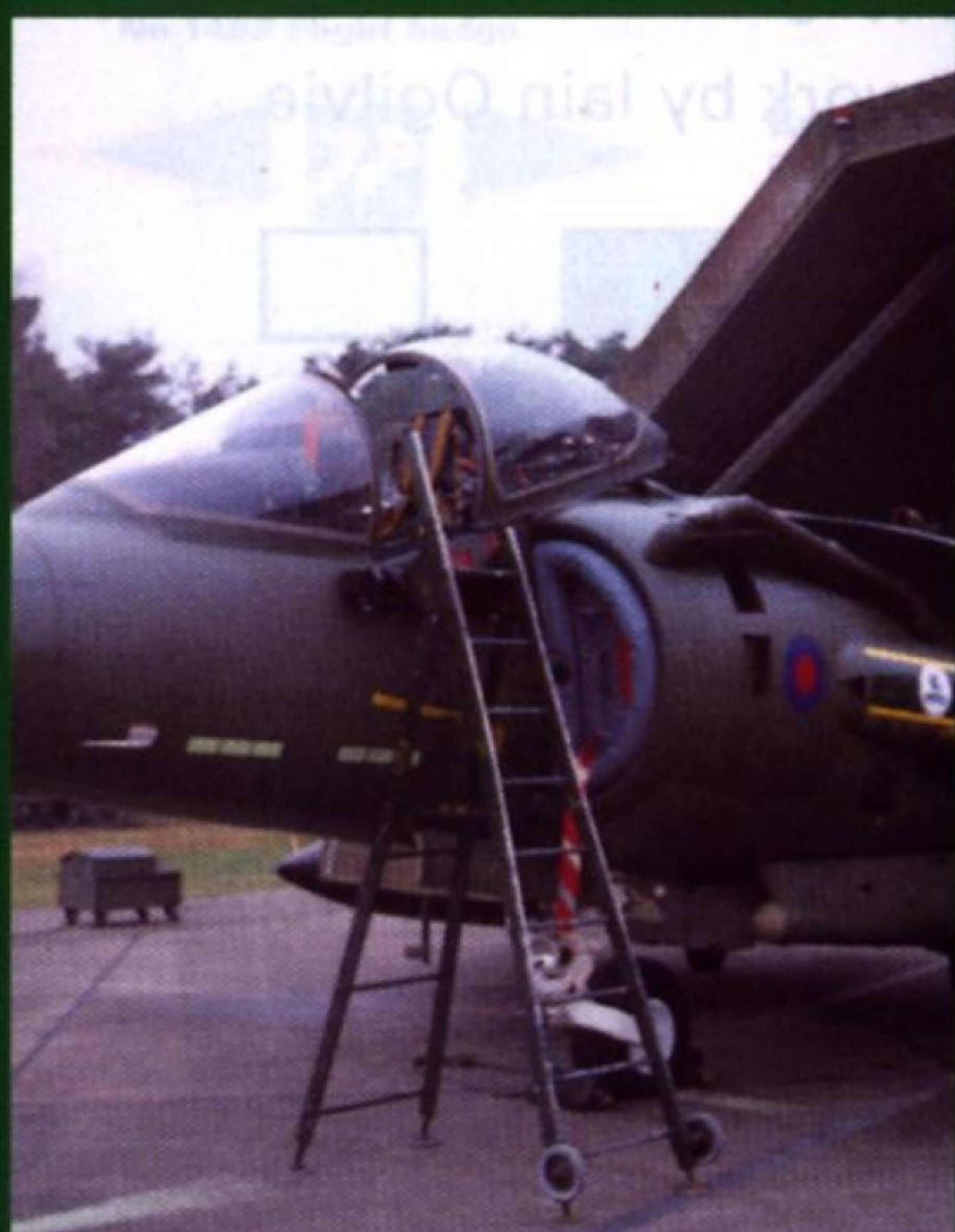
Access to the Harrier GR.7 is by way of a wheeled boarding ladder. (Gary Madgwick)
