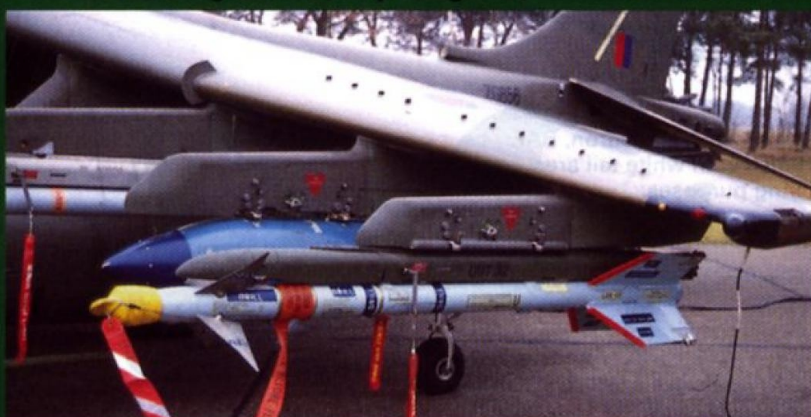
The outer wing pylons with an inert bomb and Sidewinder missile and launch rail on a No. 4 Squadron GR.7. (Gary Madgwick)
