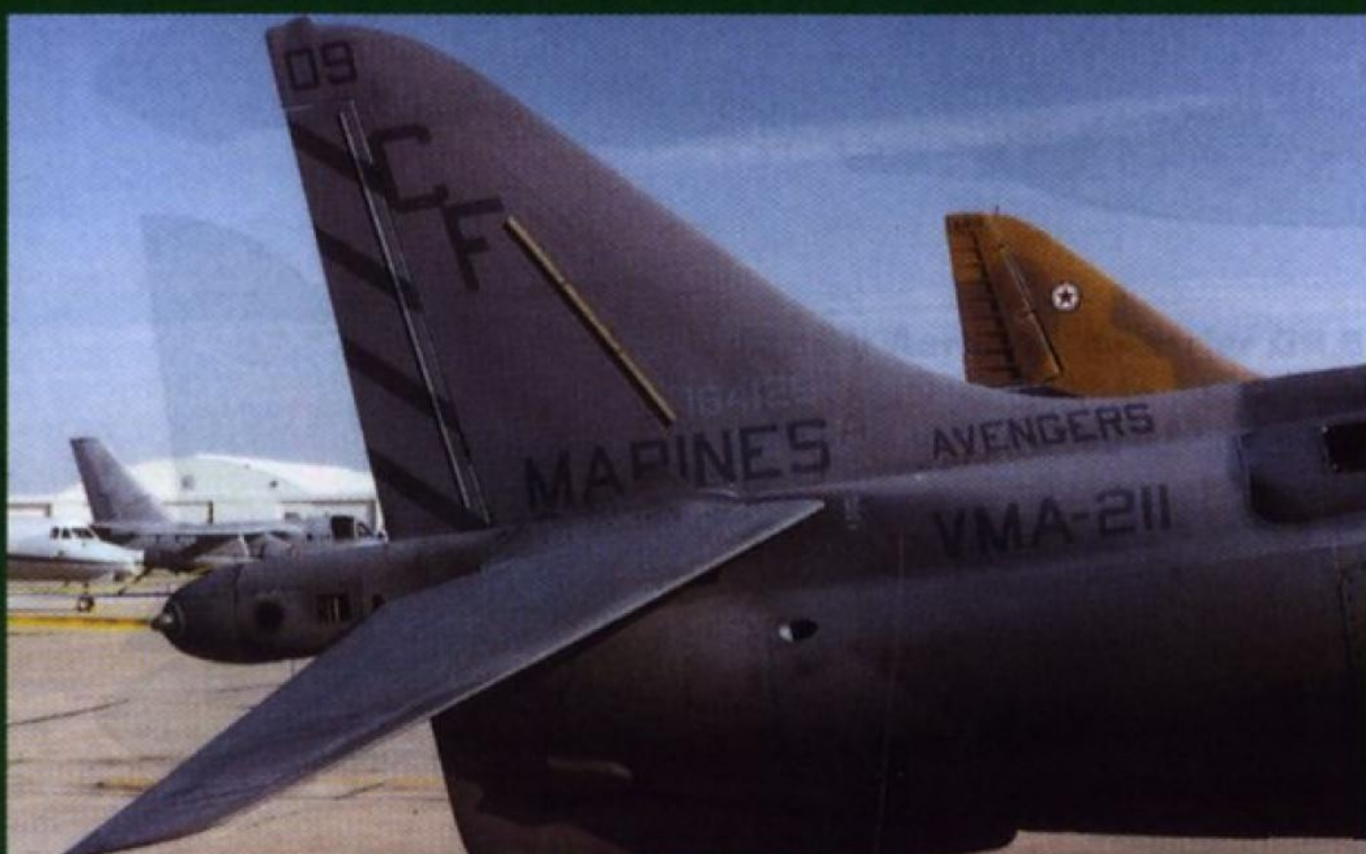
Close-up of the tail of an AV-8B Harrier II. Visible at the extreme right is part of the starboard chaff dispenser. (Scott Van Aken)
