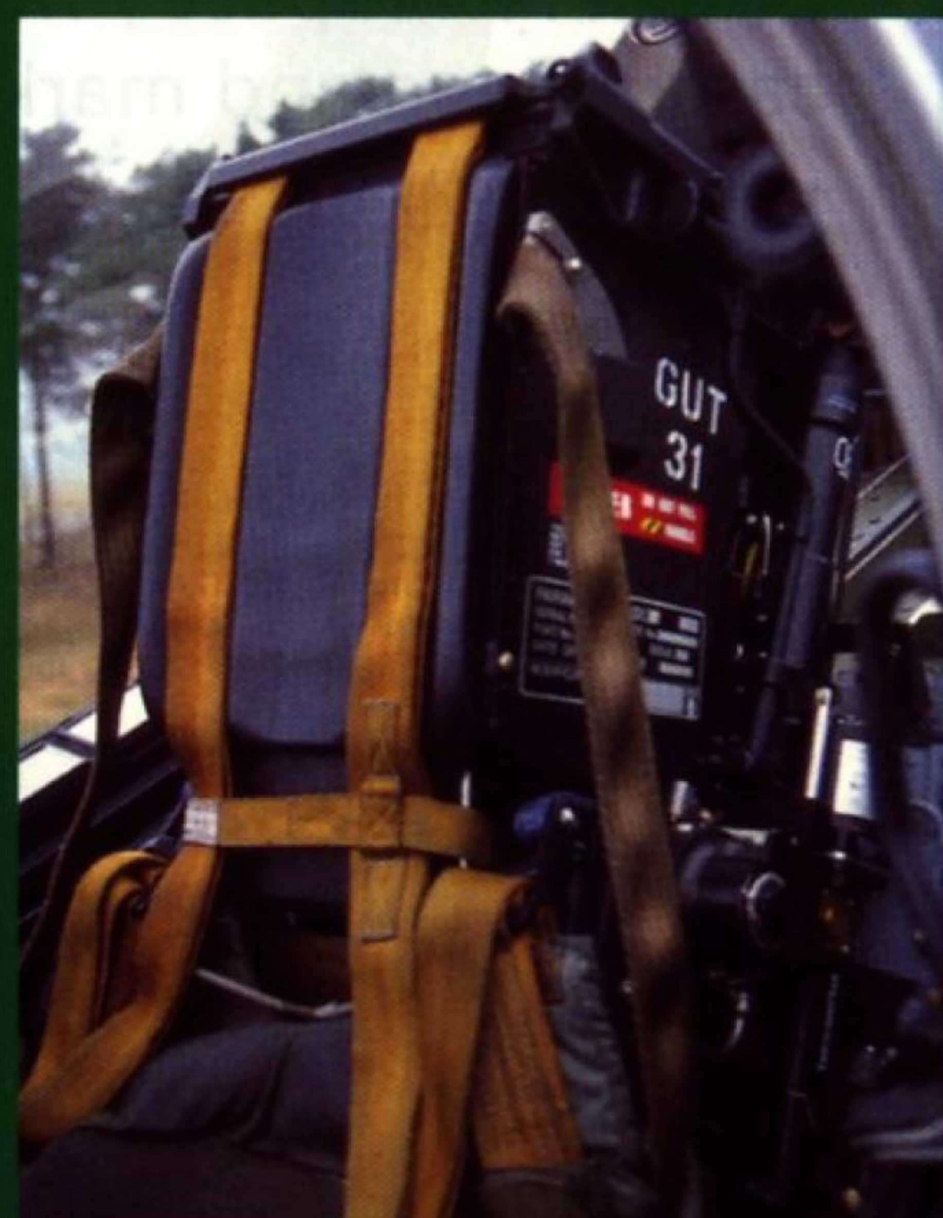
Detail of the Martin-Baker Mk. 12 ejection seat in British aircraft. (Gary Madgwick)
