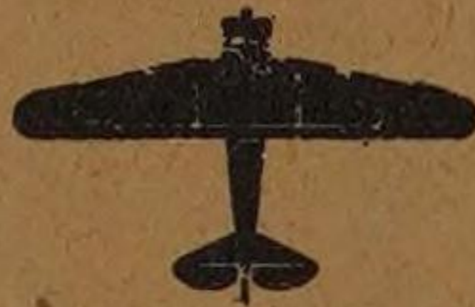
Taper on leading edge only: "Harvard"
