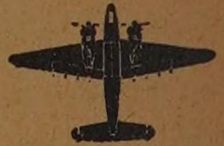
Full taper on both edges: "Hudson"
