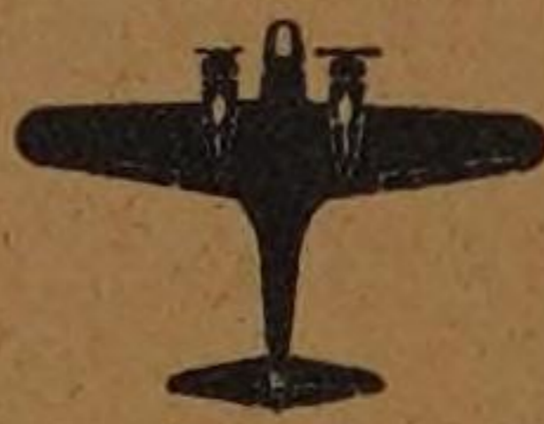
Moderate taper, about equal on both edges: "Anson"
