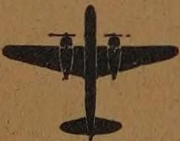
Taper on trailing edge only: "Boston"
