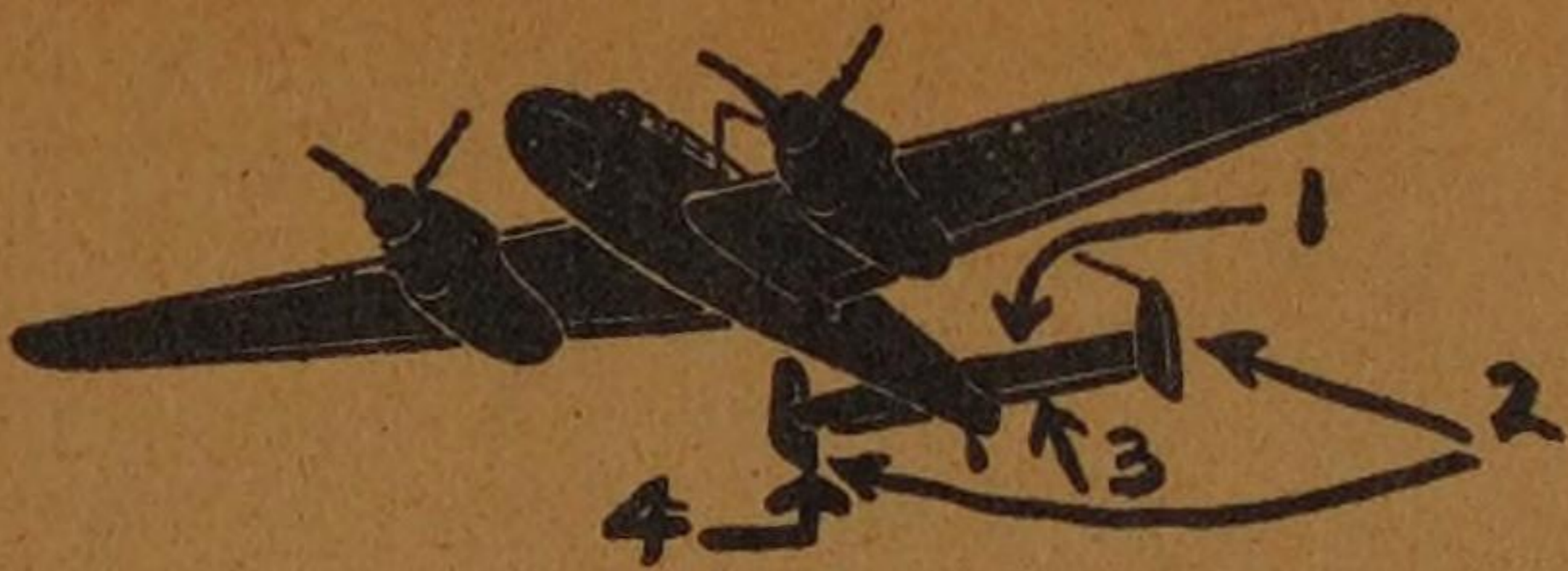
Compound Tail Unit: (1) Tailplane, (2) twin fins and rudders, (3) elevator, (4) rudder
