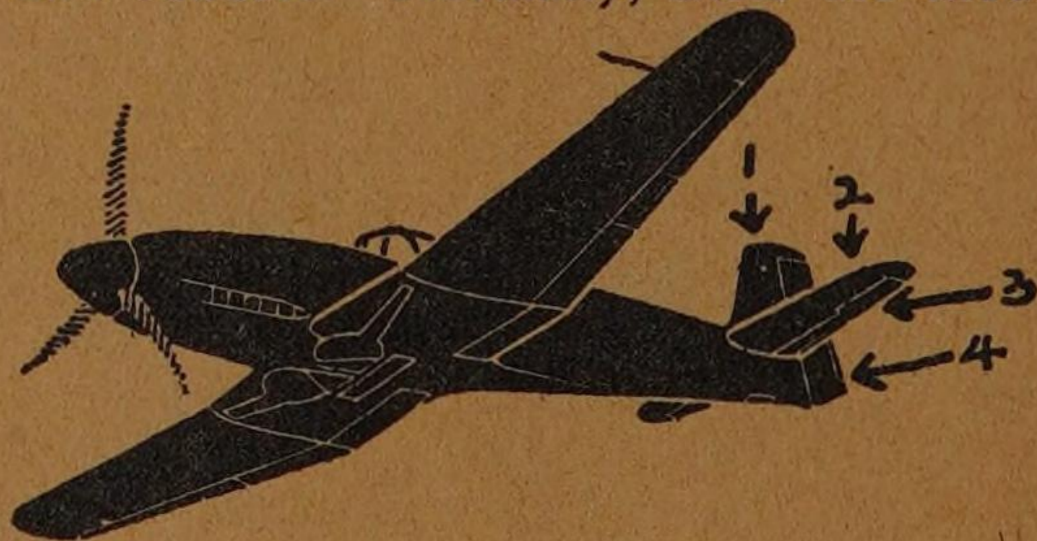
Simple Tail Unit: (1) Single fin, (2) tailplane (3) elevator (4) rudder
