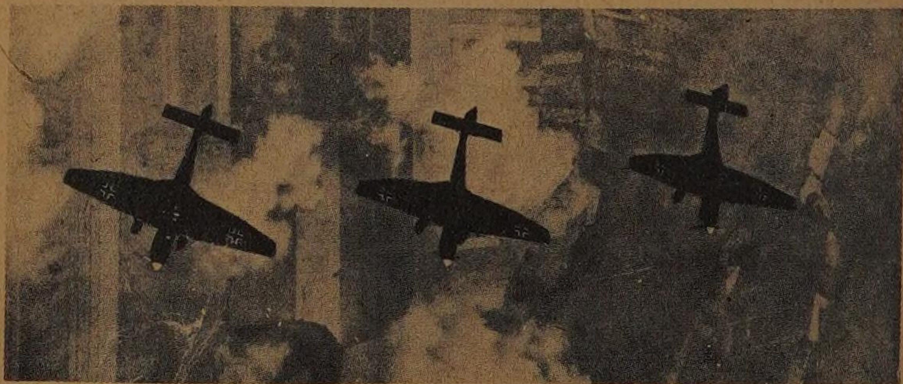
The Junkers 87 Dive Bomber. The rectangular tailplane has no cut-away.
