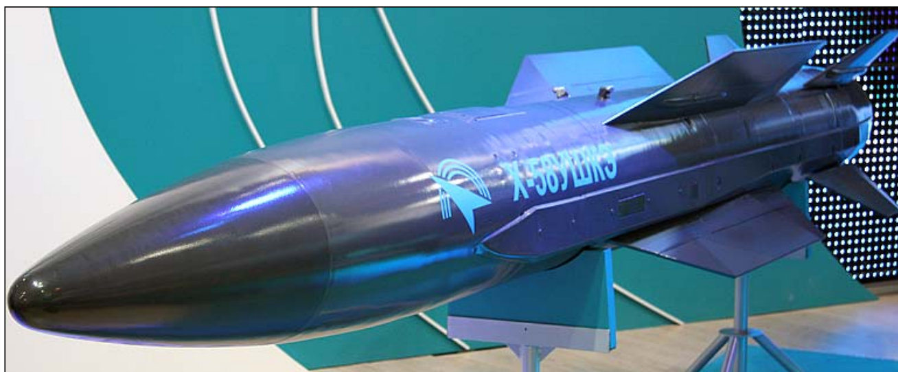
KTRV Kh-58UShKE Kilter anti-radiation missile. Note the significantly revised radome and cruciform reduced span folding wing design of this recent variant (© 2009 Vitaliy V. Kuzmin).
