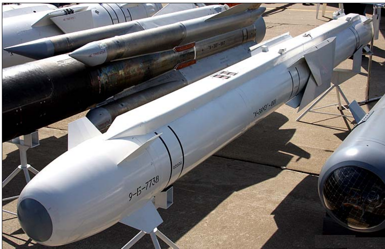
Kh-38 mockup on display. Note the folding fins for internal carriage ( © 2009 Vitaliy V. Kuzmin).
